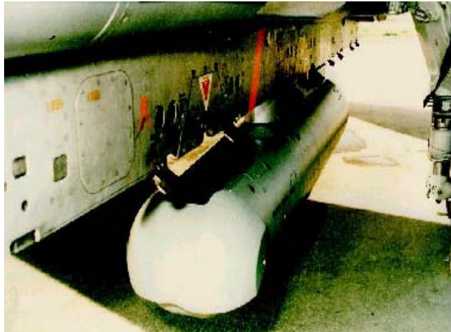
Figure 6-4: TORNADO-IDS CLDP Installation.
