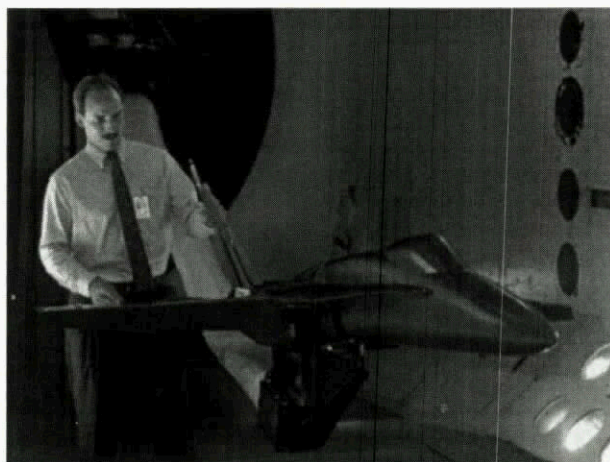
Figure 2. The 1/6-Scale F/A-18 model in the Transonic Dynamics Tunnel at the NASA Langley Research Center
