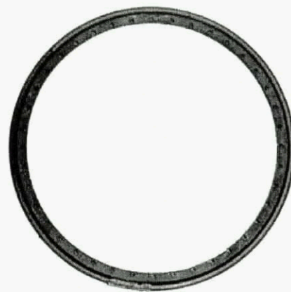
Figure 2. A compressor spacer of the type used in this study.
