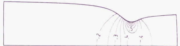
Fig.7 Inverse calculation Mach contours for the axisymmetric convergent-divergence nozzle case
