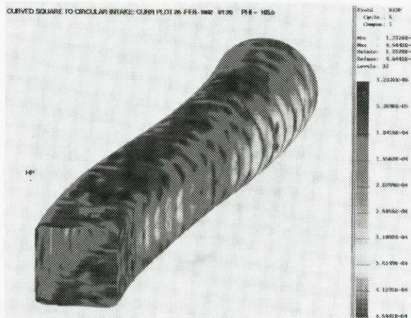
Fig. 24 Radar signature prediction for air intakes positioning and design
