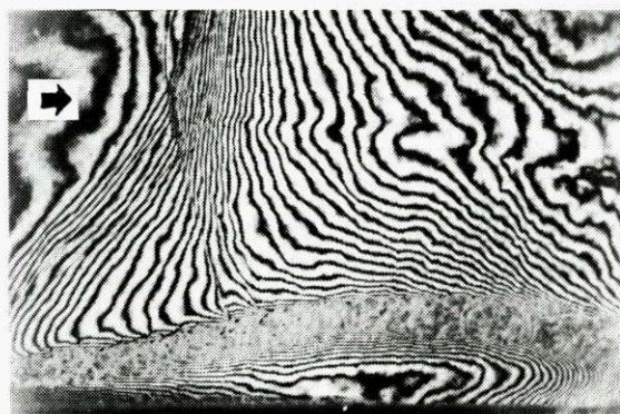
Fig. 35 - Conical Holographic Interferogram of Mach 2.43, \alpha = 15^\circ Interaction.
