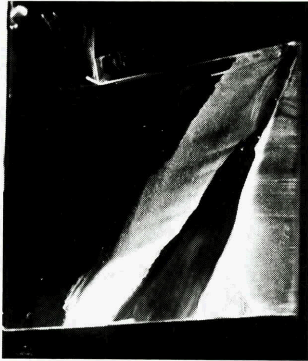
Fig. 16: Surface flow visualization, M = 2 , evidence of secondary separation
