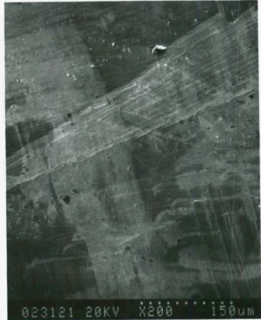
Figure 3(a). Solidifying surface of CPTi showing the planar/cellular growth. (SEM image).
