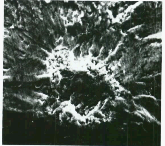
Crack initiation at an inclusion
