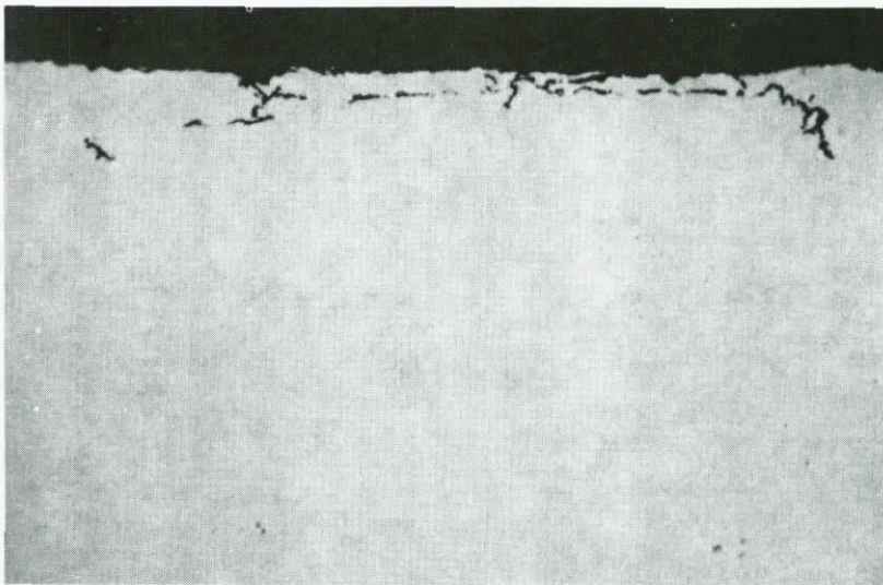
FIGURE 7: Shallow surface dross film. Mag 200X
