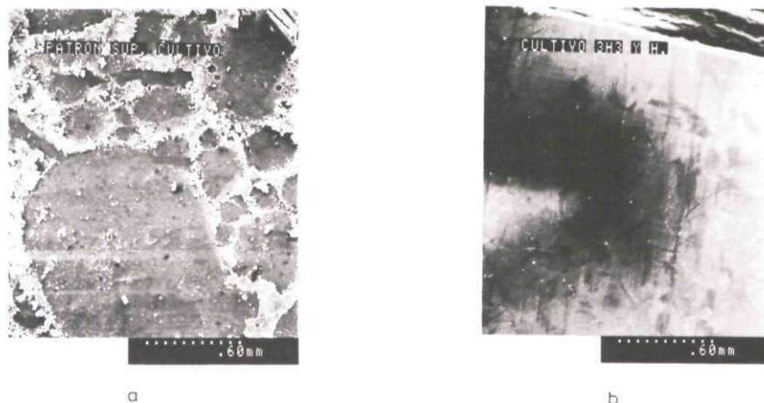
Figure-4 SEM photograph of the surface of an Hercules AS-4/8552 specimen (a) exposed to a culture of microorganisms in JP8/water and (b) after having been wiped with acetone.
