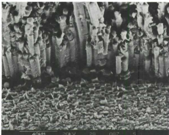
Figure 9. Fibre-matrix interfaces in tension area and fibre tips in compression area (APC2-FC(330)).
