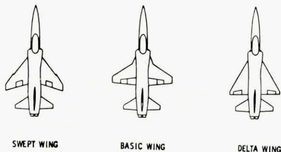
Fig. 5. Wing models tested with model based on F-5 configuration (Ref. 8)
