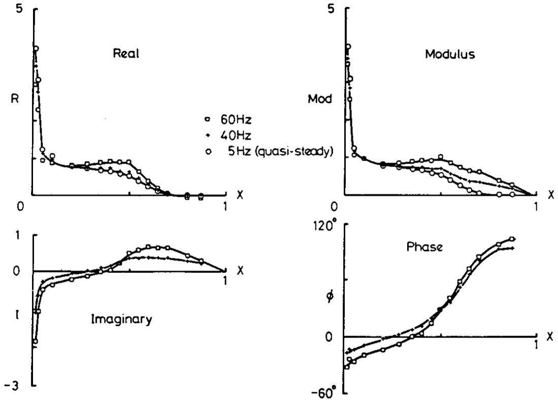
Fig 7.10 Oscillatory pressures,  $M = 0.90$ ,
