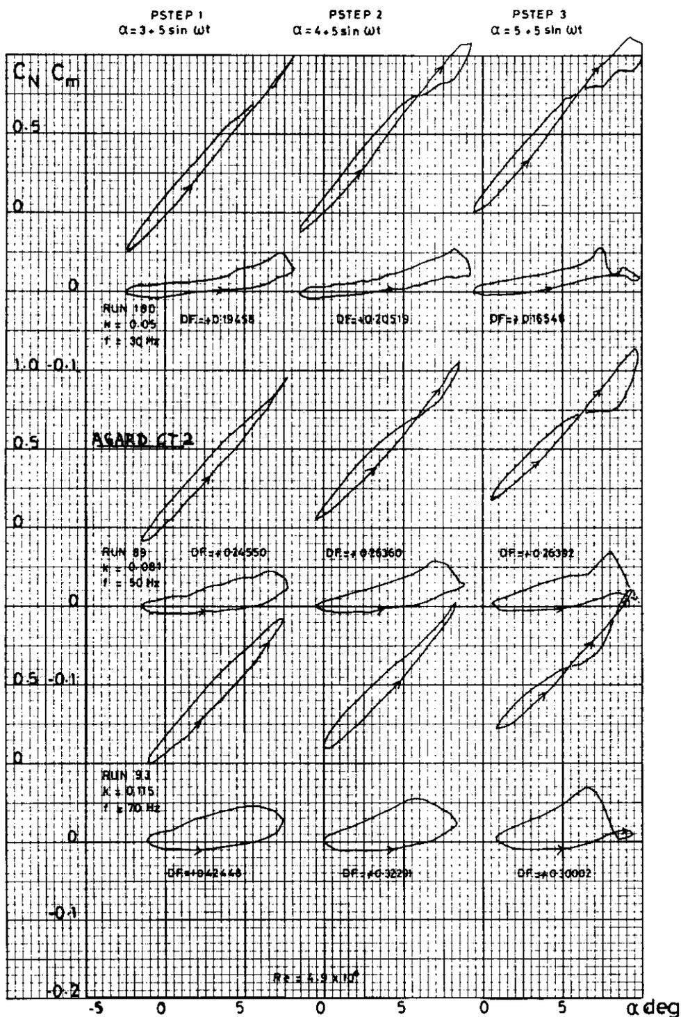
Fig 3.3  $C_N, C_m$  v. incidence over range of  $\alpha_m = 3^\circ, 4^\circ, 5^\circ$ ;  $\alpha_0 = 5^\circ$ .
