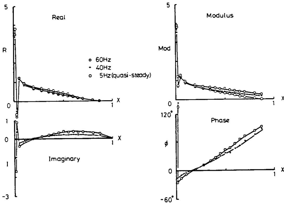
Fig 7.9 Oscillatory pressures,  $M = 0.80$ ,  $\alpha_m = 0$ . Influence of frequency, Section 2E
