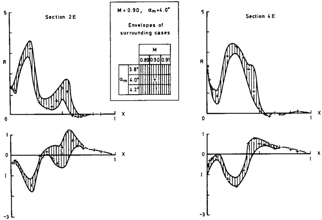
Fig 7.18 Oscillatory pressures for a matrix of cases centred on  $M = 0.90$ ,  $\alpha_m = 4.0^\circ$ ,  $f = 40$  Hz
