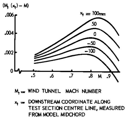
Fig. 4.11 Mach number distribution in NLR Pilot Tunnel test section
