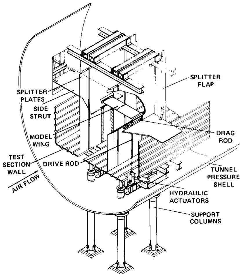
Fig. 2.1. General arrangement of oscillating airfoil test apparatus in NASA Ames 11- by 11-Foot Transonic Wind Tunnel.
