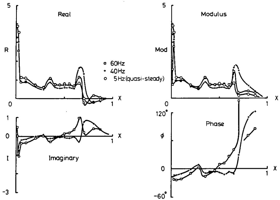
Fig 7.11 Oscillatory pressures,  $M = 0.95$ ,
