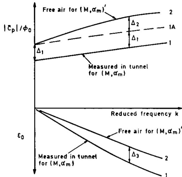
It is assumed that a steady condition  $(M, \alpha_m)$  in the tunnel is equivalent to a steady condition  $(M, \alpha_m)'$  in free air.
