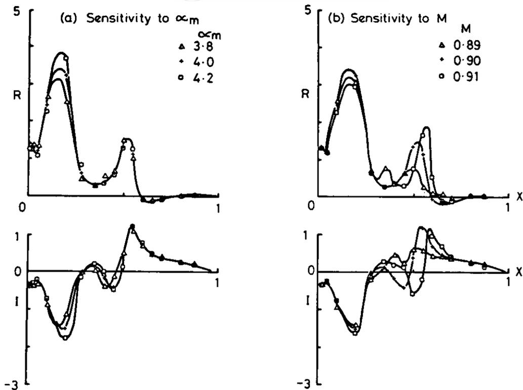
Fig 7.16 Oscillatory pressures. Sensitivity to small changes of incidence and Mach number.  $M \approx 0.90$ ,  $\alpha_m \approx 4^\circ$ . Section 2E,  $f = 40$  Hz
