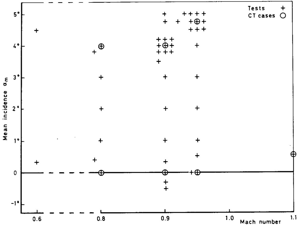
Fig 7.2 Test conditions and computational test cases
