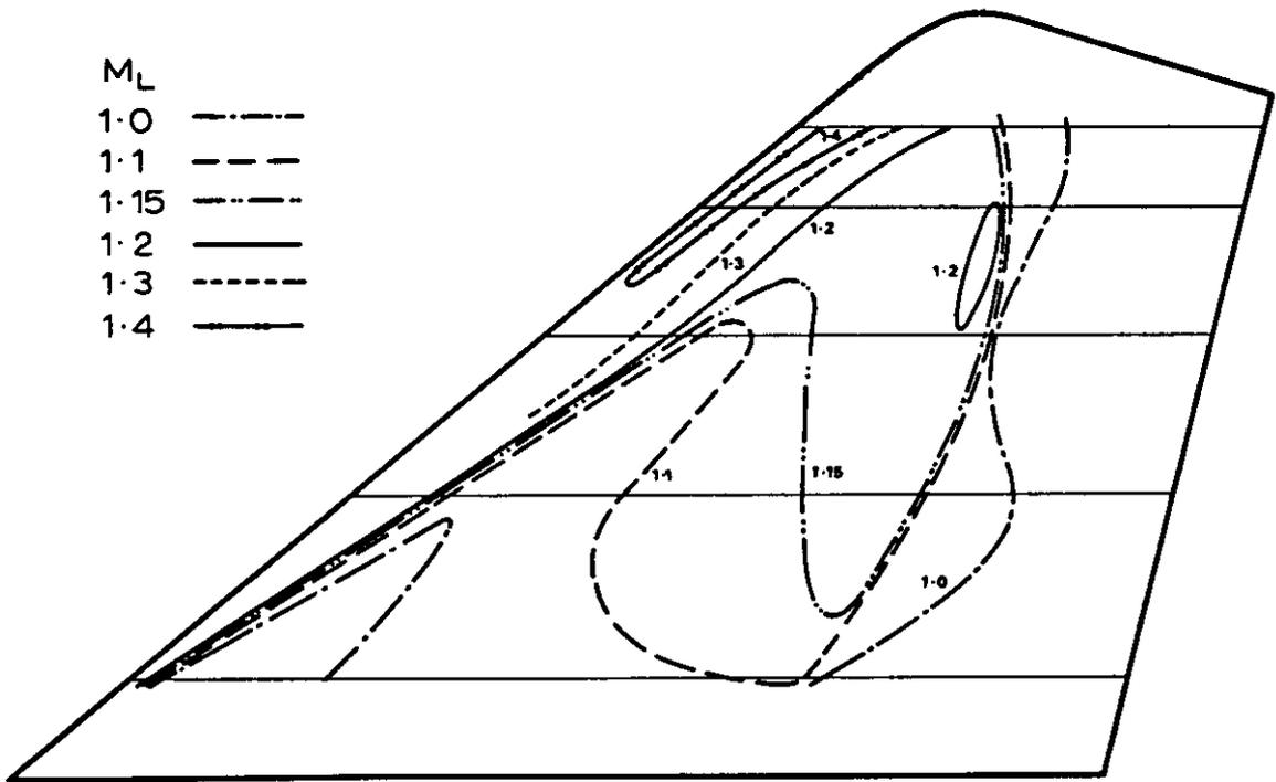
Fig 7.7 Isomachs,  $M = 0.95$ ,  $\alpha = 4^\circ$
