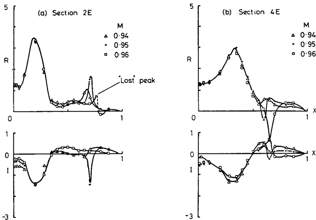
Fig 7.17 Oscillatory pressures. Sensitivity to small changes of Mach number.  $M \approx 0.95$ ,  $\alpha_m = 4.75^\circ$ ,  $f = 40$  Hz
