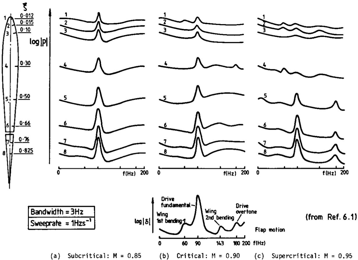
Fig 6.6 Typical spectra:  $\alpha = 0, \eta = 0.60$
