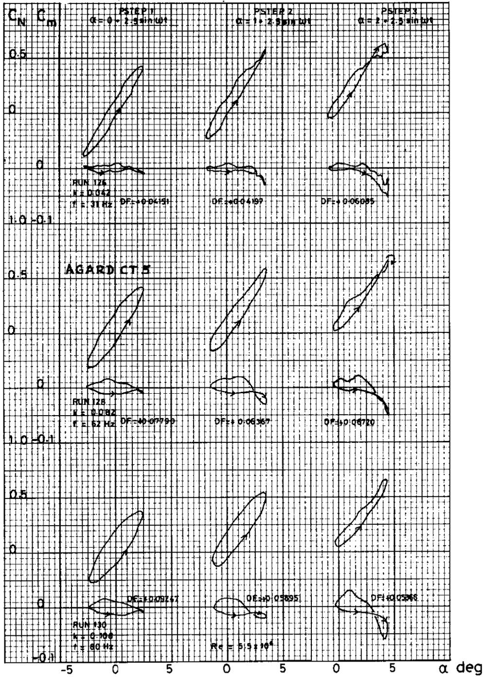
Fig 3.4  $C_N, C_m$  v. incidence over range of  $\alpha_m = 0^0, 1^0, 2^0$ ;  $\alpha_0 = 2.5^0$ .
