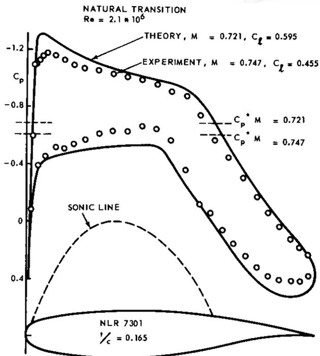
Fig. 4.9 Theoretical and experimental "shock-free" pressure distributions of the NLR 7301 airfoil (free transition)
