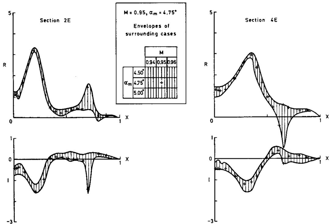
Fig 7.19 Oscillatory pressures for a matrix of cases centred on  $M = 0.95$ ,  $\alpha_m = 4.75^\circ$ ,  $f = 40$  Hz
