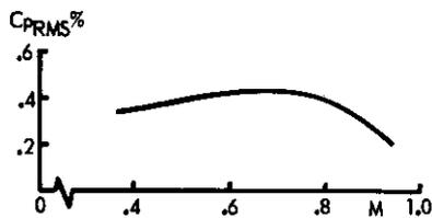
Fig. 1.6 Noise level in NLR Pilot Tunnel test section
