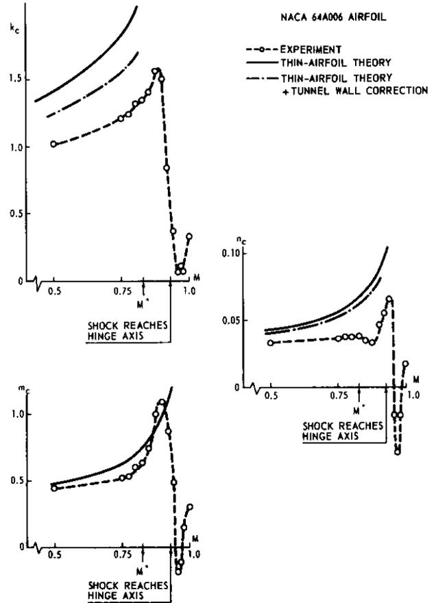
Fig. 1.3 Steady aerodynamic derivatives as a function of Mach number
