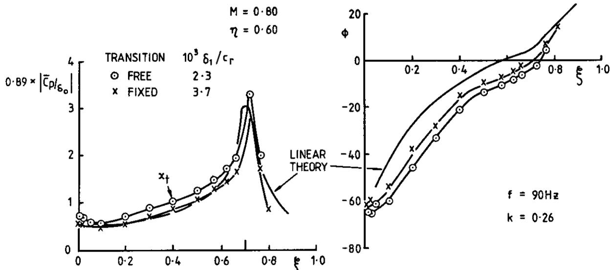
Fig 6.4 Magnitude and phase of subsonic pressure distribution
