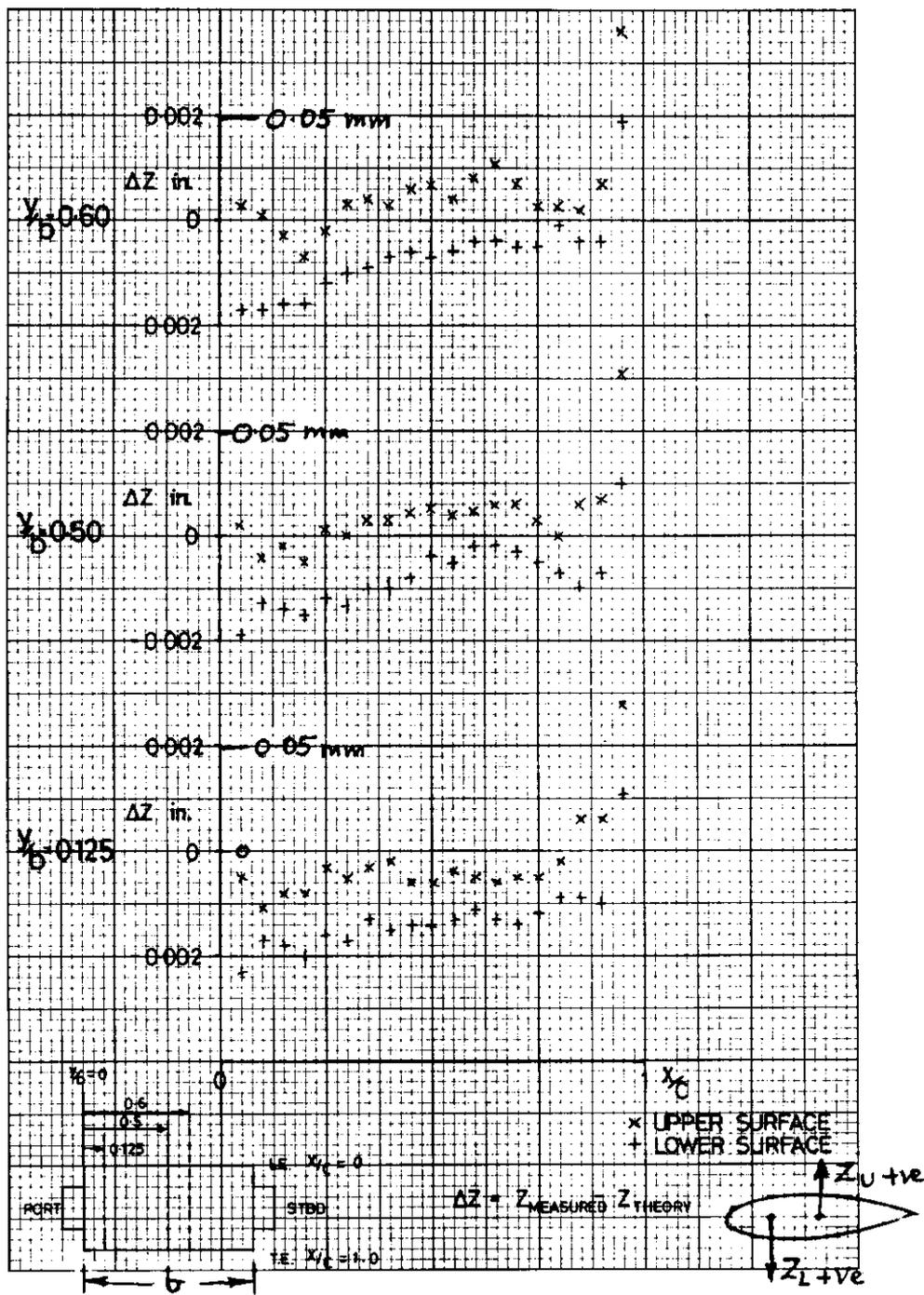
Fig 3.1 Profile inspection of NACA 0012 wing:  $Z_m - Z_t$
