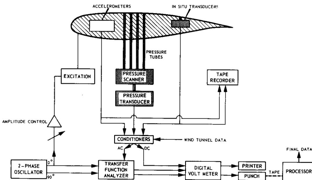
Fig. 1.9 Block diagram of measuring equipment
