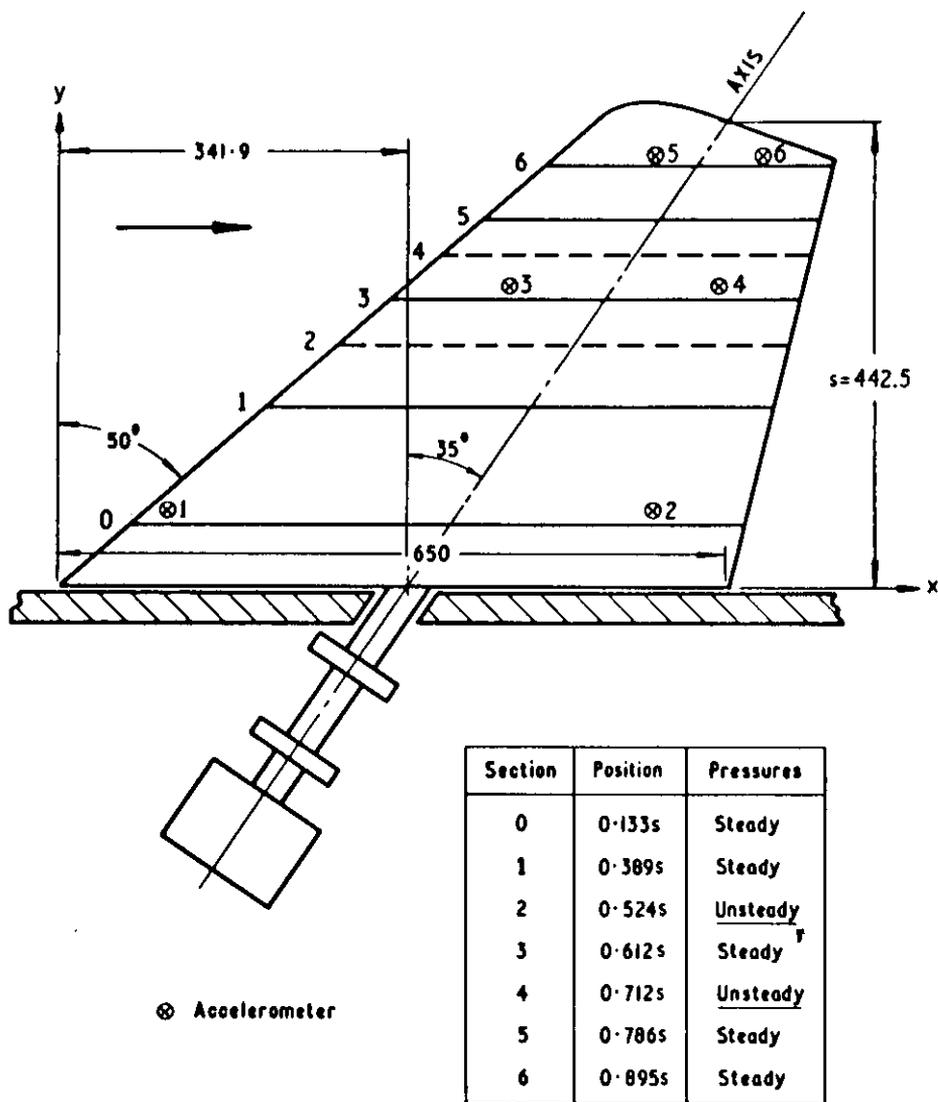
Fig 7.1 Model and rotary oscillator
