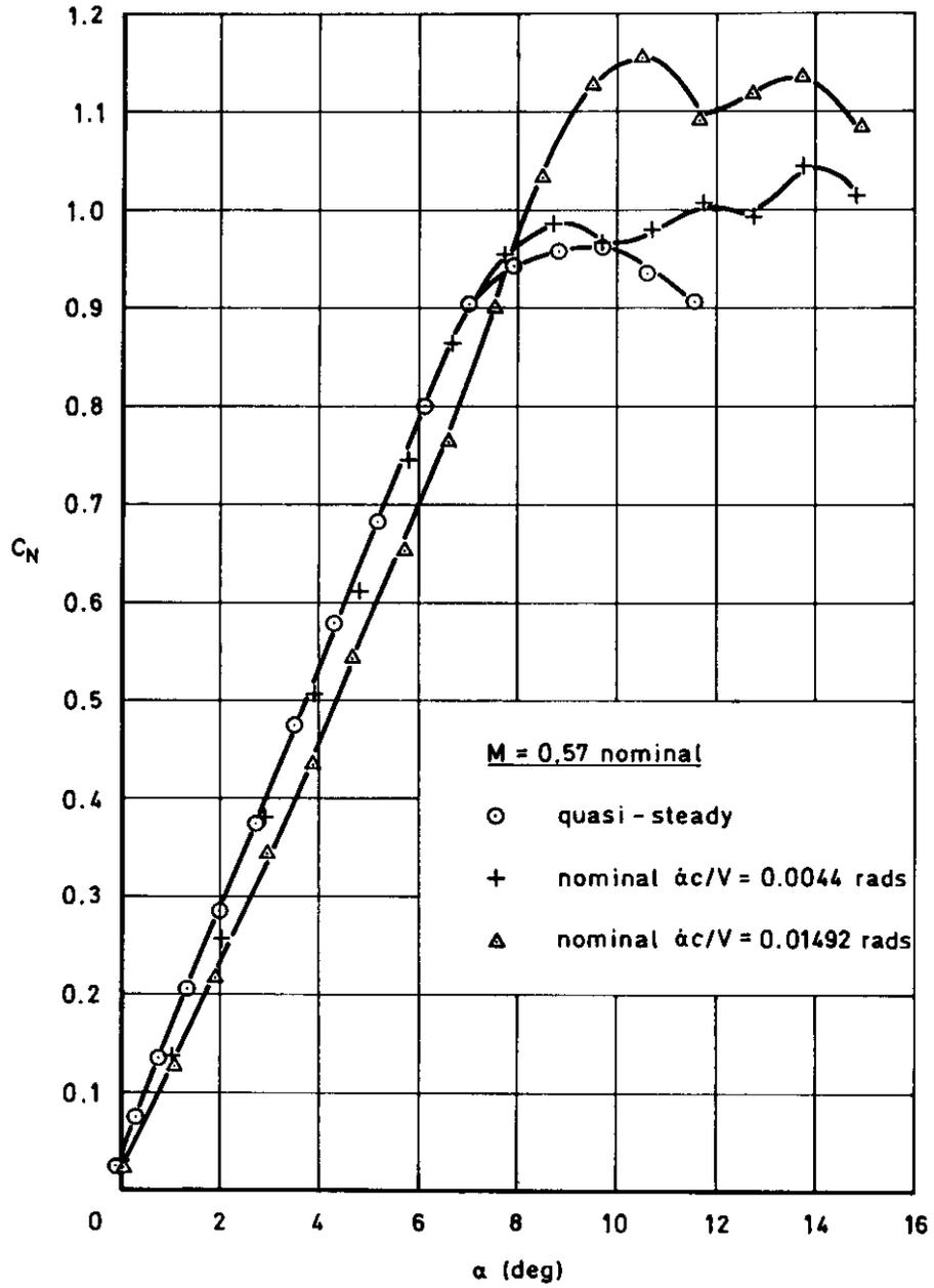
Fig 3.5 Lift  $v.$  incidence for different rates of change
