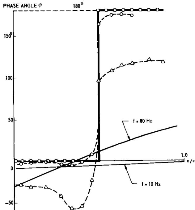
Fig. 4.1 Effect of shock wave on the unsteady pressure distributions; pitching oscillation
