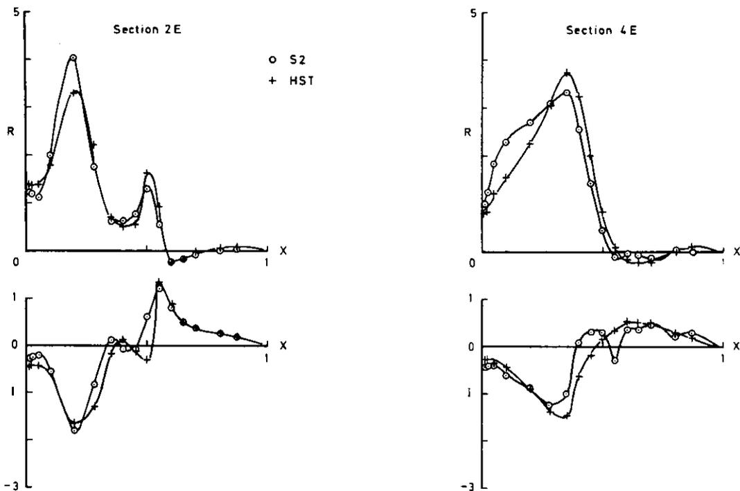
Fig 7.20 Oscillatory pressures. Comparison of data from S2 and HST.
