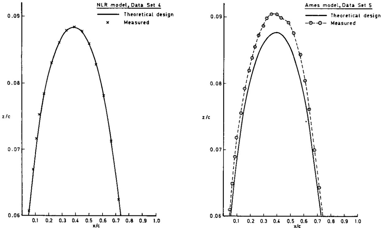
Fig 0.3 NLR 7301 Airfoil. Comparison between physical models and design shape. Profile height  $z/c$  for part of upper surface. (Note: the base line used to define  $z$  is not the same for both models; this is irrelevant to the comparisons)
