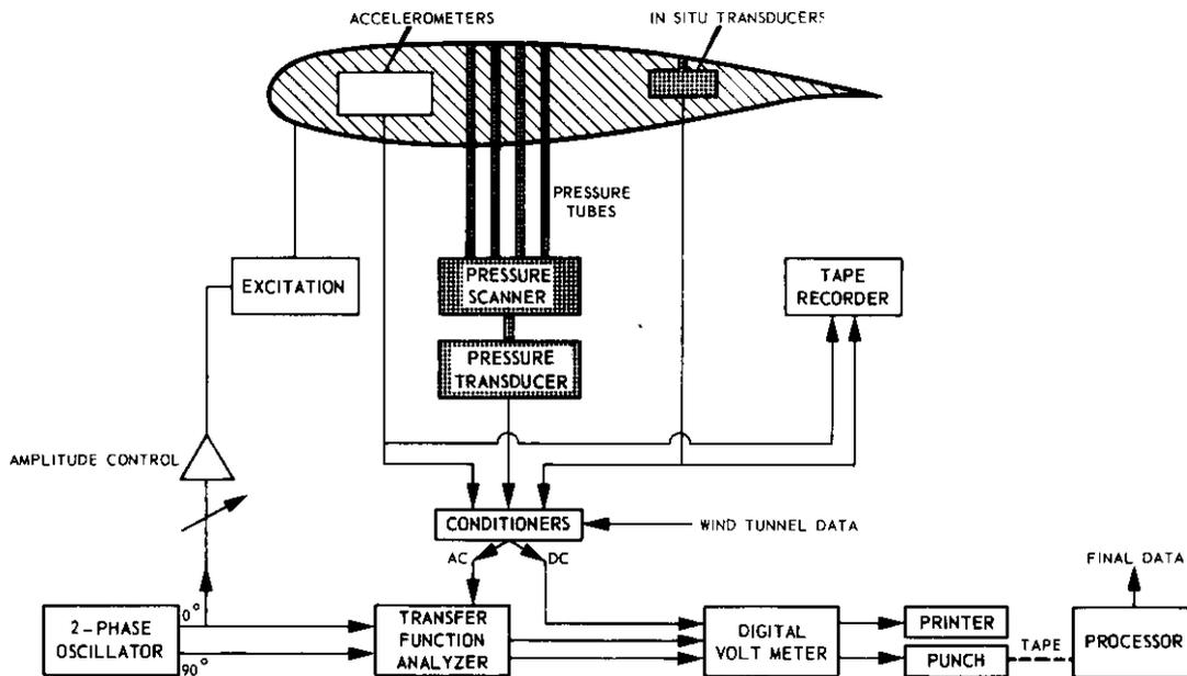
Fig. 4.17 Block diagram of measuring equipment (Conf. A). Similar equipment essentially for Conf. B
