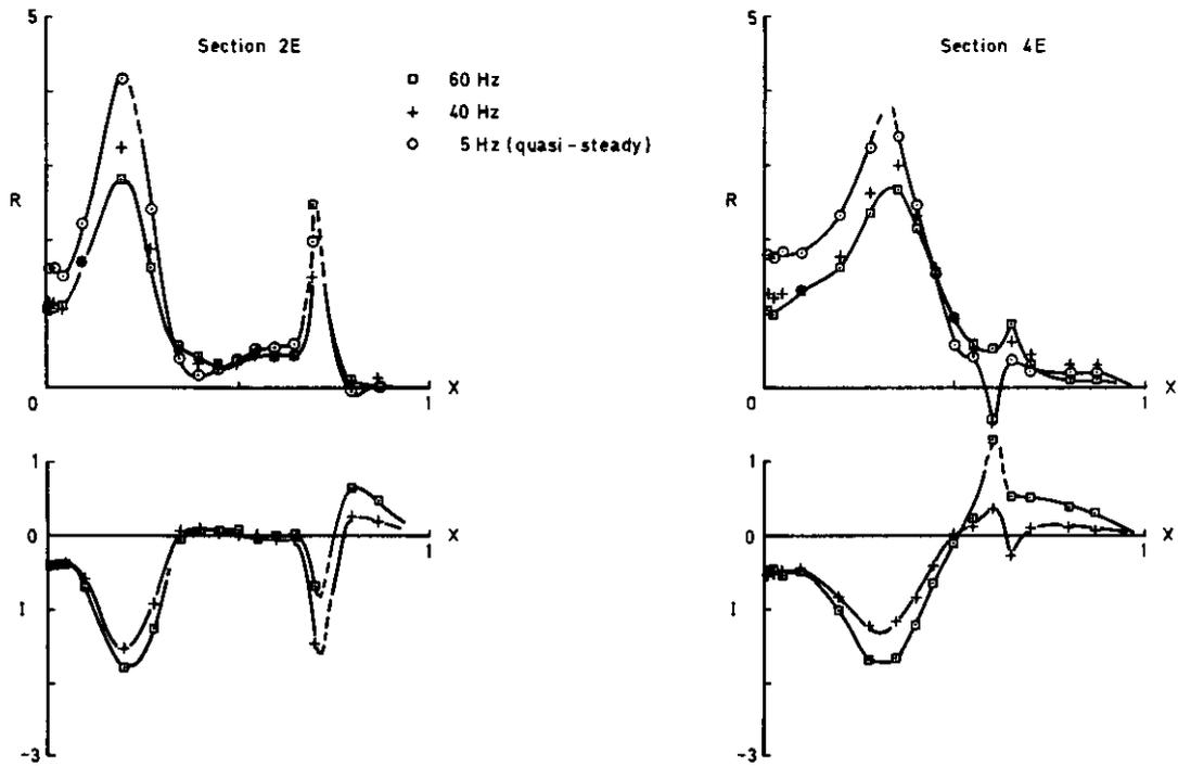
Fig 7.15 Oscillatory pressures,  $M = 0.95$ ,  $\alpha_m = 4.75^\circ$ . Influence of frequency
