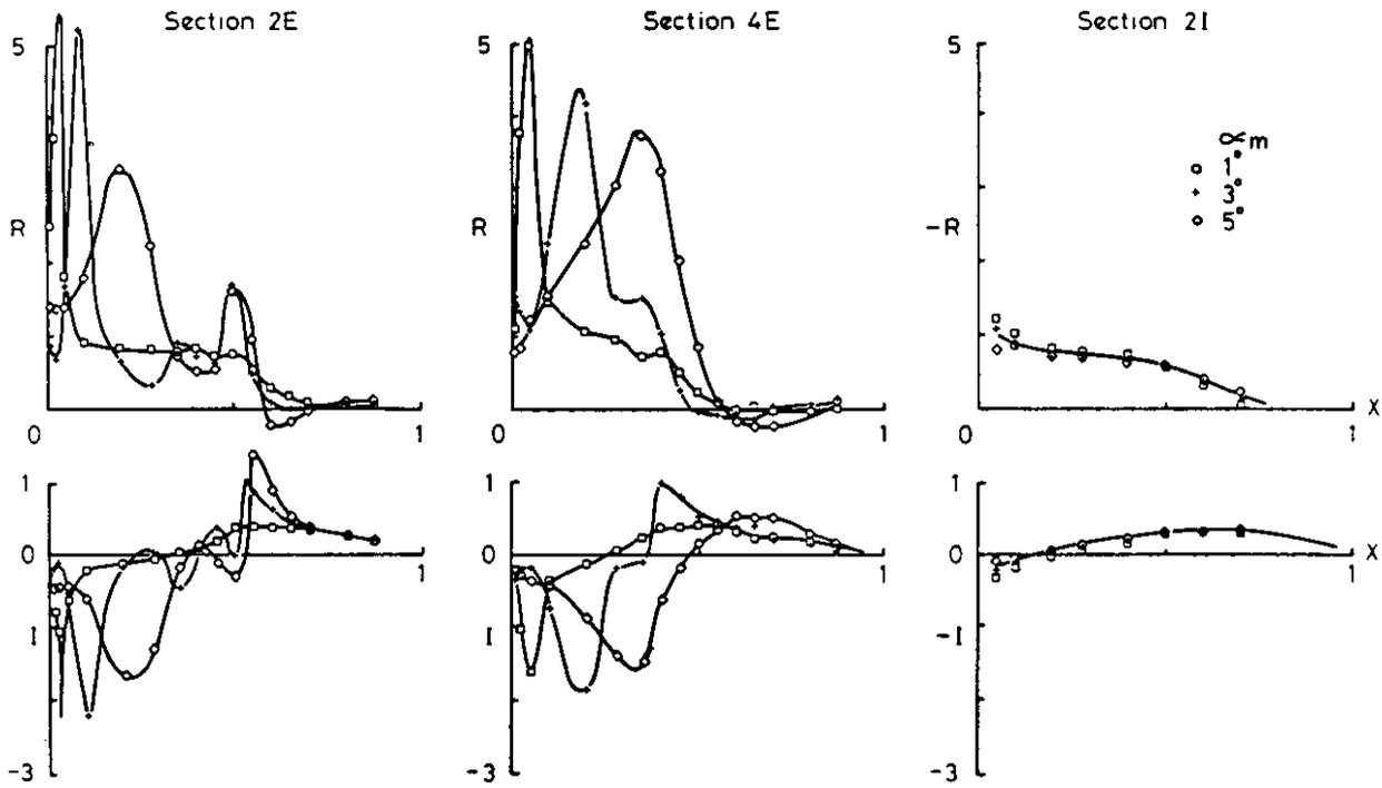
Fig 7.8 Oscillatory pressures. Influence of incidence,  $M = 0.90$ ,  $f = 40$  Hz
