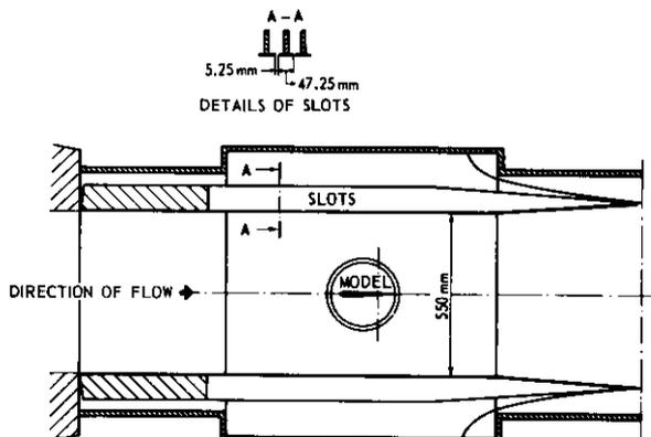
Fig. 4.10 Transonic test section of the NLR Pilot Tunnel
