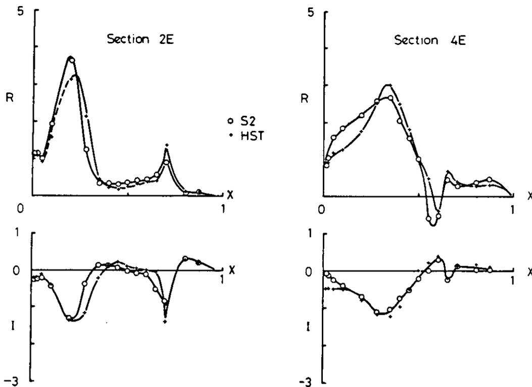
Fig 7.21 Oscillatory pressures. Comparison of data from S2 and HST.
