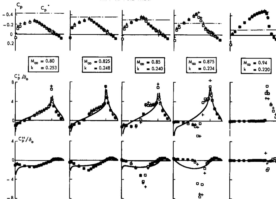
Fig. 1.1 Development of mean steady and unsteady pressure distributions with Mach number (f = 120 Hz)
