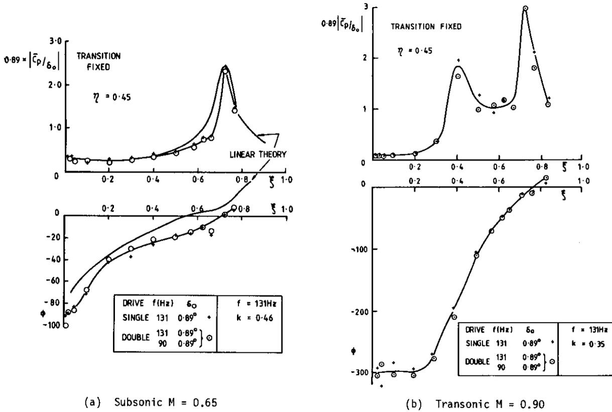
Fig 6.5 Superposition of two frequencies
