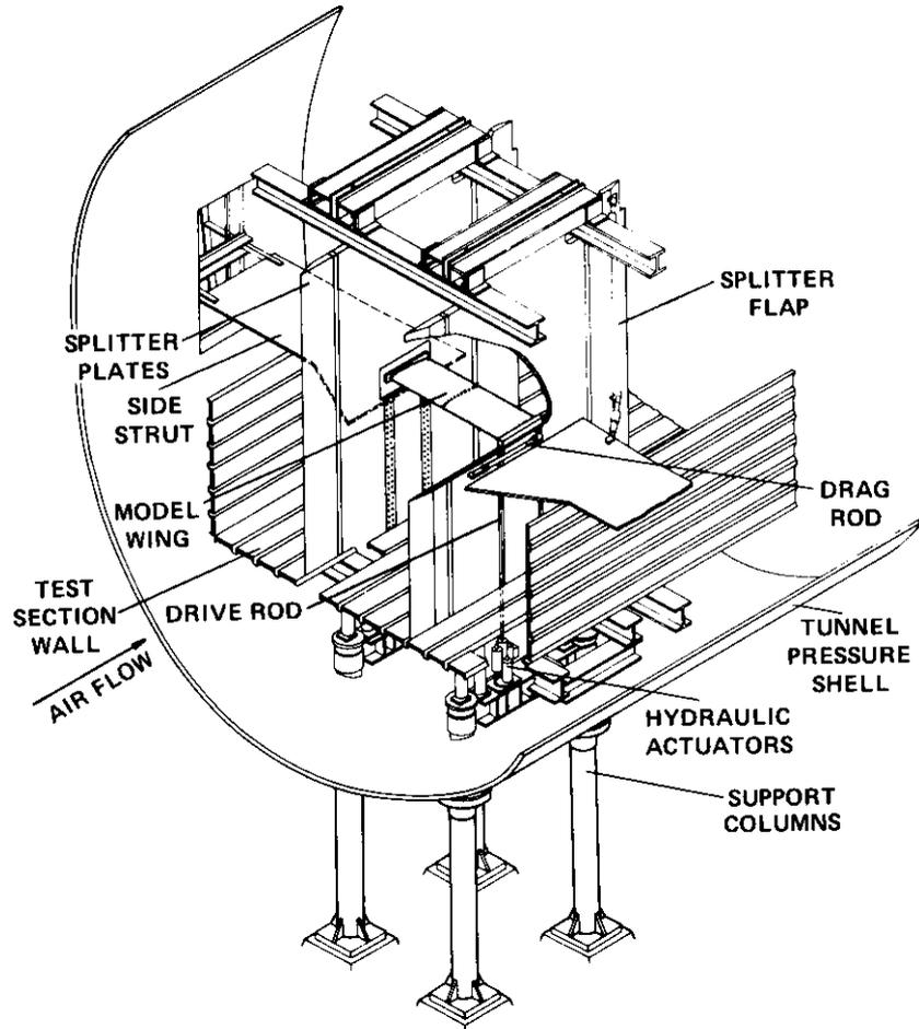
Fig. 5.1. General arrangement of oscillating airfoil test apparatus in NASA AMES 11- by 11-Foot Transonic Wind Tunnel.
