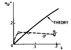
Fig. 4.3 Unsteady normal-force and moment coefficients as a function of frequency in transonic flow with a well-developed shock wave; pitching oscillation
