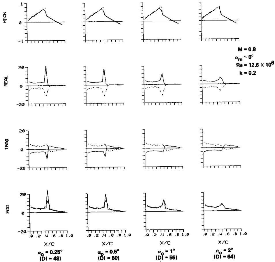
Fig. 2.3. Effect of varying oscillation amplitude.
