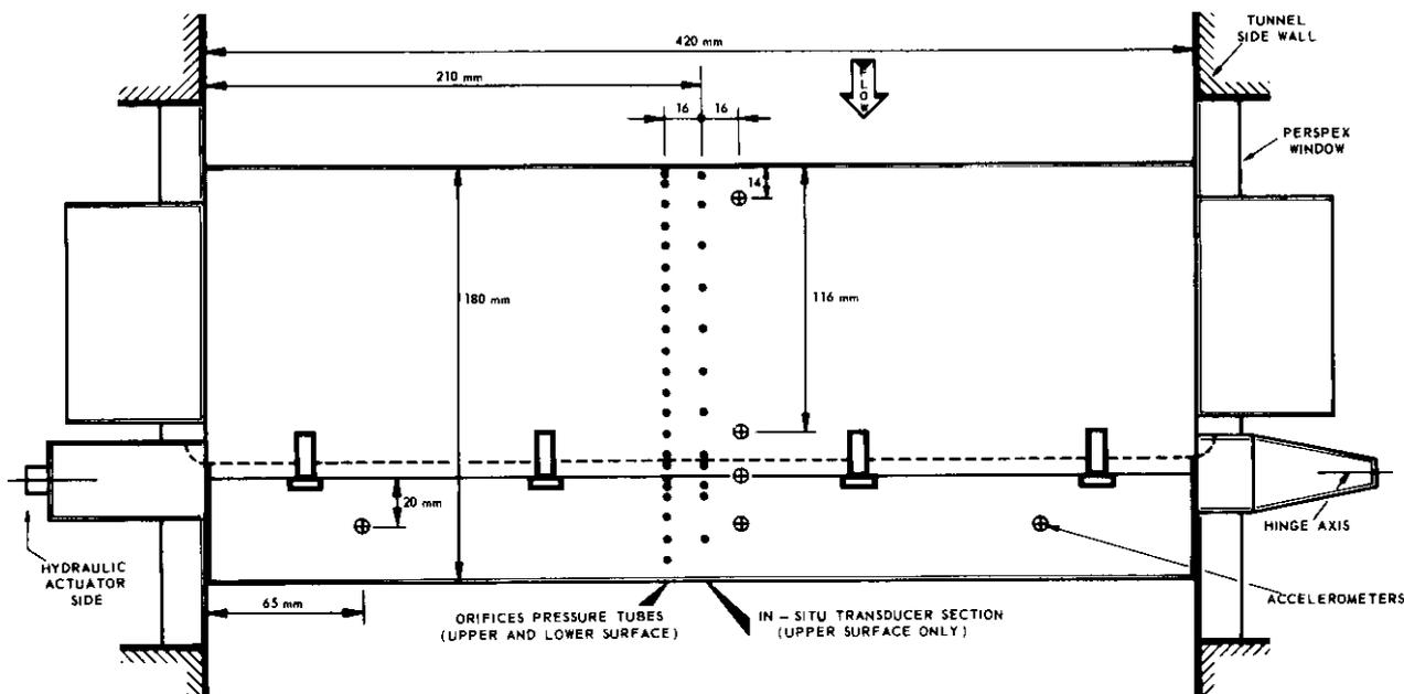
Fig. 4.15 Test set-up and instrumentation of the NLR 7301 airfoil with control surface (Conf. B)
