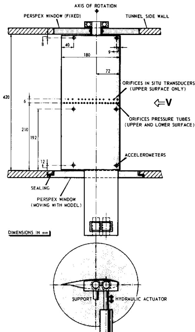
Fig. 4.13 Test set-up and instrumentation of the NLR 7301 airfoil (Conf. A)
