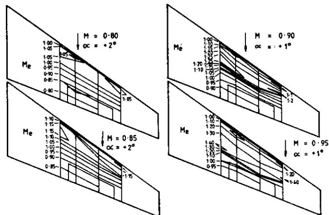
Fig 6.3 Mean isomach contours: suction surface
