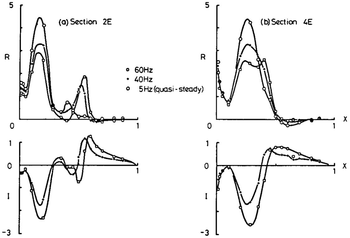
Fig 7.14 Oscillatory pressures,  $M = 0.90$ ,  $\alpha_m = 4^\circ$ . Influence of frequency
