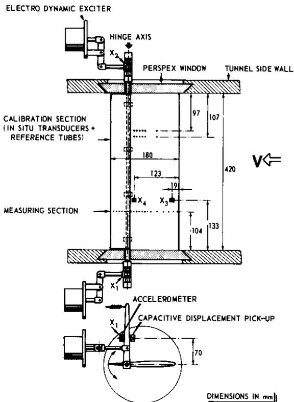
Fig. 1.7 Test set-up and instrumentation of the NACA 64A006 airfoil with flap
