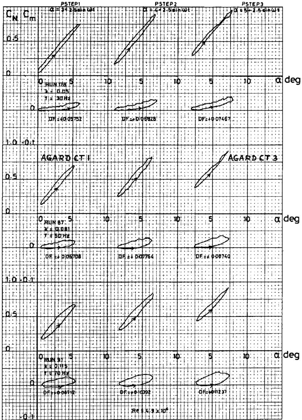
Fig 3.2  $C_N, C_m$  v. incidence over range of  $\alpha_m = 3^\circ, 4^\circ, 5^\circ$ ;  $\alpha_0 = 2.5^\circ$ .
