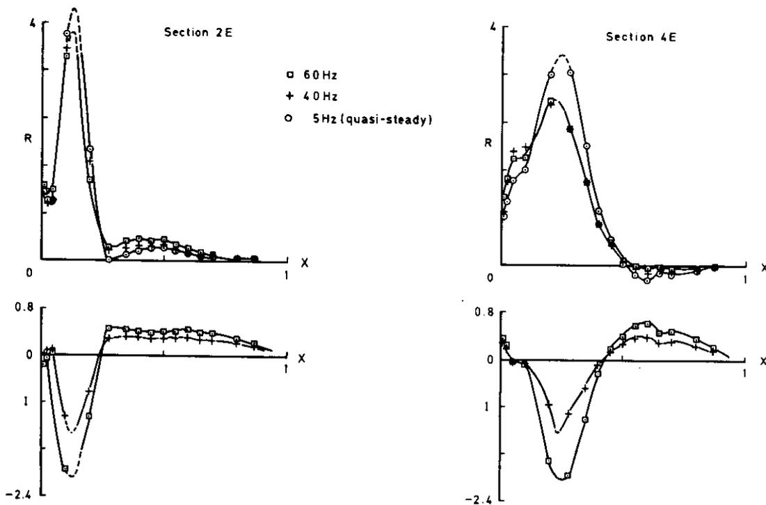
Fig 7.13 Oscillatory pressures,  $M = 0.80$ ,  $\alpha_m = 4.0^\circ$ . Influence of frequency
