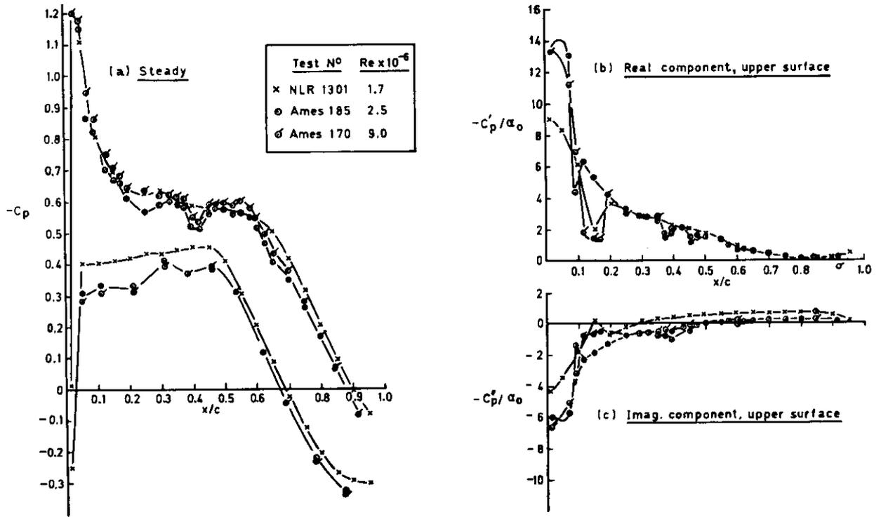
Fig 0.4 NLR 7301 Airfoil. Comparison of NLR and Ames data relating to CT Case 2 (subsonic M = 0.5)
