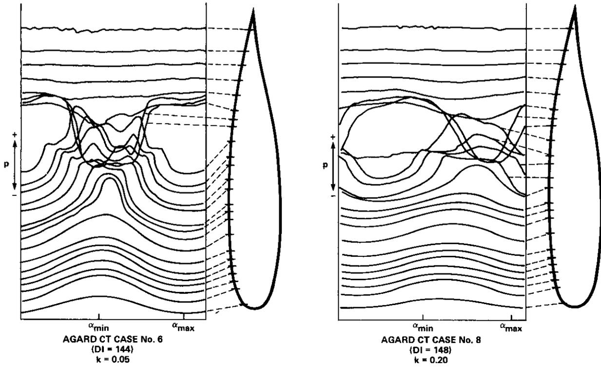
Fig. 5.11. Unsteady pressure time-histories for supercritical design case.  $M = 0.721$ ,  $\alpha_m = 0.19^\circ$ .
