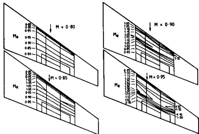
Fig 6.2 Mean isomach contours:  $\alpha = 0$
