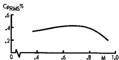
Fig. 4.12 Noise level in NLR Pilot Tunnel test section
