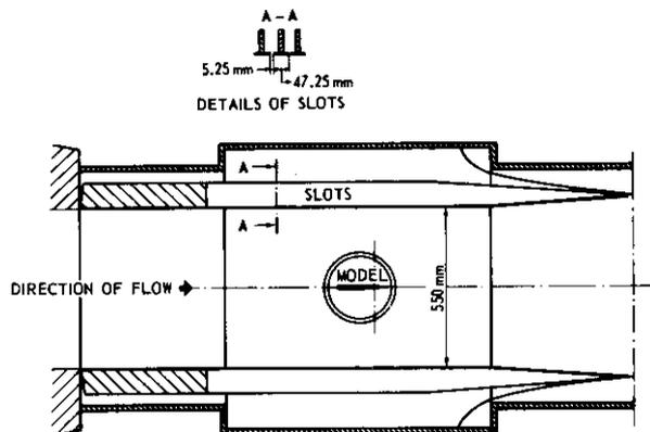
Fig. 1.4 Transonic test section of the NLR Pilot Tunnel
