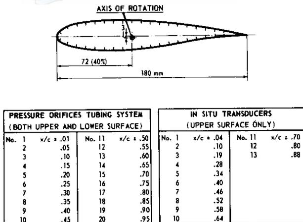
Fig. 4.14 Location of pressure orifices of the NLR 7301 airfoil (Conf. A)
