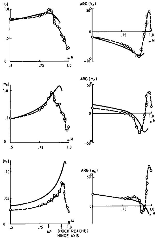
Fig. 1.2 Unsteady aerodynamic coefficients as a function of Mach number ( $f = 120$  Hz)
