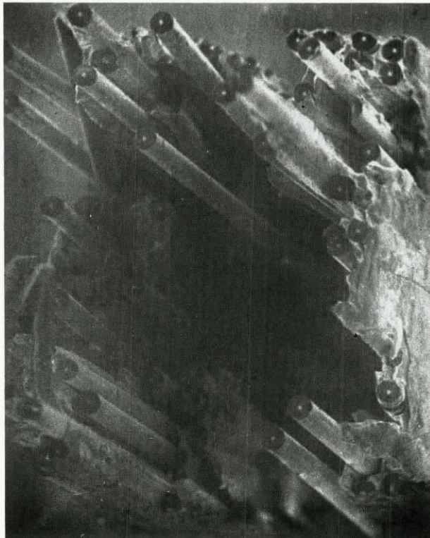
Figure 5. Surface of rupture of MMCs with insufficient interaction of components: (a) Al-C ( \times 146 ); (b) Al-B ( \times 80 )
