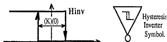
Figure 13 : Hysteresis inversion : a fundamental non-linearity.
