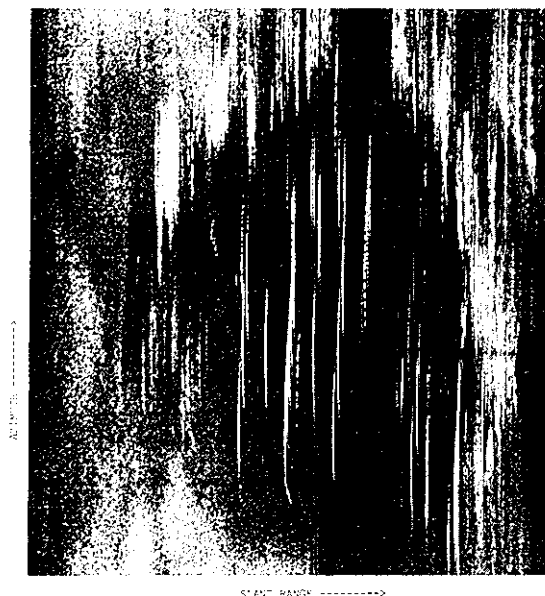
Fig. 16 Raw data: RCM corrected, range compressed image before the azimuth processing.
