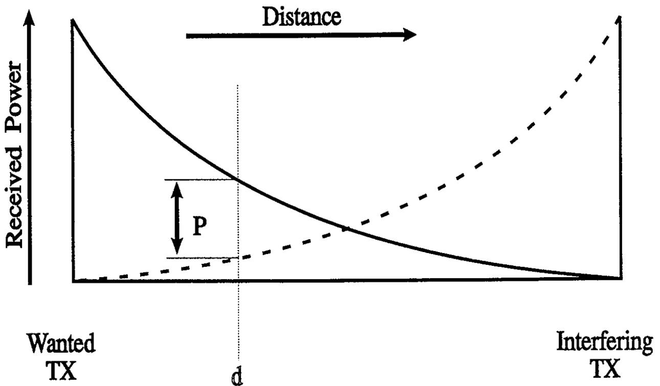
Figure 17: Illustration of frequency dependent rejection
