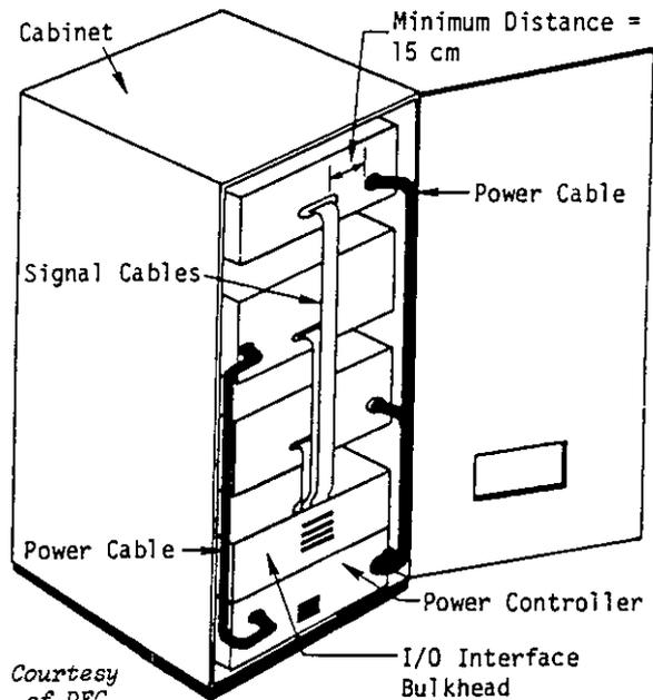
Fig. 2.15.4. Mounting of cables.
