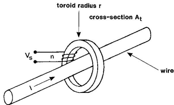
Fig 2.13. Current Transformer.
