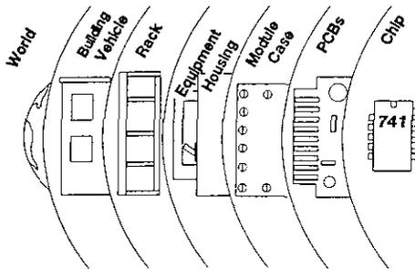
Fig. 1.2. EMC-levels of a system.
