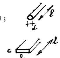
It follows that low impedance may be achieved by using a multiwire, small diameter combination or a very large plate.
