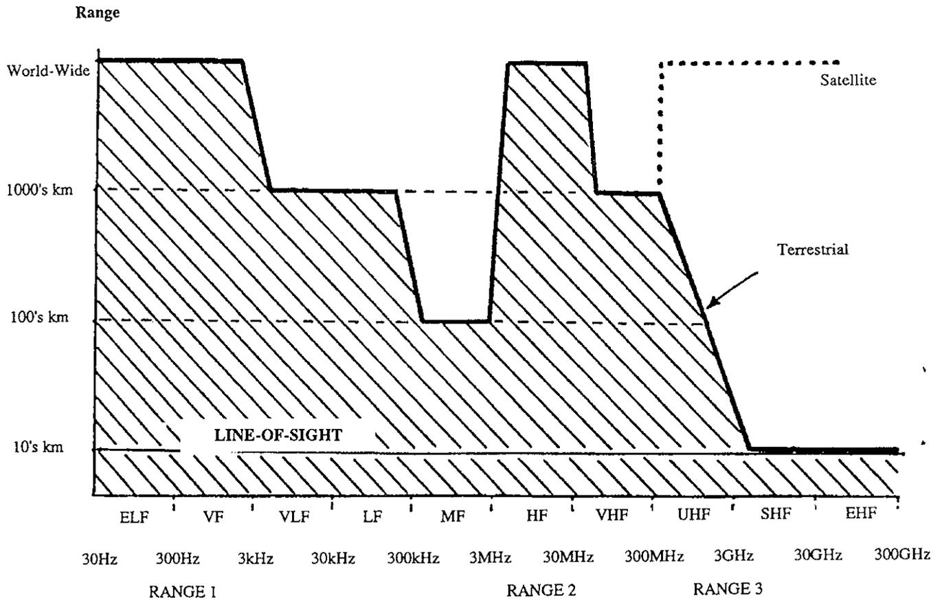
**Figure 4: Variation of Radio System Range With Frequency**
