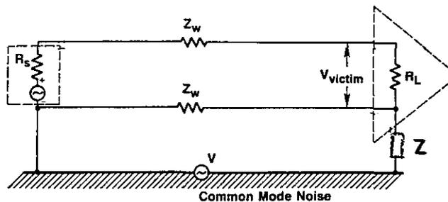
Fig. 2.3.1. Unbalanced system.
