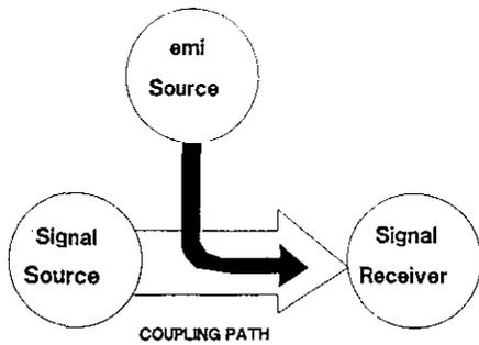
Fig. 1.1. EMC transmission path
