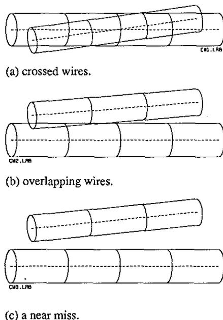
Fig. 15 Wire spacing errors for nearly parallel wires.
