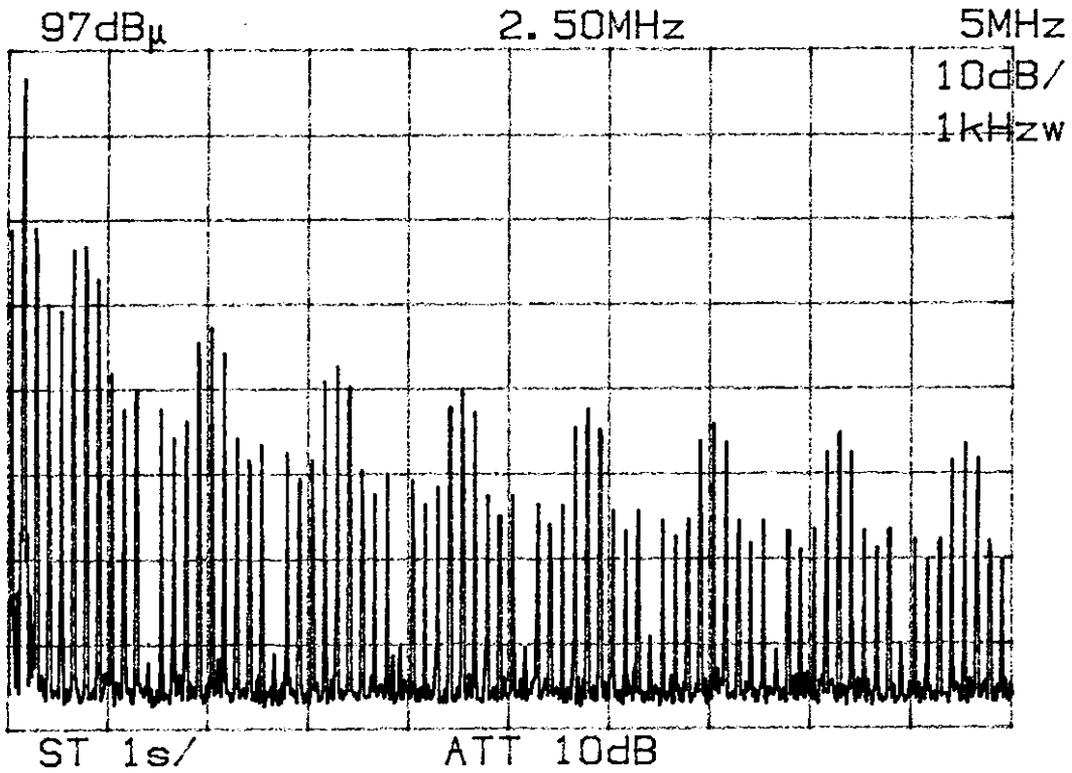
Fig 1.1. Spectrum of Harmonics from a Digital Circuit.
