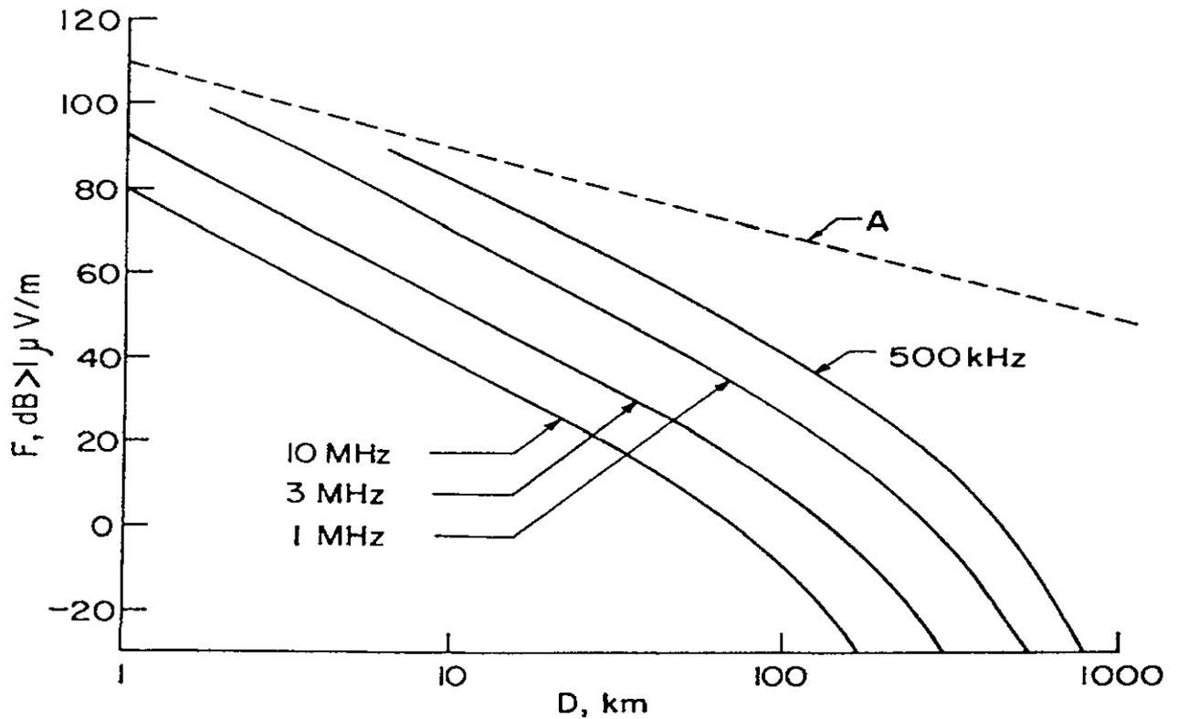
Figure 8: Groundwave Field-Strength variation with Distance (CCIR 368-2)
