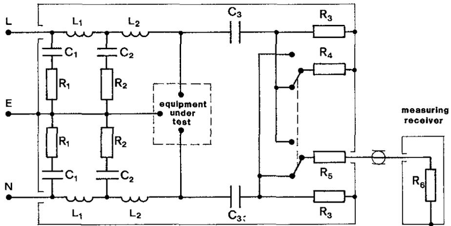
Fig 2.16. LISN Circuit Diagram.
