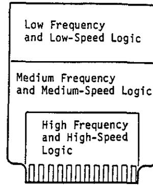
Fig. 2.15.2. Component placement on PCB.
