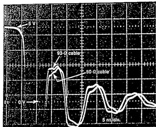
Fig. 2.9.2. Example of ringing due to line-reflections.
