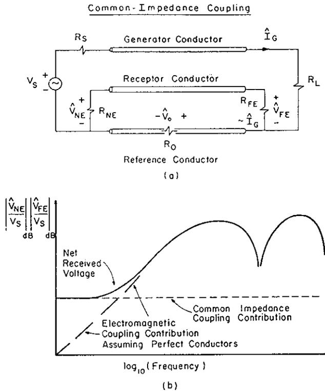
Fig. 12. Common-impedance coupling due to imperfect conductors
