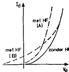
Fig. 2.13.2. DC-shift of diode-circuit due to HF demodulation.
