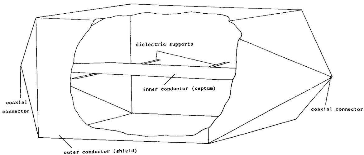
Fig 2.20. Cross-Section of a Crawford Cell.
