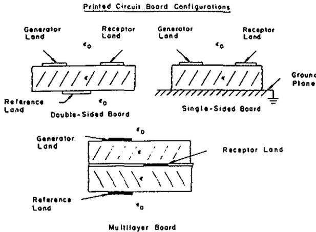
Fig. 4. Cross-sectional configurations of PCB lands
