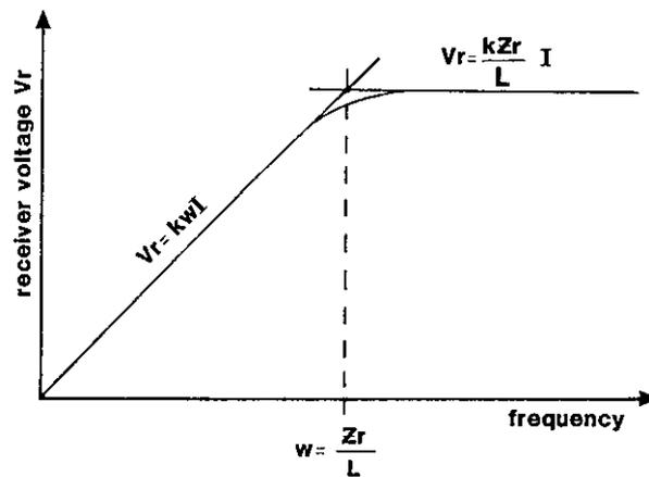
Fig 2.14. Frequency Response of Current Transformer.
