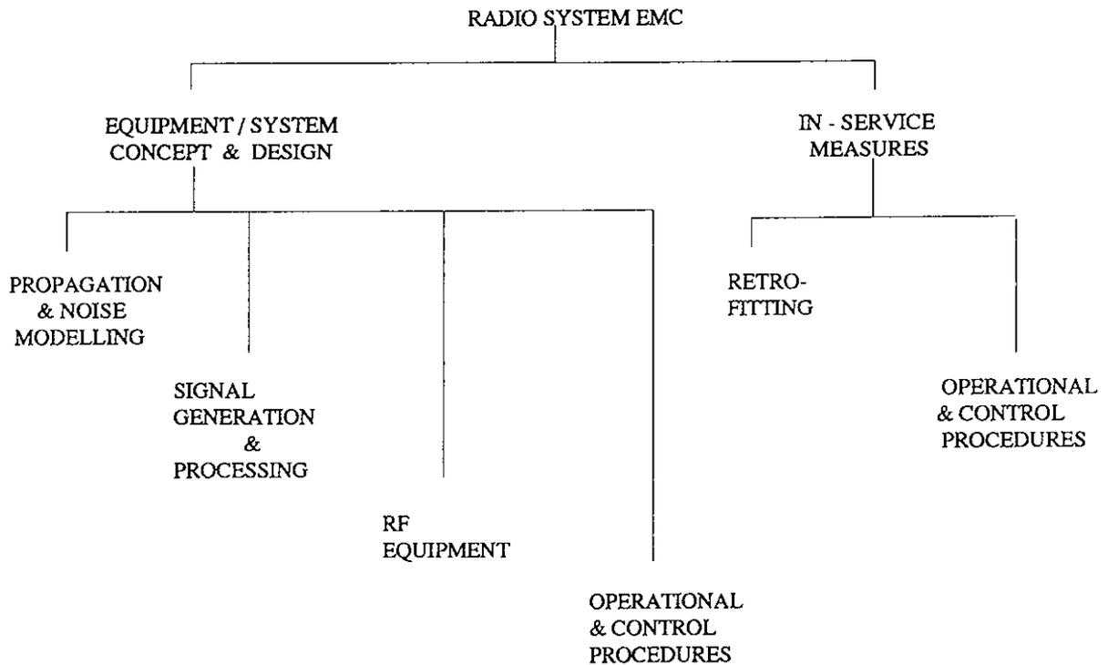
Fig. 12 Elements of radio system EMC
