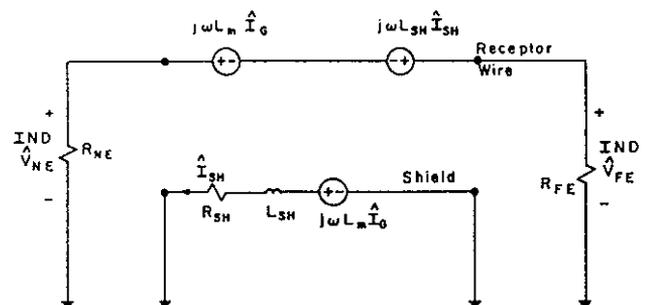
Fig. 15. Simplified model for inductive coupling to a shielded receptor wire
