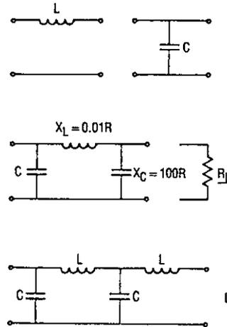
Fig. 2.7.1. Basic filter components.
