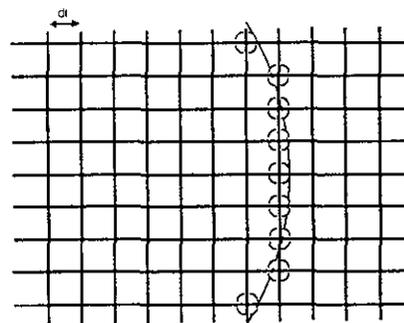
Fig. 18(b) Wavefront superimposed on TLM mesh showing approximate scattering centres.
