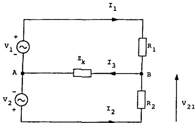
Fig. 2.1. Examples of common impedance.
