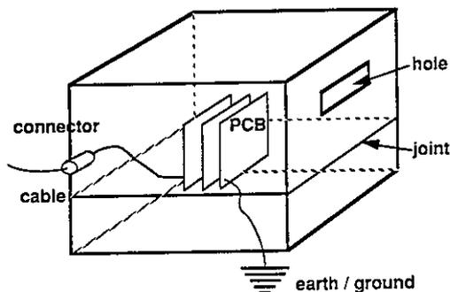
Fig. 2.10.1. Example of housing.
