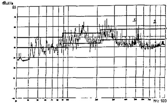
Fig. 2.1. : Emission spectrum from a PCB.
