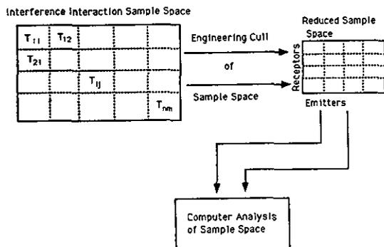
Fig. 1 Interference Interaction Matrix
