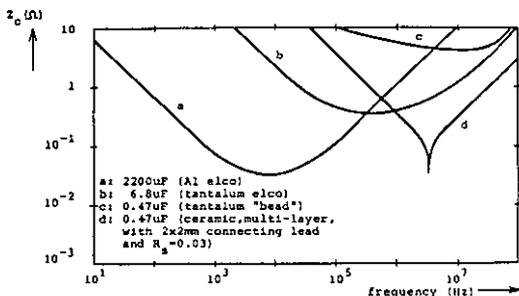
Fig. 2.11.2. Decoupling capacitors.
