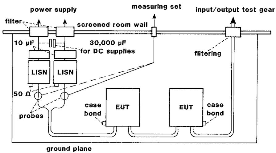
Fig 2.18. Conducted Interference Measurement Layout.
