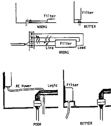
Fig. 2.6.2. Mounting of power line filter.
