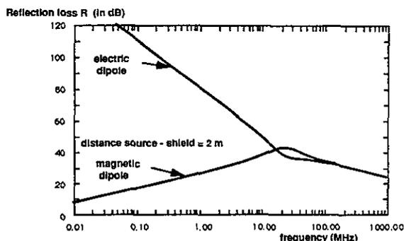
Fig. 2.4. : Reflection loss R as function of frequency
