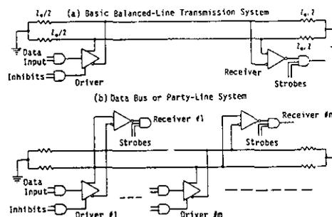
Fig. 1.2. : Characteristic impedance for matching bus systems.
