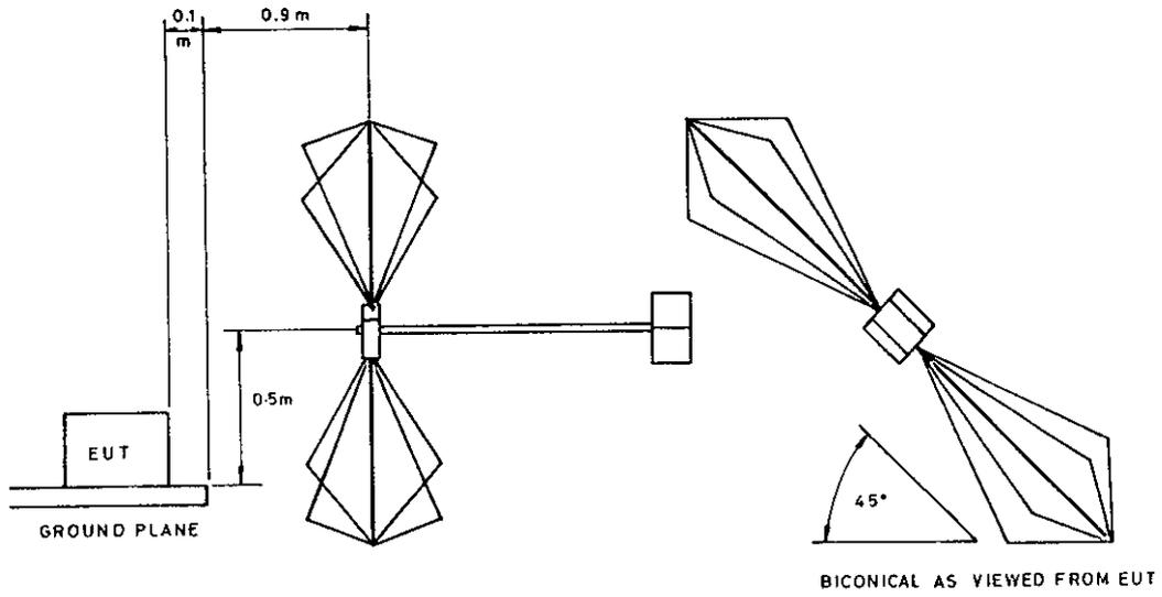
Fig 2.11. EUT and Antenna for 30 - 200MHz.
