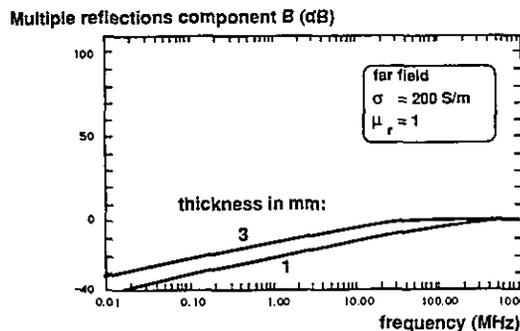
Fig. 2.6.: Re-reflection B as function of frequency
