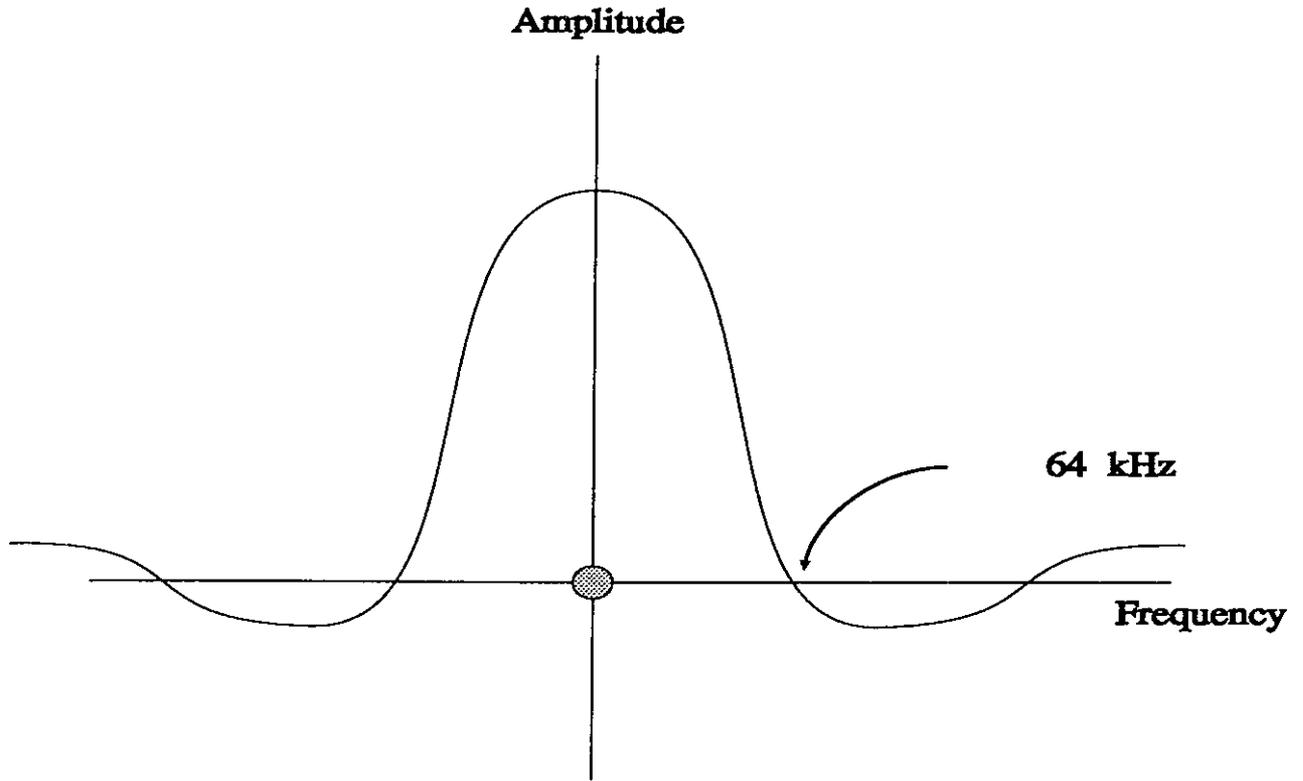
Figure 14: Spectrum of 64 kbits/sec digital signal
