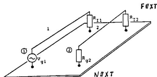
Fig. 2.8.1. Crosstalk of two wires.
