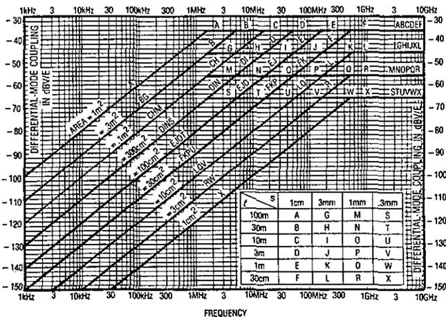
Fig. 2.4.2. DM coupling E-field/loop voltage (ref. D. White/ICT)
