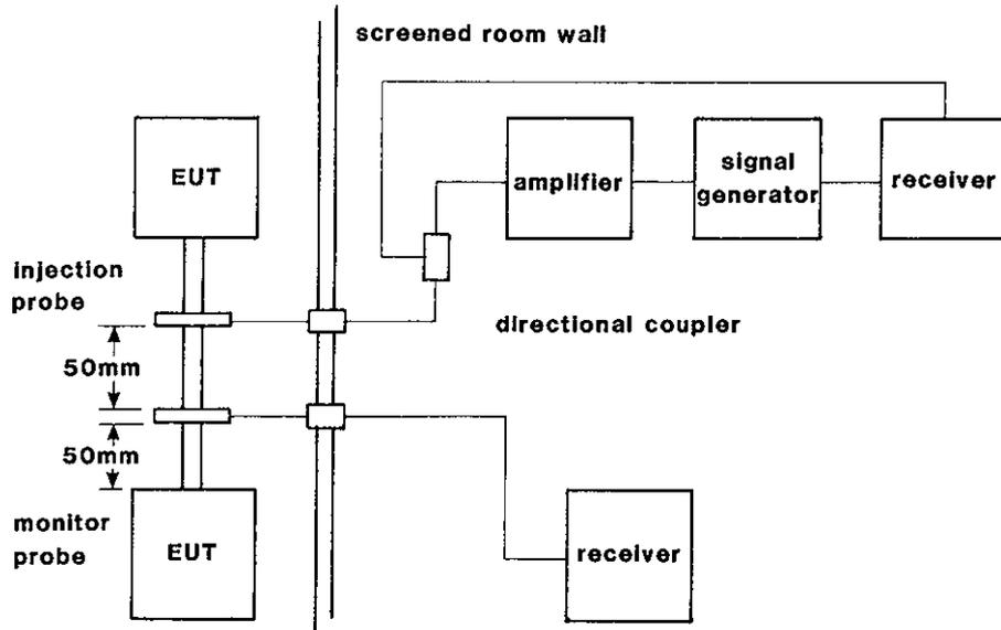
Fig 2.21 Bulk Current Injection Test System.
