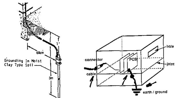
Fig. 3.1. : Wires for bonding.
