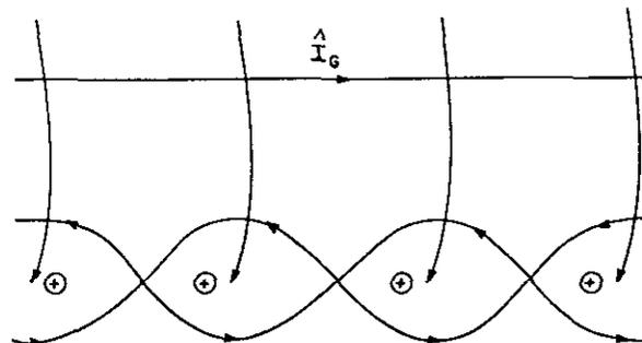
Fig. 19. Effect of a twisted pair on inductive coupling
