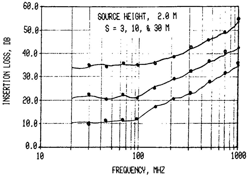
attenuation for horizontally polarised dipoles over perfect ground. Solid curves are calculated, points are measured data
