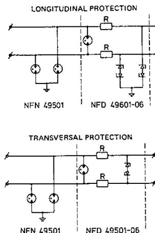
Fig. 2.12.1. Principle protection for electrical overstress.
