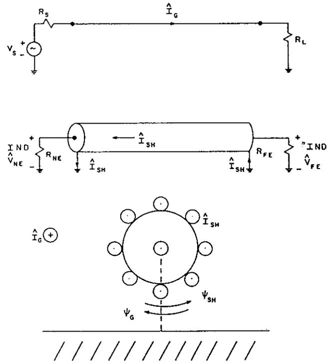
Fig. 14. Effect of a shield on inductive coupling
