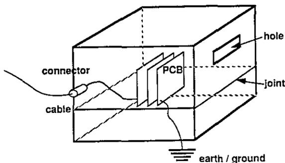
Fig. 0.1. : Coupling of systems to fields.
