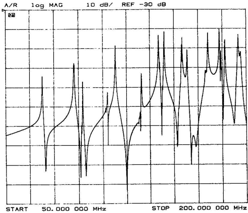
Fig 2.12. Frequency Response of Screened Enclosure 30 - 200MHz.
