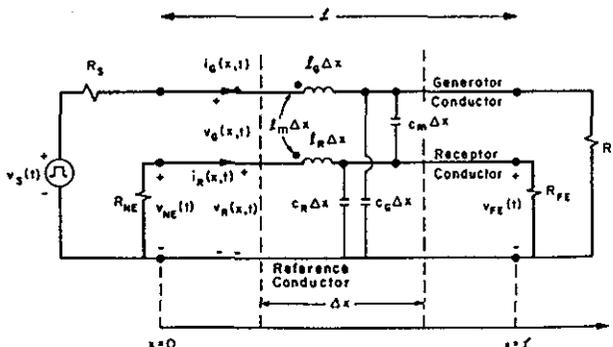
Fig. 5. The per-unit-length transmission-line model
