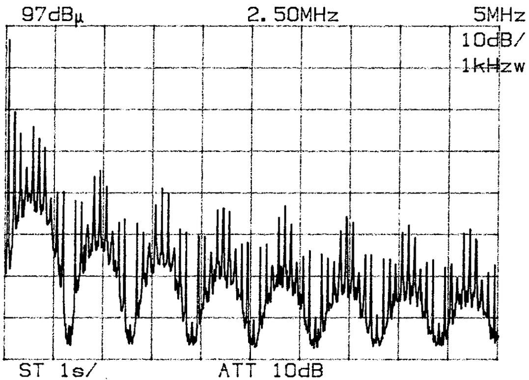
Fig 1.2. Continuous Spectrum of Digital Data.
