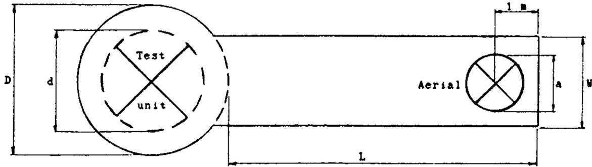
$D = d + 2 m$ , where  $d$  is the maximum test unit dimension;
