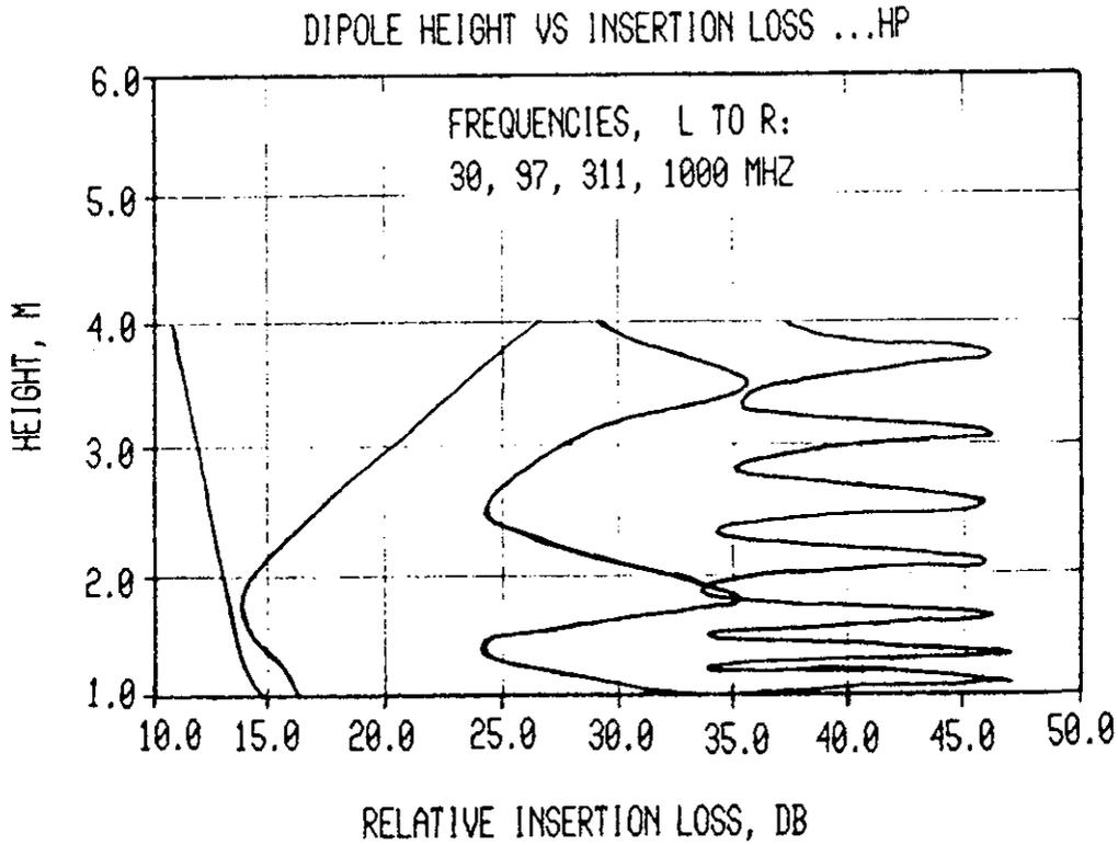
Selected relative insertion loss data calculated for horizontally polarized, dipoles over perfect ground. Site attenuation is the single minimum insertion loss value of each curve. Separation distance is 3 m; transmitting dipole height is 2 m.
