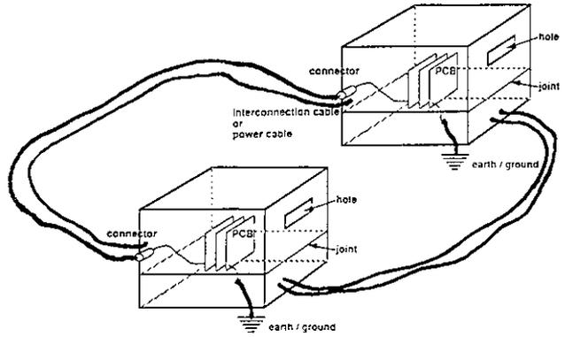
Fig. 1.4. : Return current flowing over earth.
