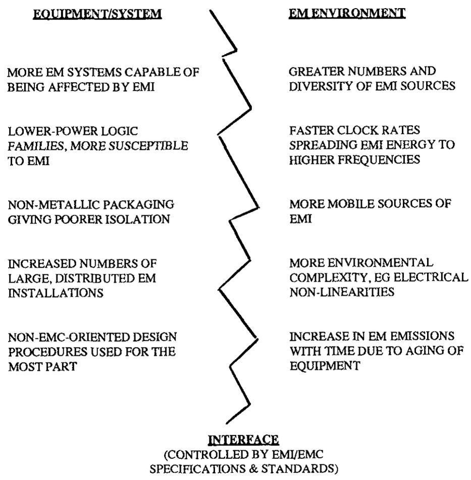
Fig. 1: EMC as an interface control problem
