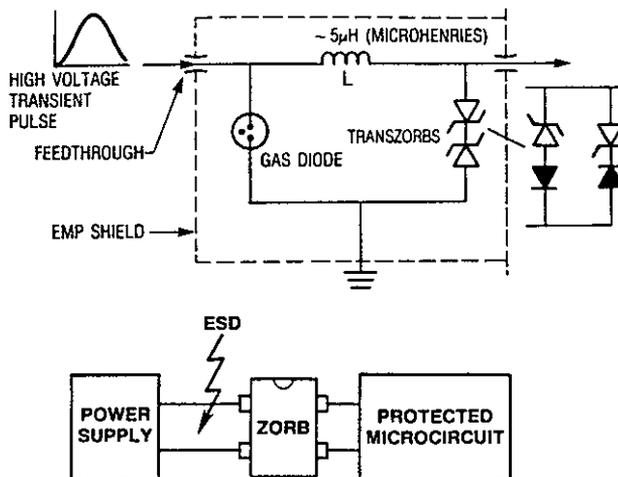
Fig. 2.12.2. Typical protection devices.
