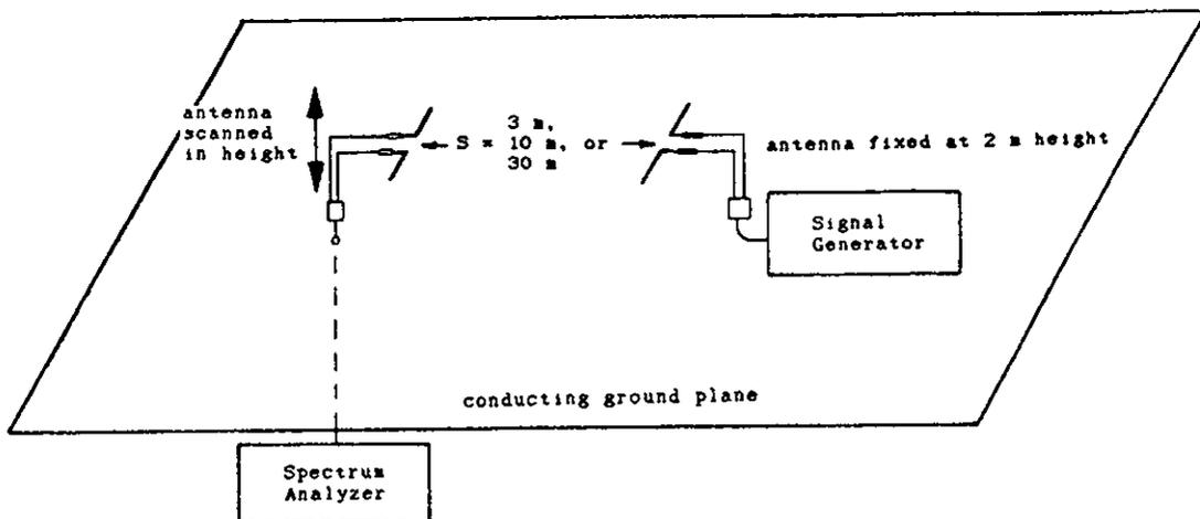
Fig 2.5. Antenna Positions for OFTS Site Attenuation.
