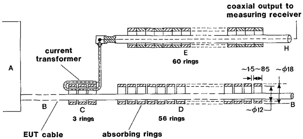
Fig 2.15. Absorbing Clamp Construction.
