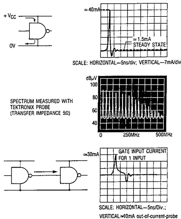
Fig. 2.11.1. Current during state transitions.
