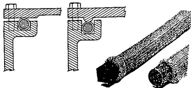
Fig.3.2.: Applying a gasket in practice
