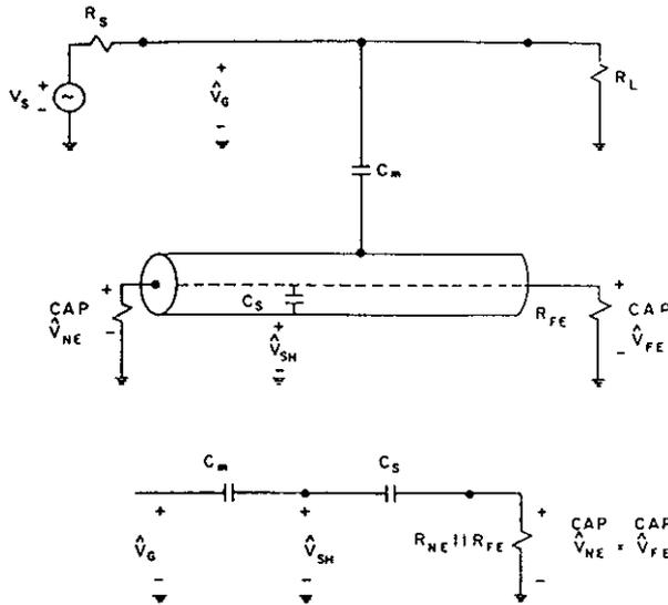
Fig. 13. Effect of a shield on capacitive coupling
