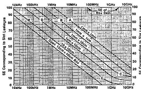
Fig. 2.3.3. : Leakage of slots (ref. Don White/ICT)
