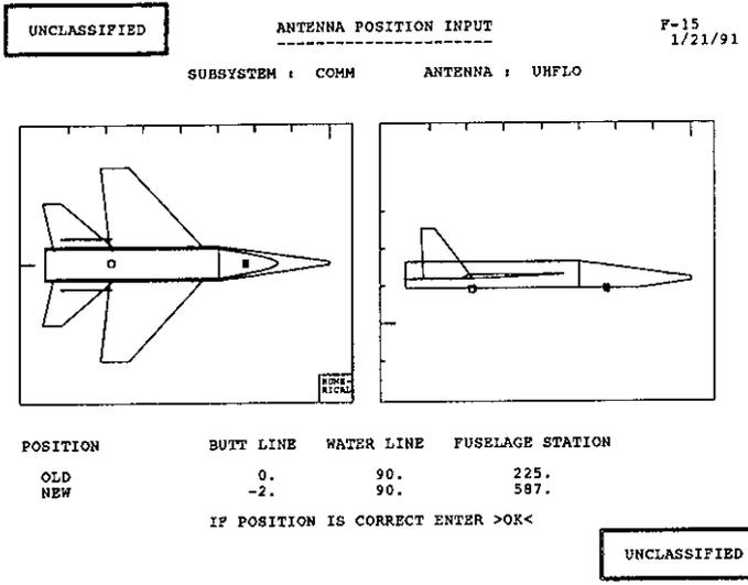
Fig. 9 Antenna Position Input
