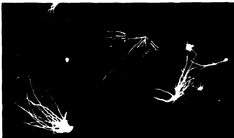
Fig. 5 - Surface streamer produced by charging the fuselage.
