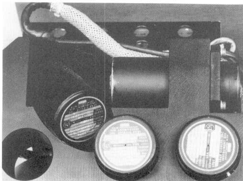
Figure 19. Principle of semiskewed rate gyros applied to a strapdown system used in a BO 105 helicopter.
