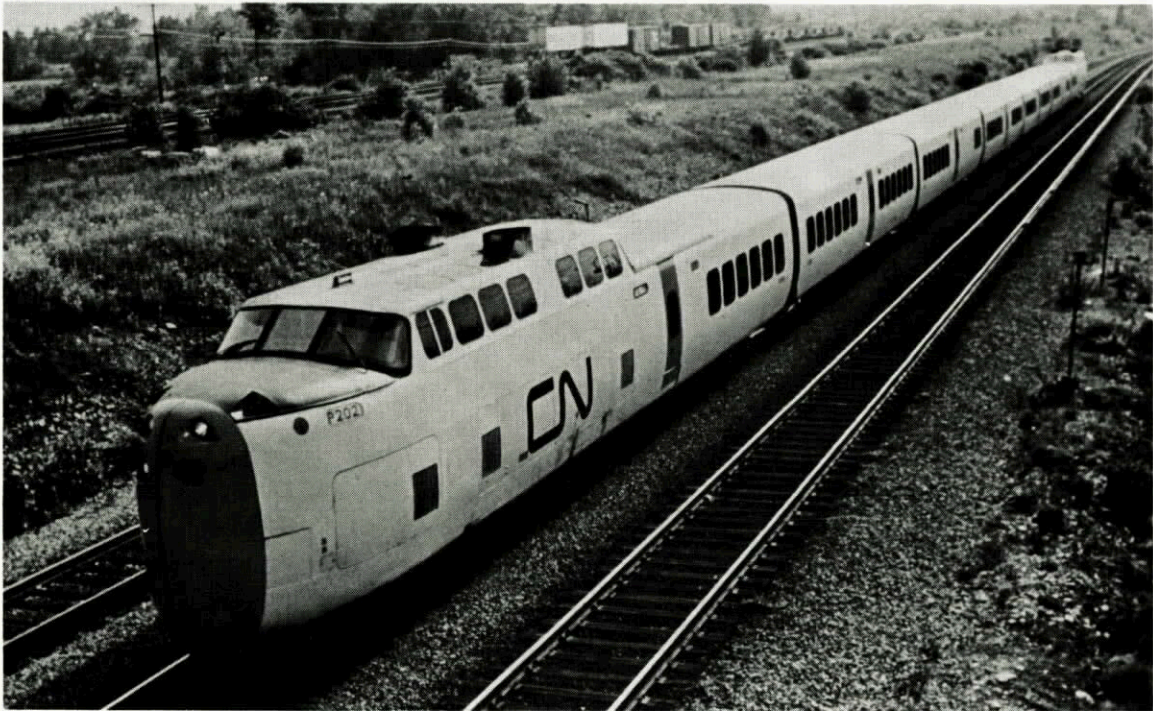
Fig.12 ST6 powered CNR Turbo Train
