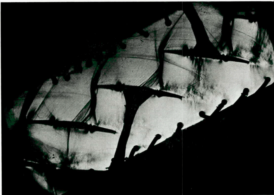
Fig.2.14: Schlieren picture of DCA-cascade at M_\infty = 1.27 and maximum pressure ratio p_2/p_\infty = 1.51 .
