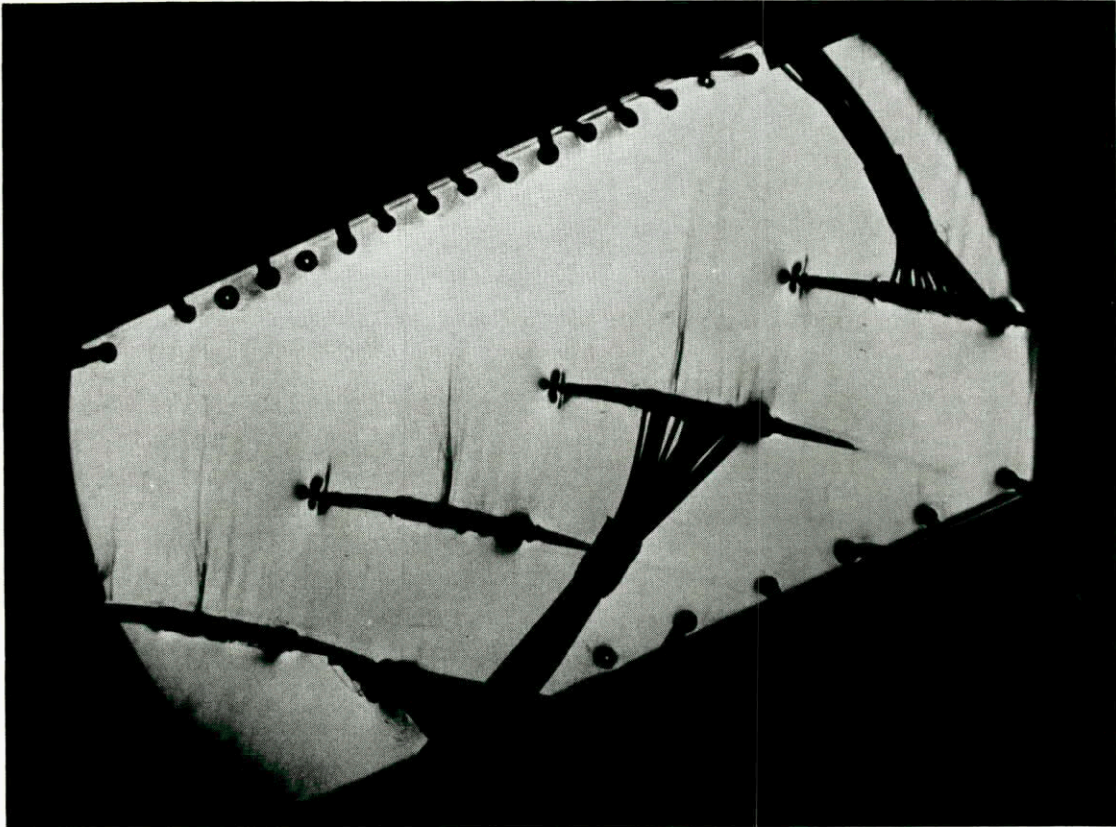
Fig.2.1: Schlieren picture of "Double circular Arc" (DCA)- cascade at subsonic inlet Mach number, M_\infty = 0.9 .
