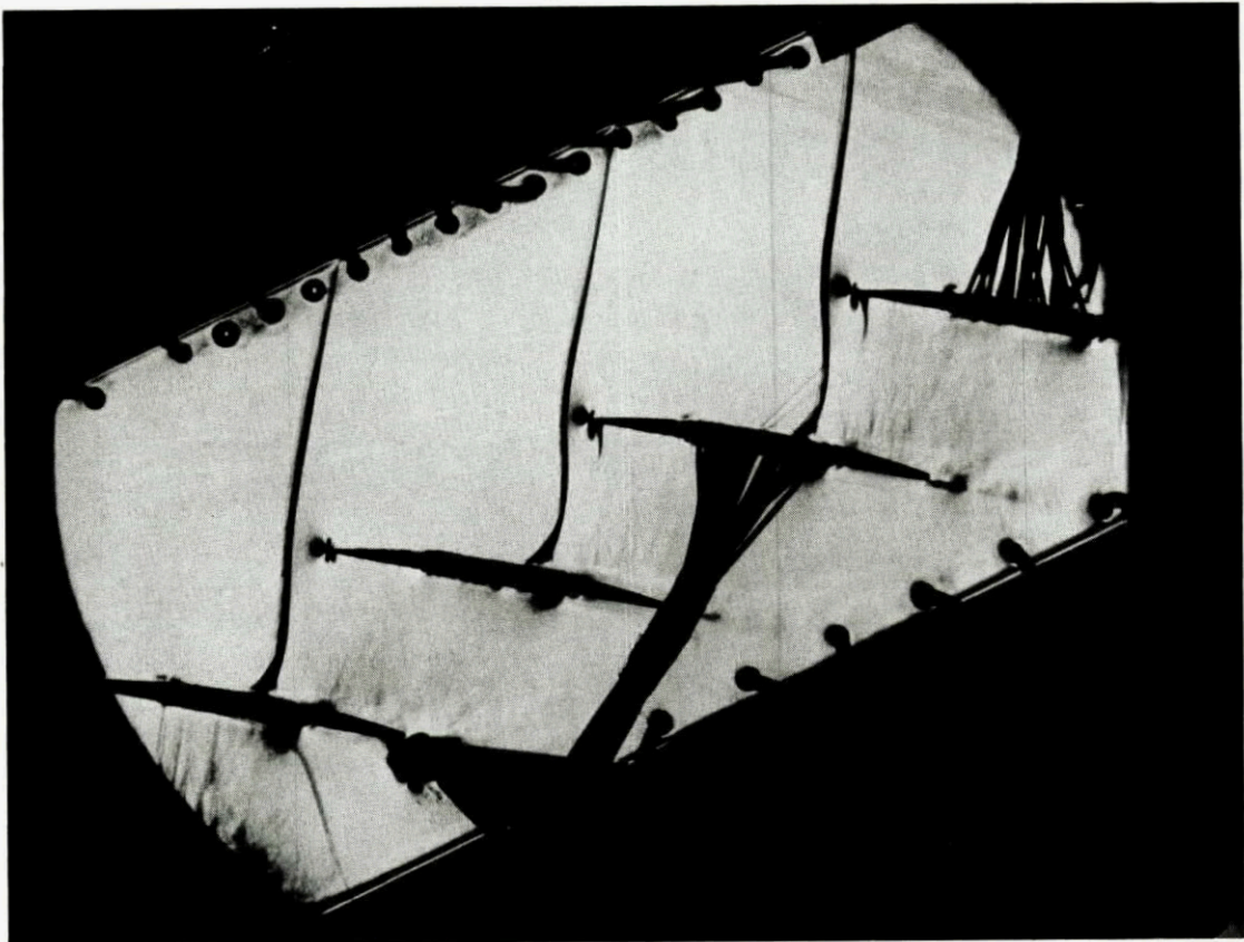
Fig.2.3: DCA-cascade at near sonic inlet velocity, M_\infty = 1.03 .
