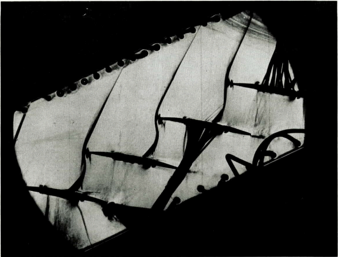
Fig.2.7: DCA-cascade at low supersonic inlet velocity, M_\infty = 1.10 .
