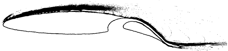
Airfoil With 30 Degree Trailing Edge Flap M = 0.15 Re = 1.7 \cdot 10^6 Total Pressure Loss Contours ( 1 - P/P_0 )
