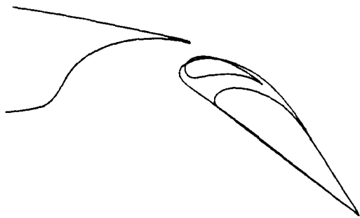
Fig.10a - Comparison of vane-flap and single-slotted systems (0.30c).
