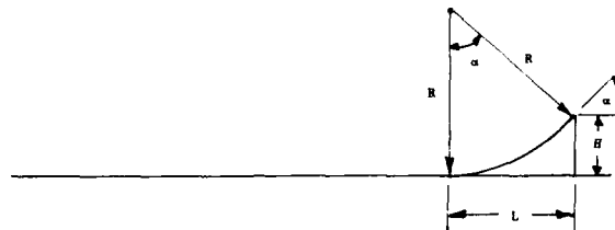
FIGURE A8. RAMP GEOMETRY
