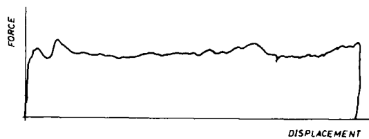
Figure 9. Force-Displacement Characteristic of Splitting Tube
