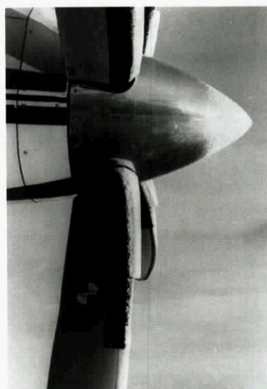
Fig. 3.1-20 Ice formation on propeller and spinner of a SAAB 340
