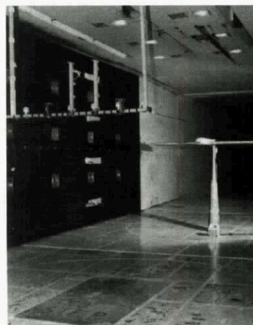
FIG. 34. RAIN SIMULATION SYSTEM IN LANGLEY 4 BY 7 METER SUBSONIC TUNNEL.
