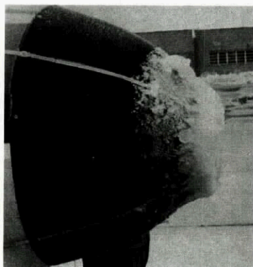
Fig. 3.1-27 Glaze ice formation on radome taken after landing
