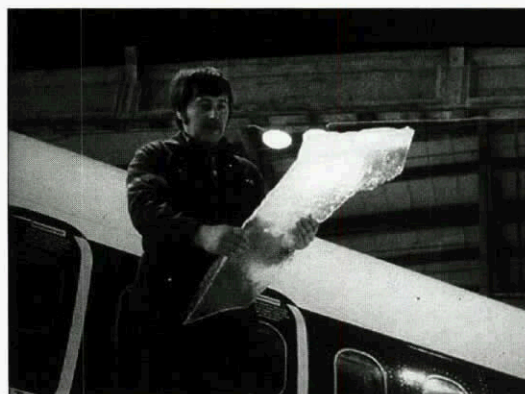
Fig. 3.1-1a A piece of clear ice formed at the wing root of a cold soaked wing
