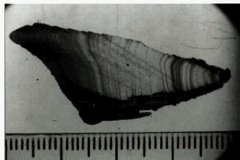
Fig. 3.1-4 Section of an ice accretion showing banded "tree ring" structure associated with variations in growth conditions
