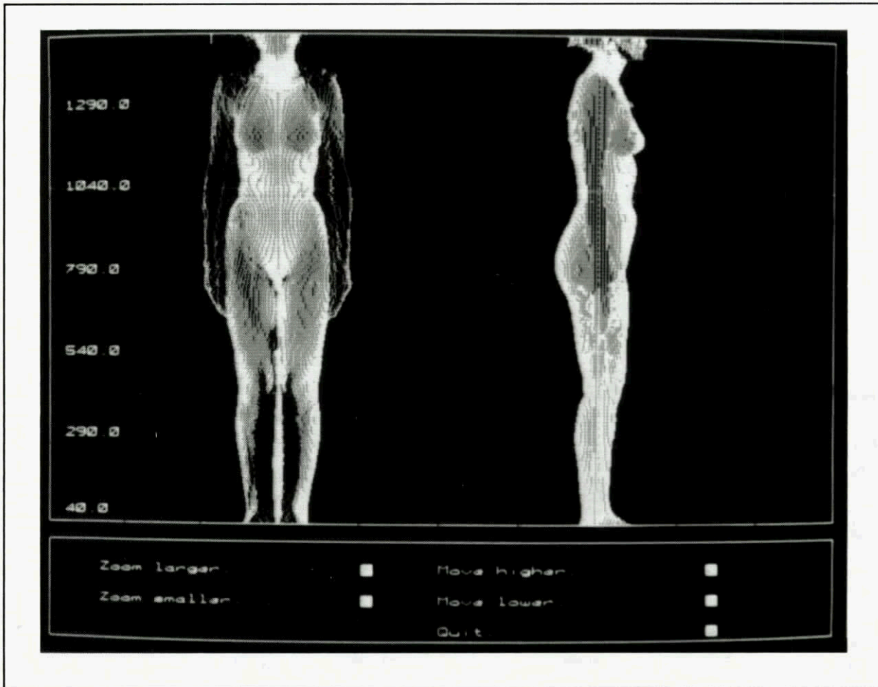
Figure 2-2. Anterior and lateral views of part of a subject scanned in high resolution (i.e., vertical slices taken in 2.5° increments at 5 mm horizontal cuts).
