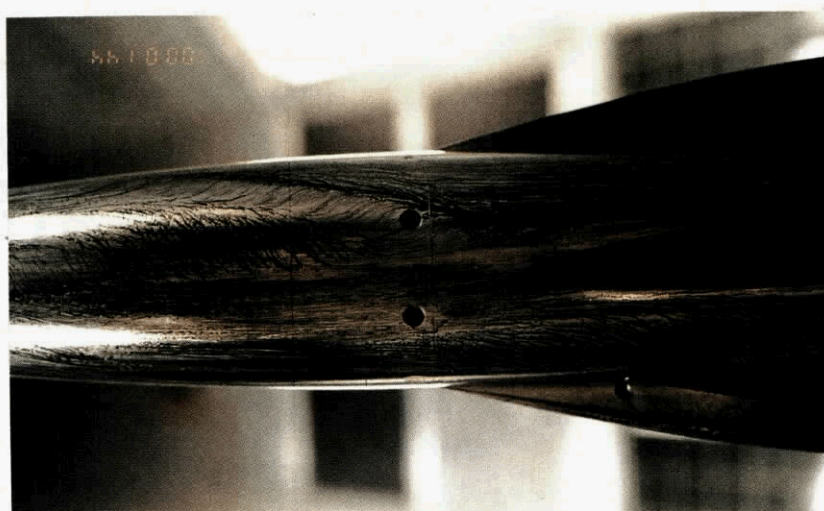
Fig A4.2.9 Forebody/LEX flow pattern at \alpha = 51^\circ , \phi_m = 180^\circ
