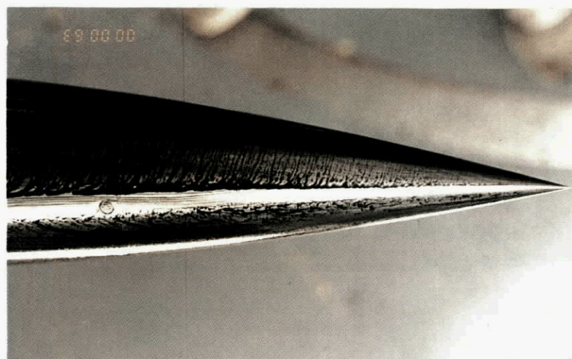
Fig A4.2.3 Forebody flow pattern at \alpha = 41^\circ , \phi_m = 90^\circ
