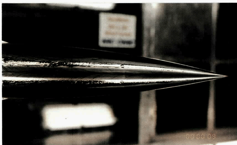
Fig A4.2.1 Near-symmetric forebody leeward flow pattern ( \alpha = 30^\circ )
