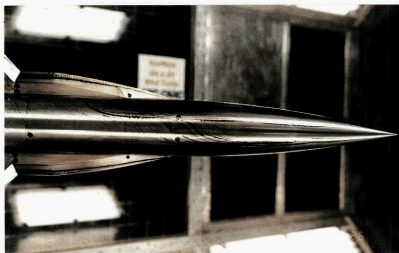
Fig A4.2.2 Asymmetric forebody leeward flow pattern ( \alpha = 39^\circ )
