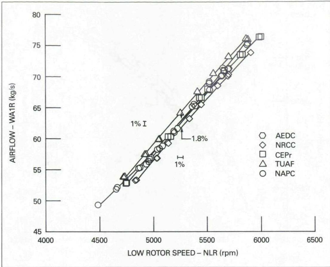
Fig.6 Facility airflow (engine 615037)
