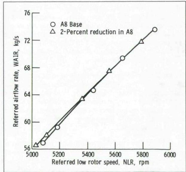
Fig.17-1D Effect of exhaust nozzle area on airflow based on low rotor speed (TC6-607594)
