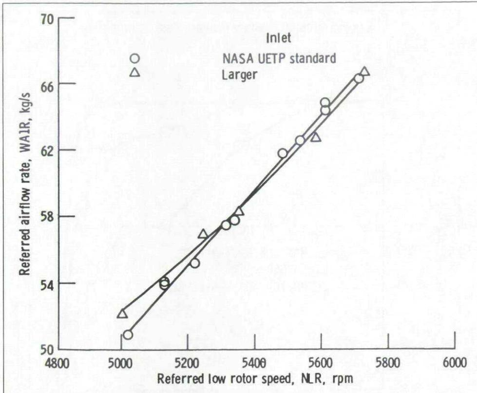
Fig.17-3C Effect of inlet duct on airflow (TC 9)
