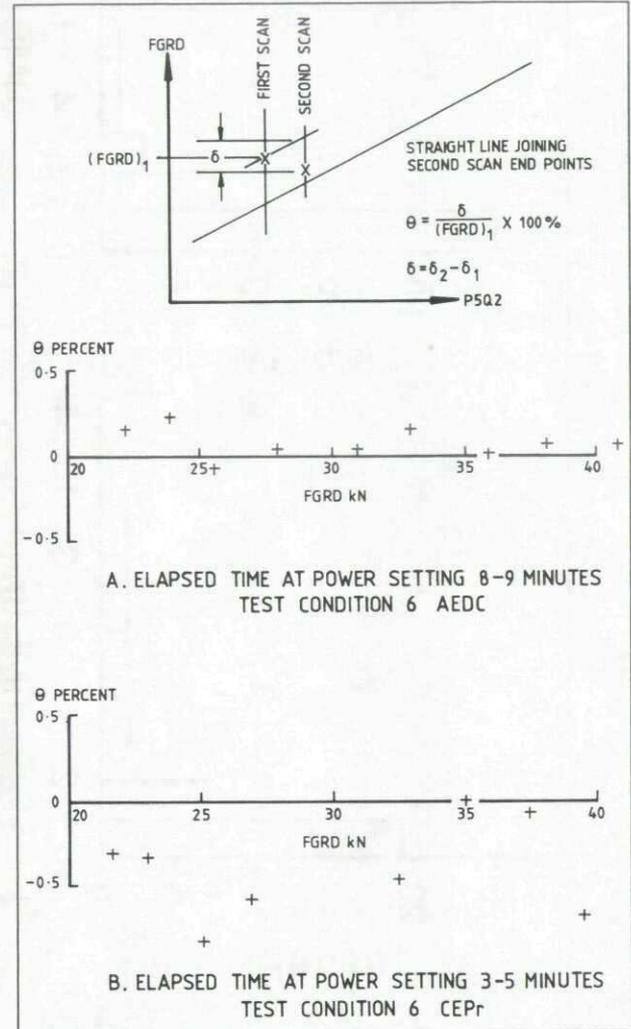
Fig.12-6 Differences in gross thrust between first and second data scans
