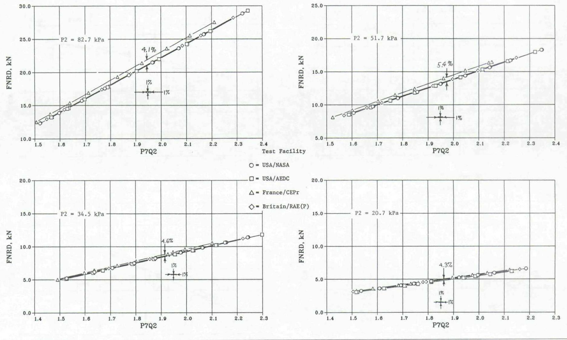
Fig.9-2e Altitude facility net thrust comparison with variable inlet pressure (engine 607954)
