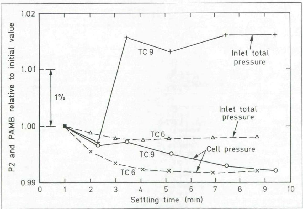
Fig.12-4 Inlet and cell pressures during stabilisation time
