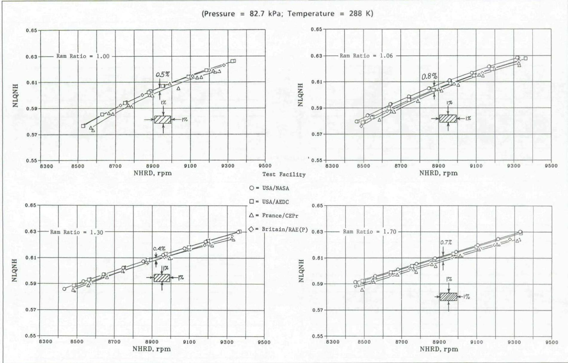
Fig.9-3a Altitude facility speed match comparison with variable RAM ratio (engine 607954)
