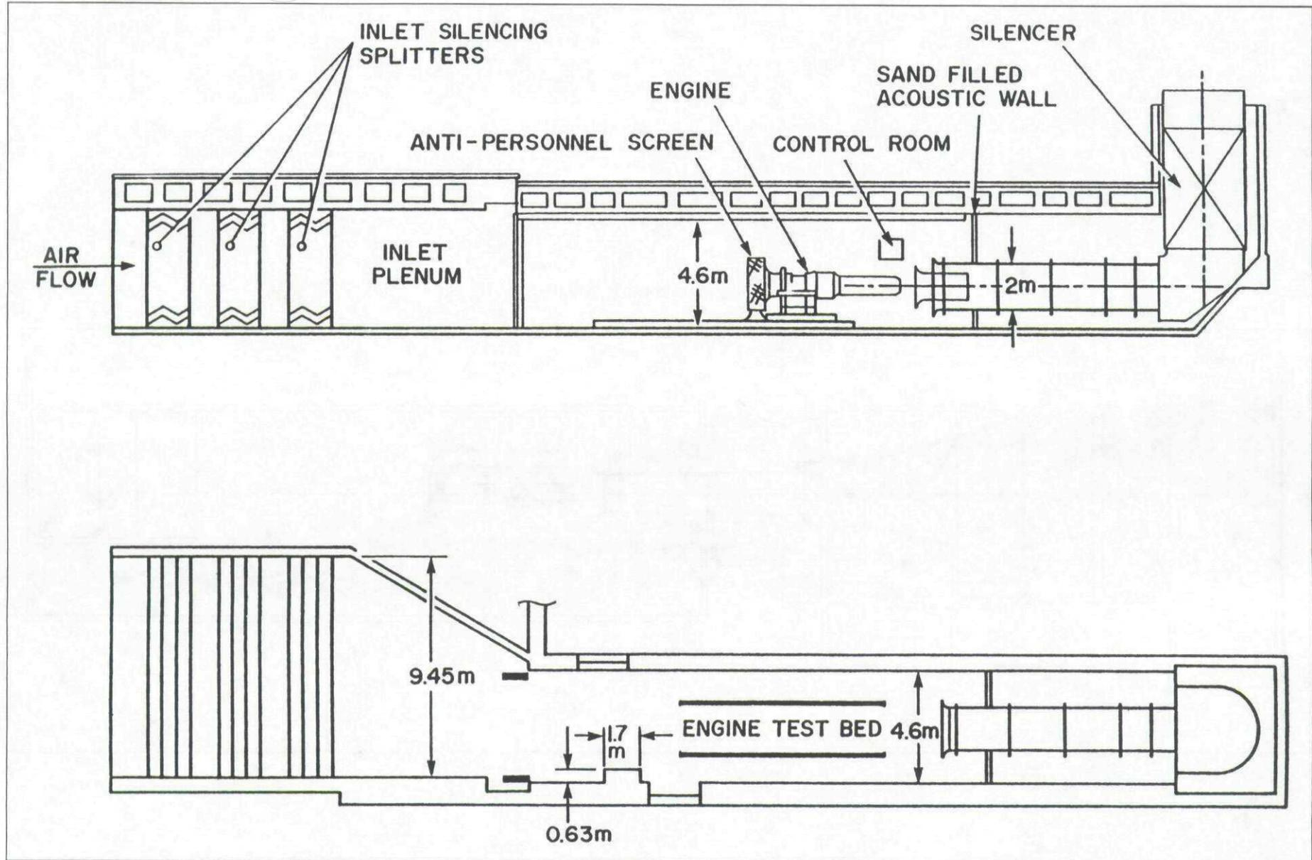
Fig.A No.5 test cell — engine laboratory — NRCC
