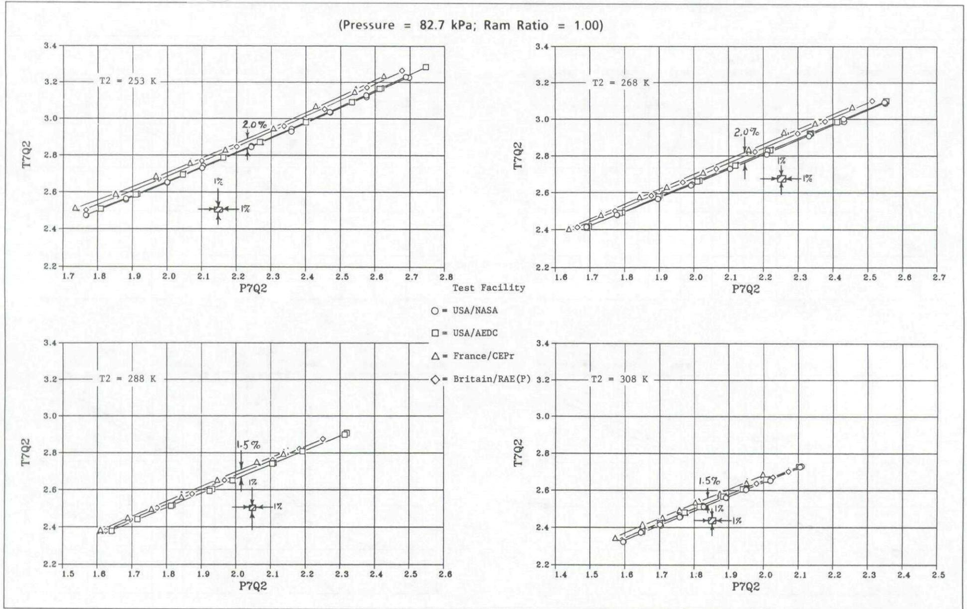
Fig.9-1b Altitude facility temperature rise comparison with variable inlet temperature (engine 607954)
