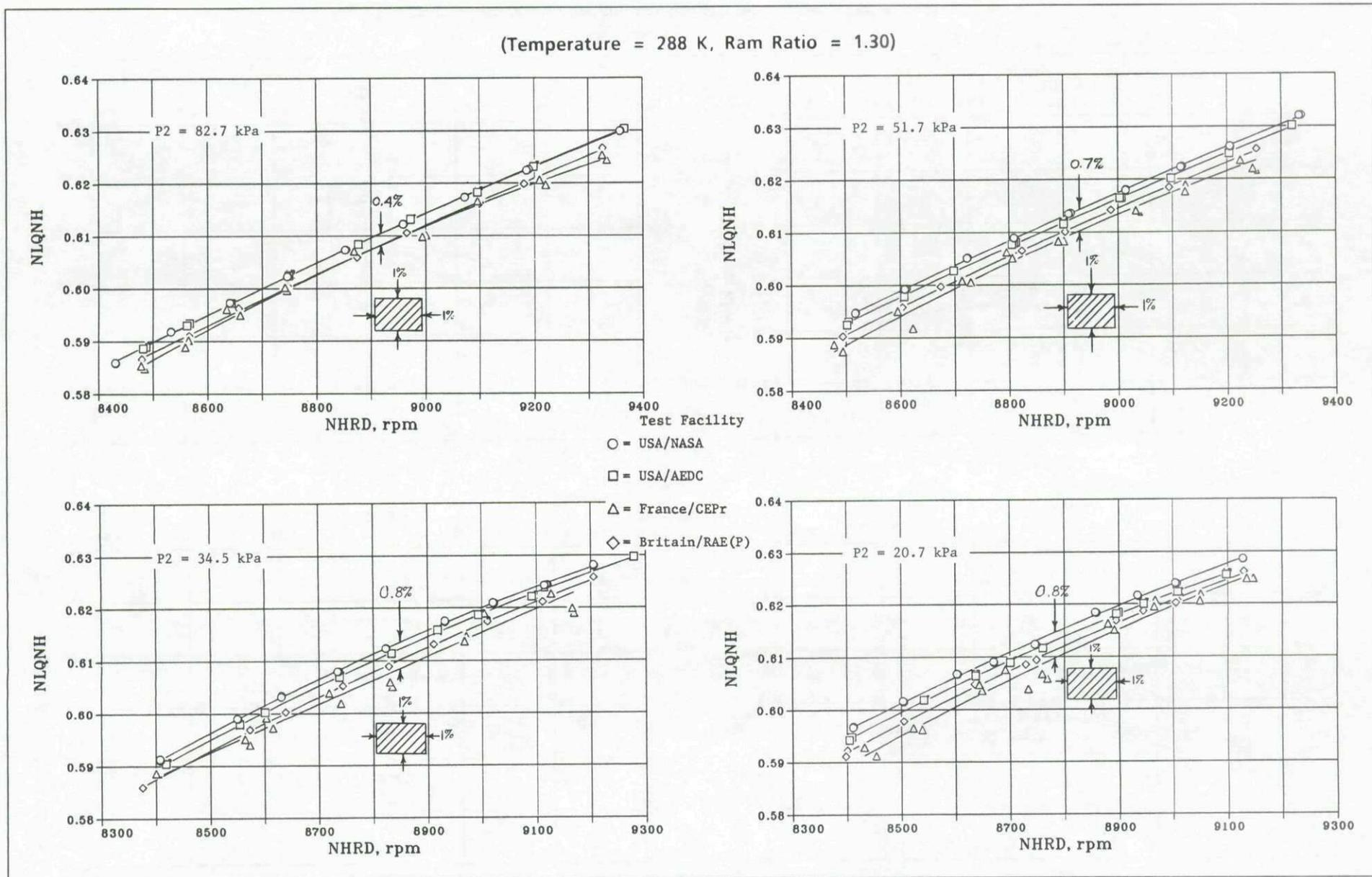
Fig.9-2a Altitude facility speed match comparison with variable inlet pressure (engine 607954)
