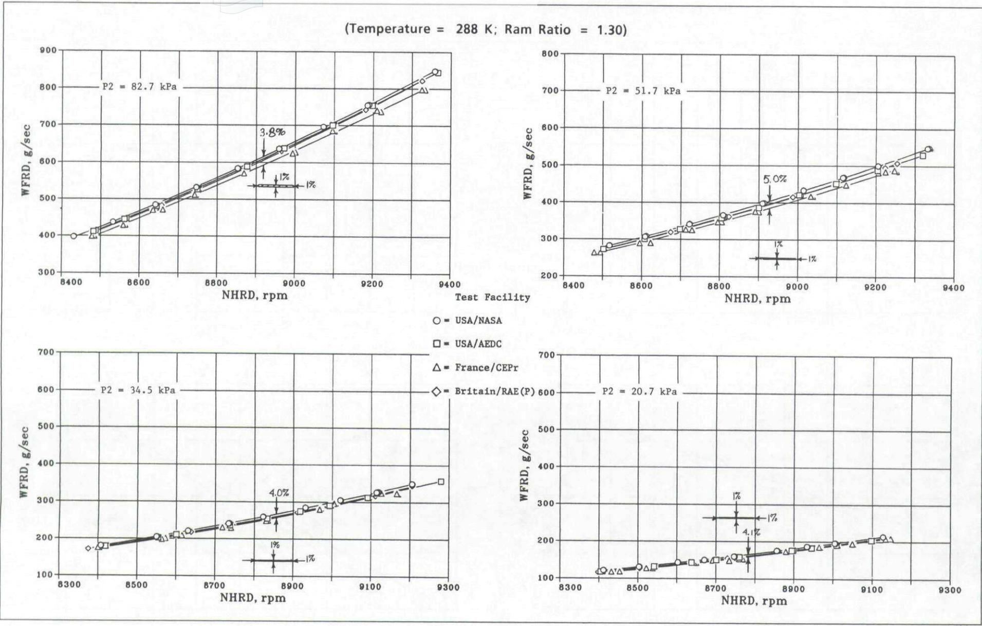
Fig.9-2d Altitude facility fuel flow comparison with variable inlet pressure (engine 607954)
