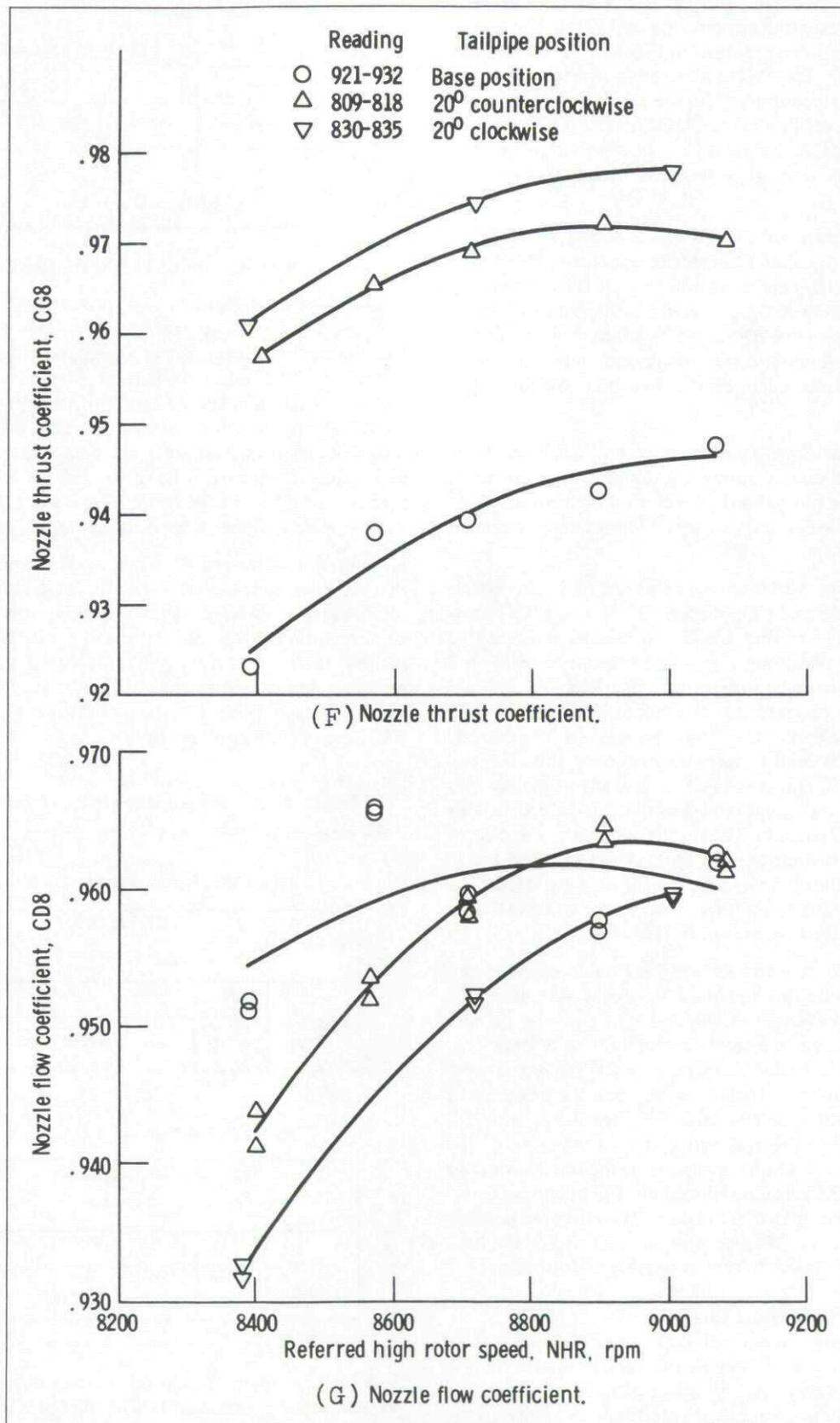
Fig.17-2F&G Effect of tailpipe rotation on thrust and flow (TC9-607594)
