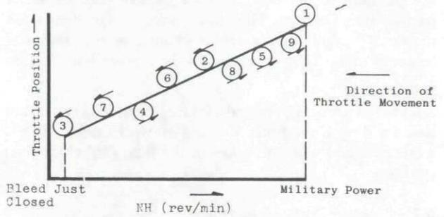
When approaching each setting the throttle lever was moved slowly towards the throttle position where the required speed was expected to be achieved and the engine allowed to stabilise. The set speed had to be within  $\pm 25$  rev/min of the desired. In going between two set speeds, the throttle direction was not allowed to change. In the event of a speed overshoot outside the tolerance band, the throttle setting was backed off approximately 100 rev/min and the speed reset.
