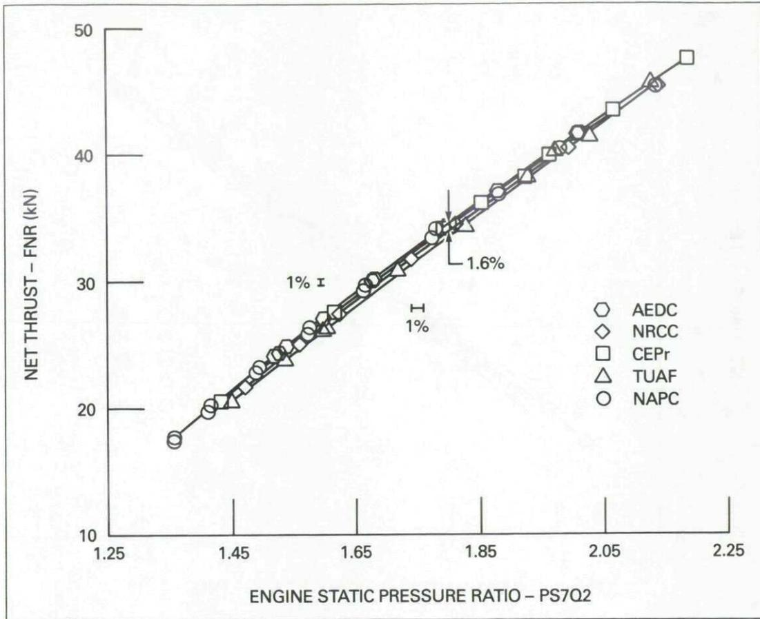
Fig.10 Net thrust as defined by GTP equations
