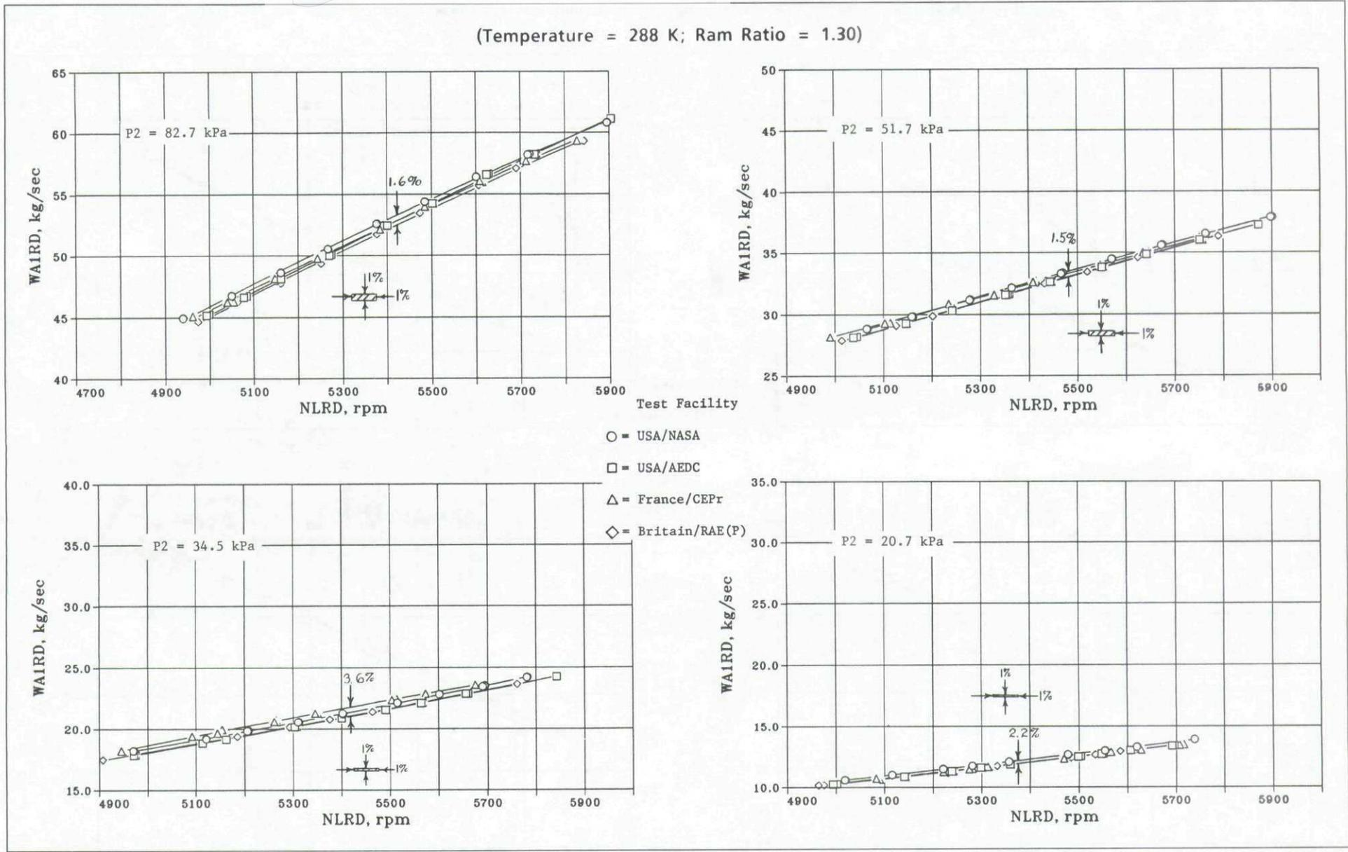
Fig.9-2c Altitude facility airflow comparison with variable inlet pressure (engine 607954)
