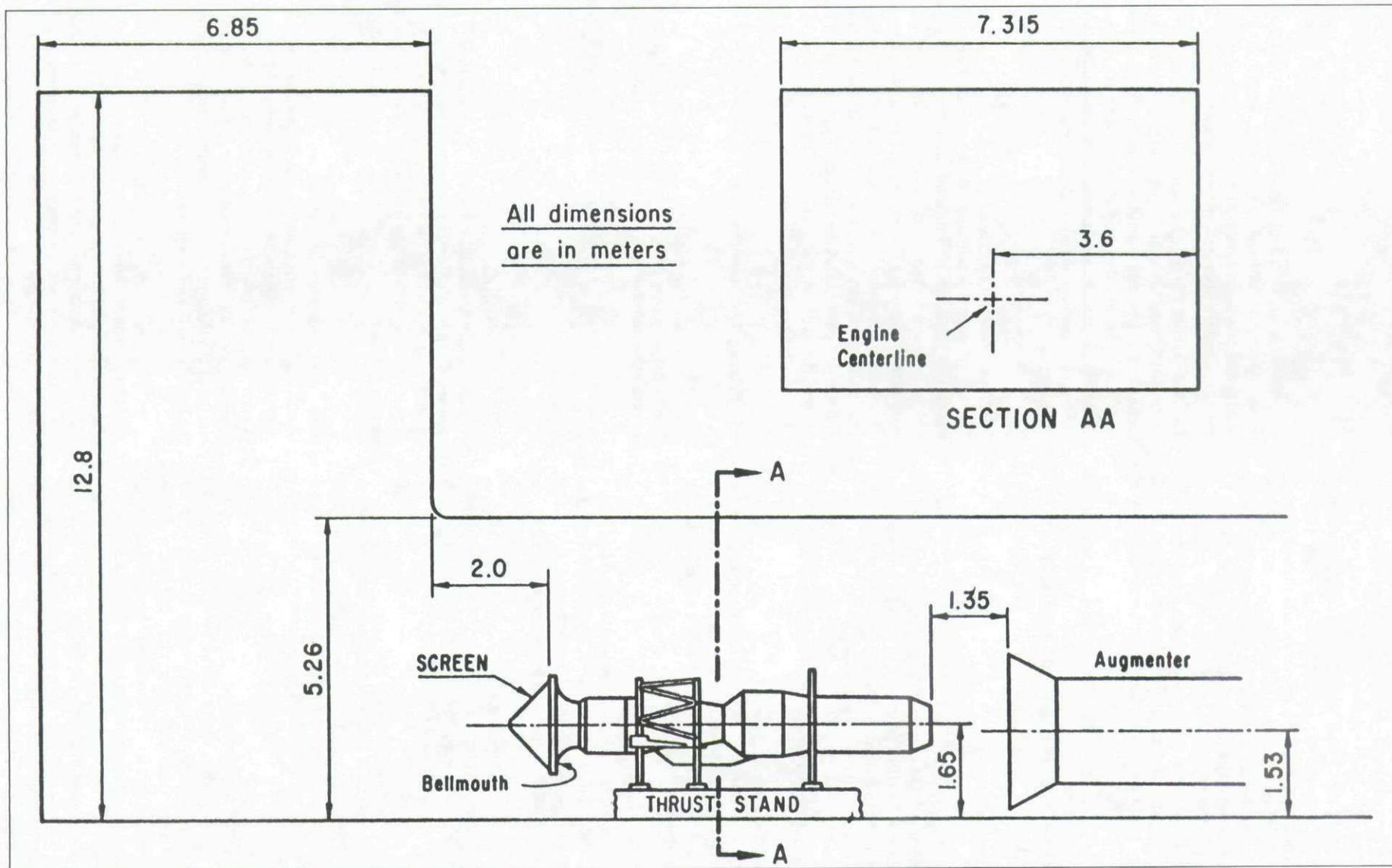
Fig.C Test cell at supply and maintenance centre, Eskisehir, Turkey (TUAF)
