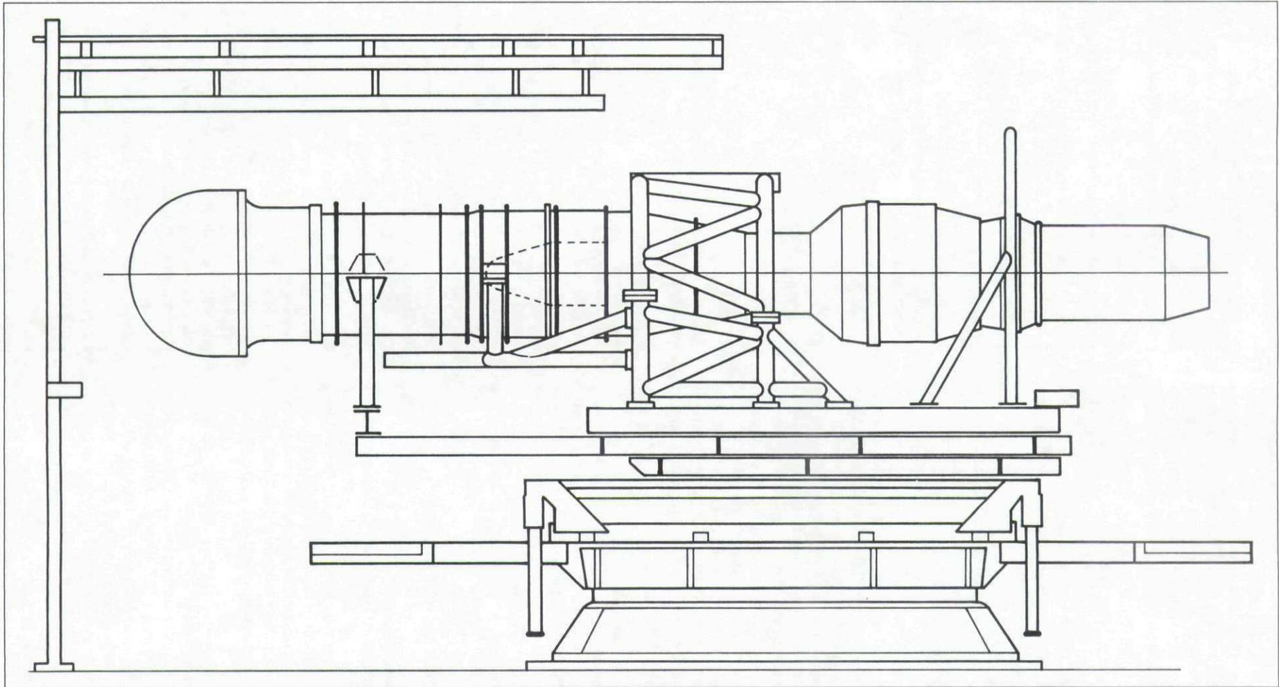
Fig.1 Engine installation at NAPC outdoor test site
