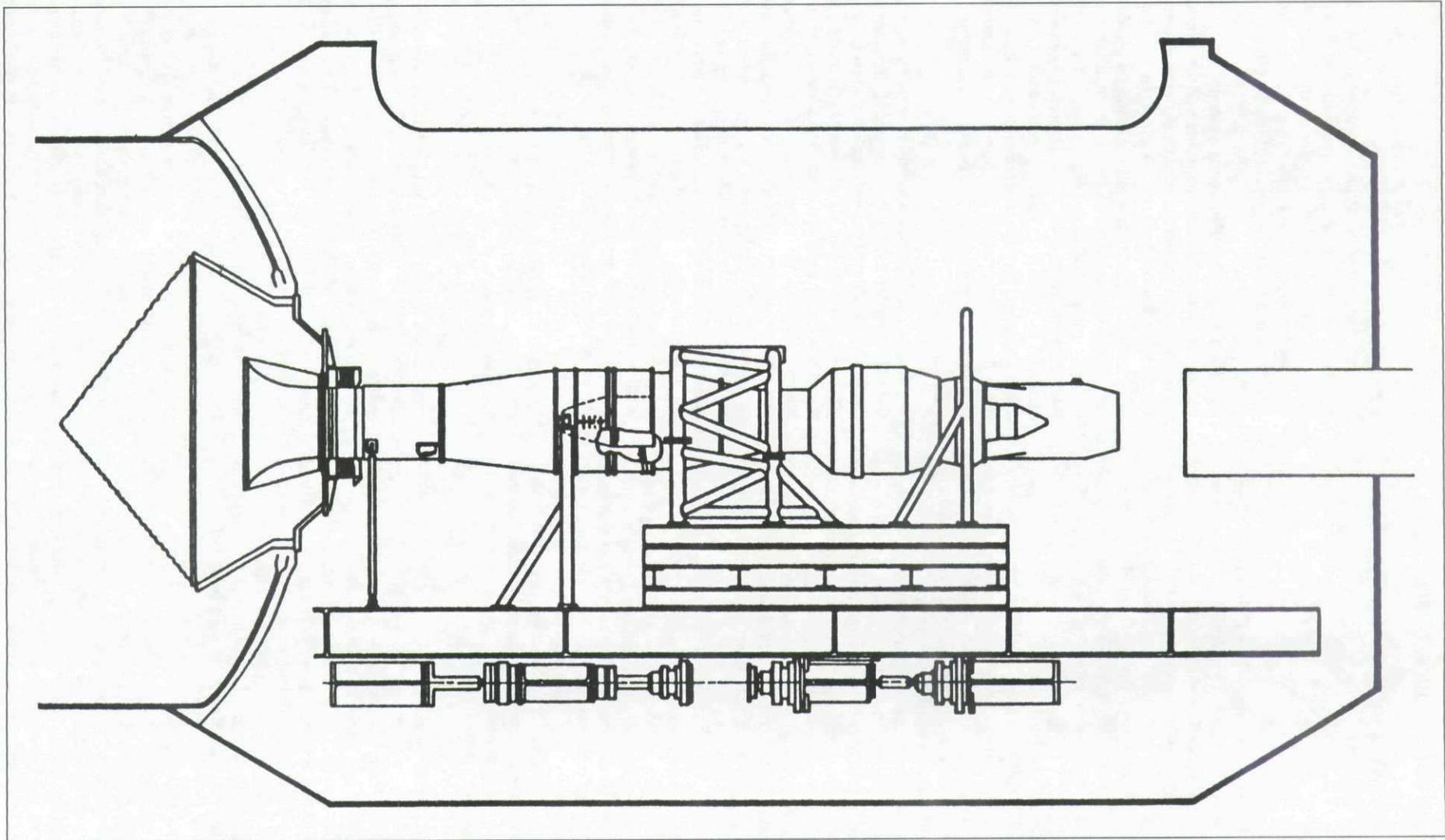
Fig.D J57 engine installed in NASA high altitude test cell PSL-3
