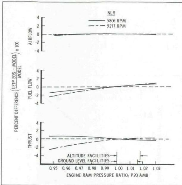
Fig.16-2 Comparison of UETP and engine model sea level temperature correction factors
