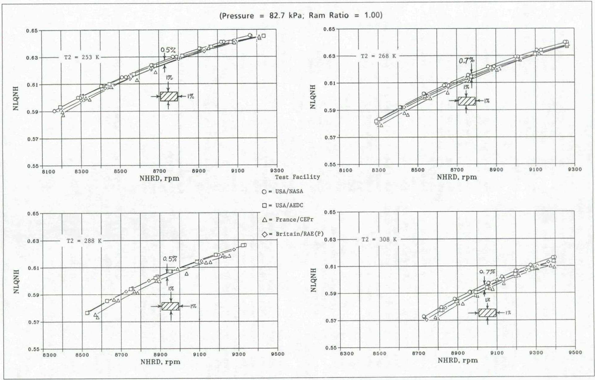
Fig.9-1a Altitude facility speed match comparison with variable inlet temperature (engine 607954)
