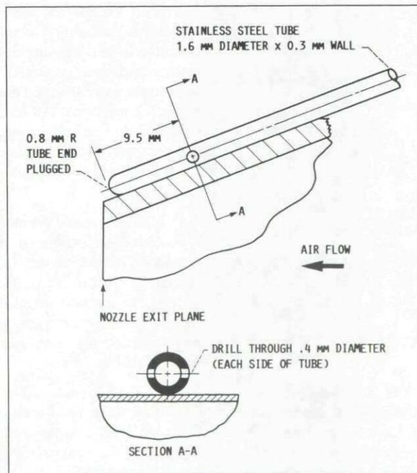
Fig.4-4 Nozzle exit lip static pressure probes
