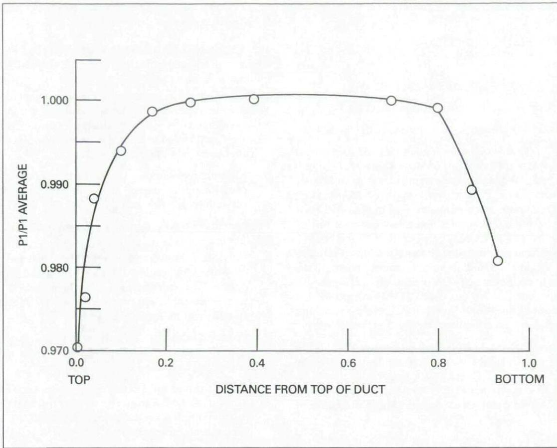
Fig.2 Station 1 inlet total pressure profile — military power
