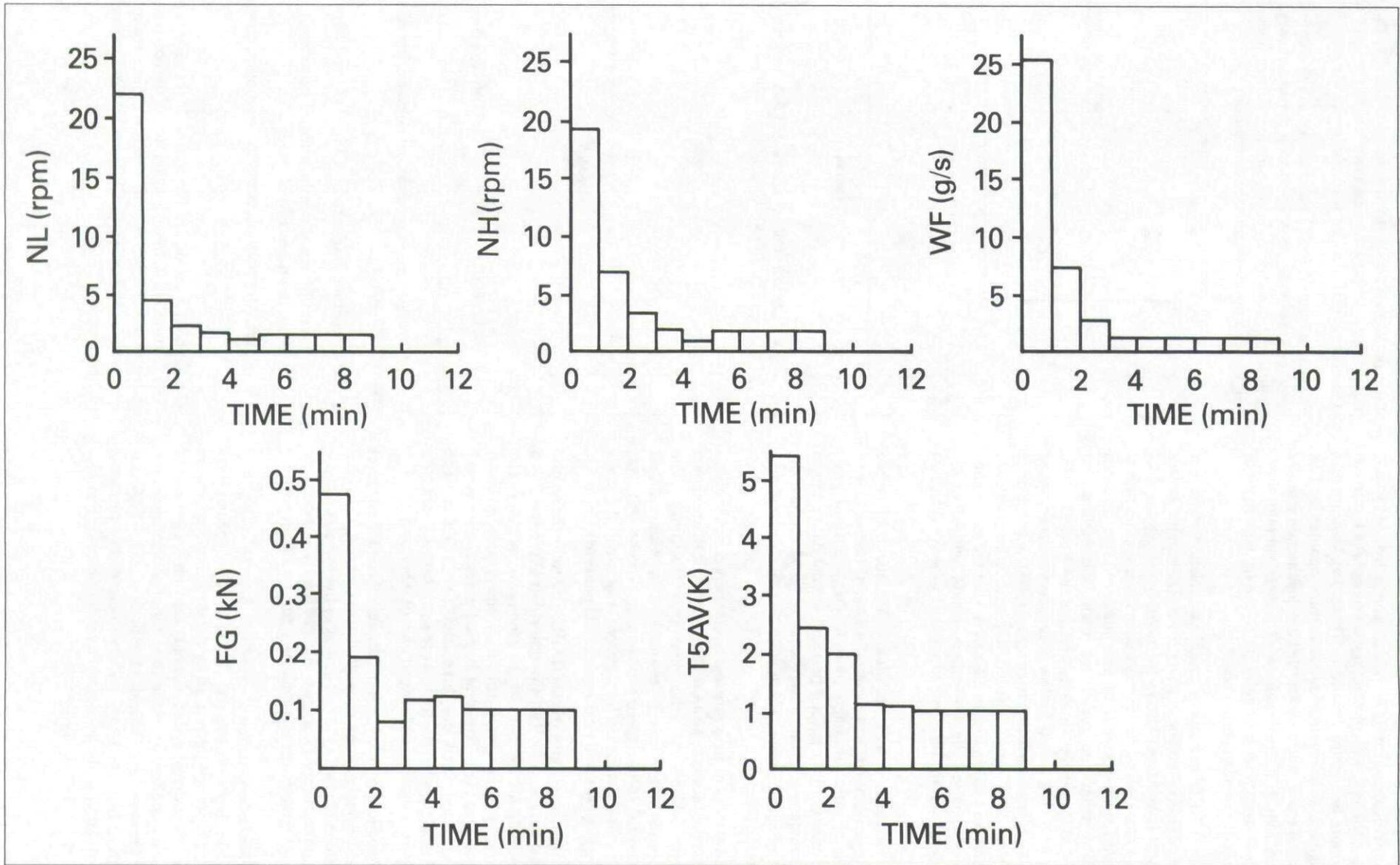
Fig.12-5 The standard deviation from the mean for several parameters as a function of engine settling time in the NRCC ground level facility
