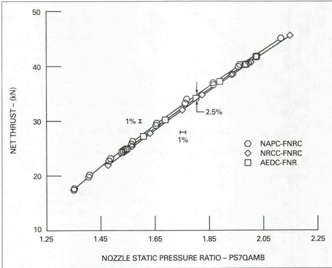
Fig.14 Net thrust vs. nozzle static pressure ratio
