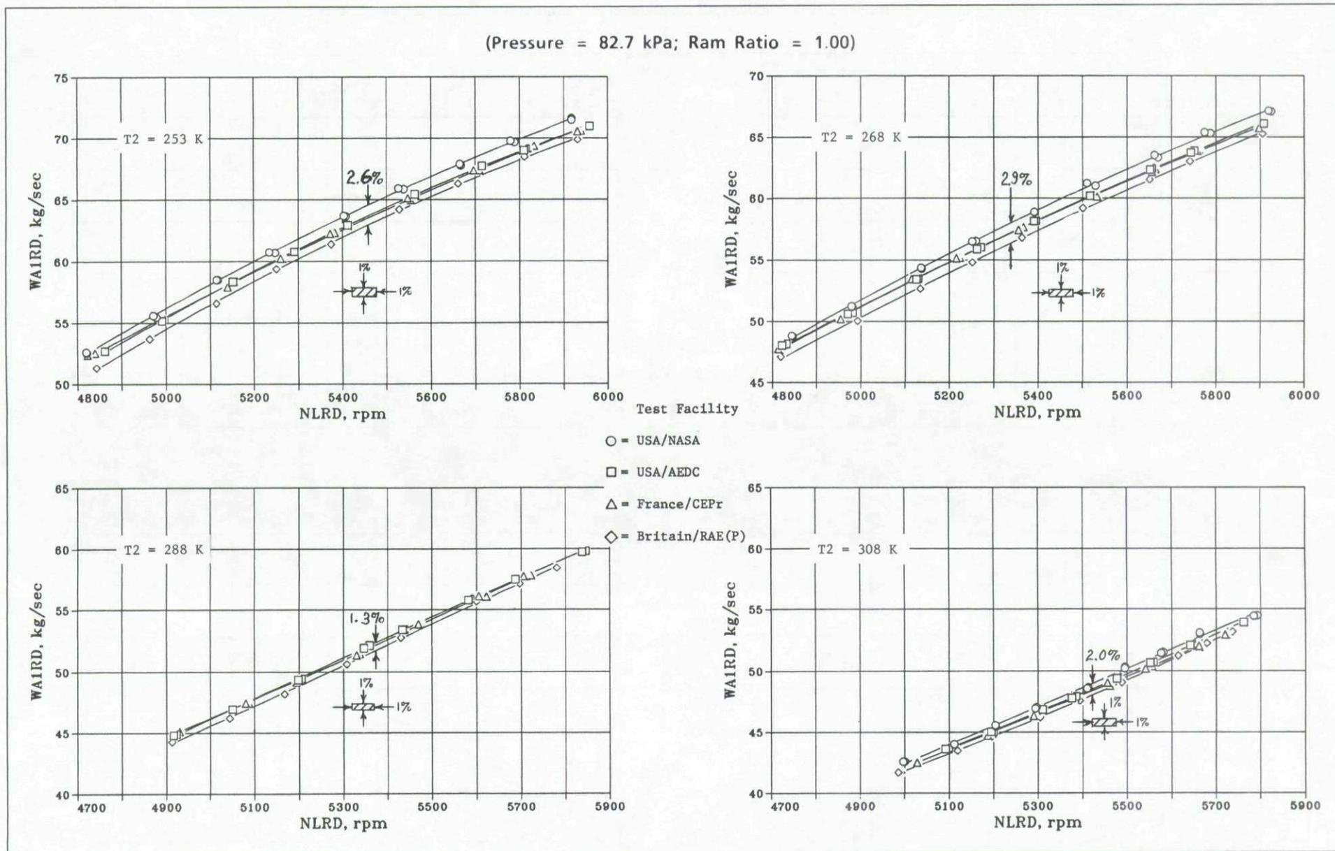
Fig.9-1c Altitude facility airflow comparison with variable inlet temperature (engine 607954)
