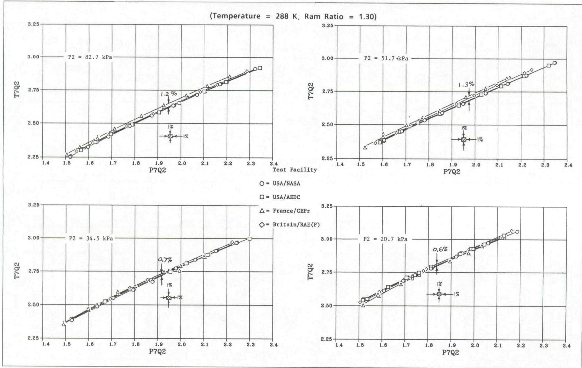
Fig.9-2b Altitude facility temperature rise comparison with variable inlet pressure (engine 607954)
