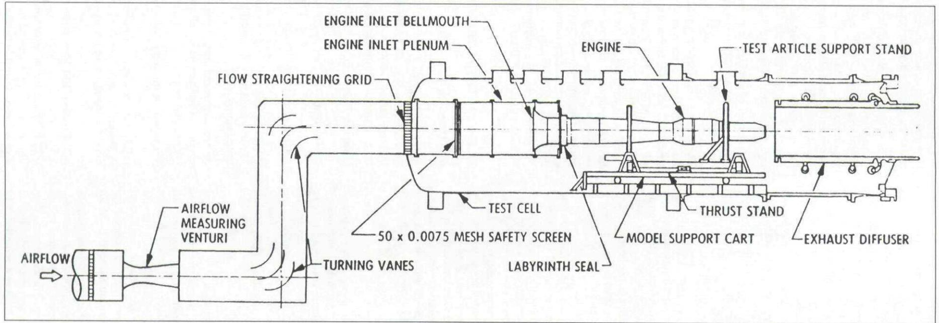
Fig.E J57 engine installed in AEDC propulsion development test cell T-2
