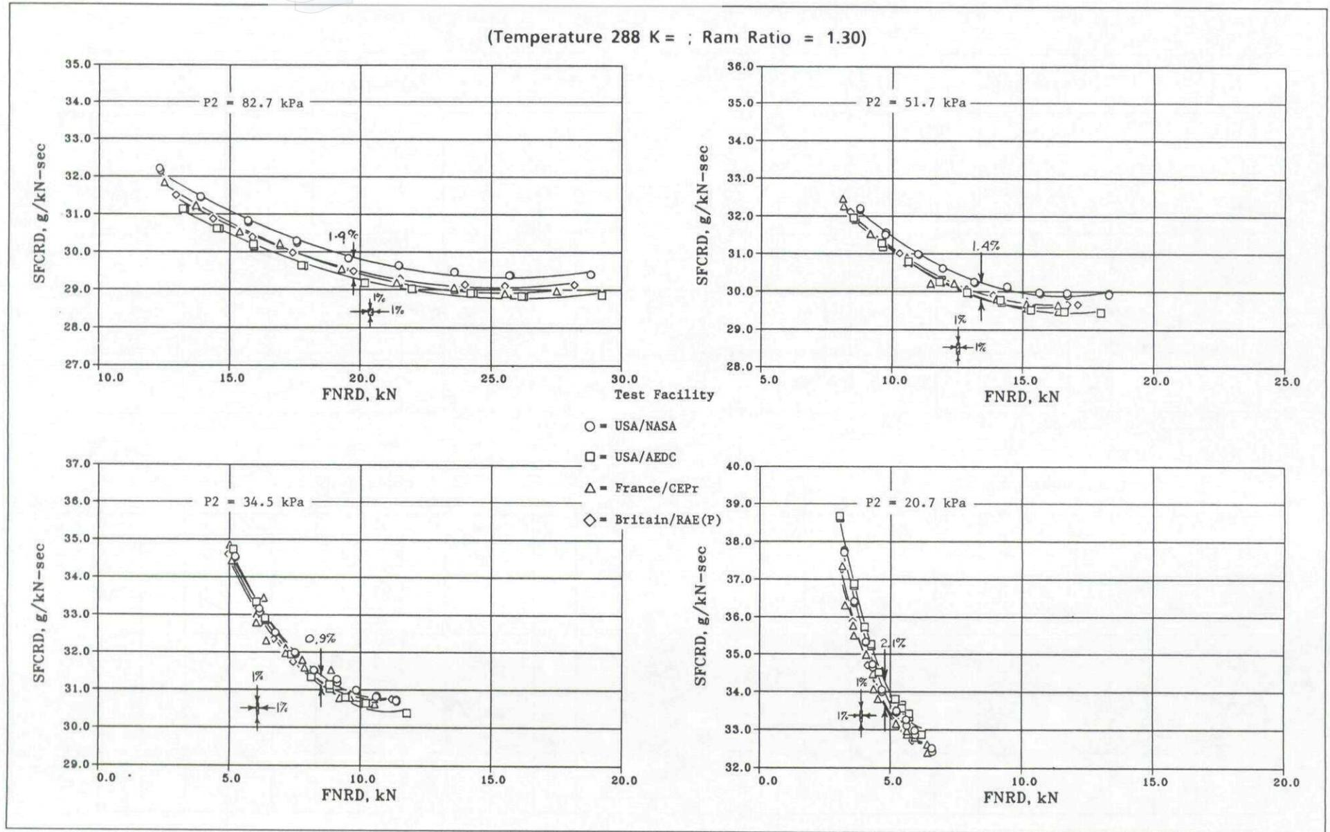
Fig.9-2f Altitude facility specific fuel consumption comparison with variable inlet pressure (engine 607954)
