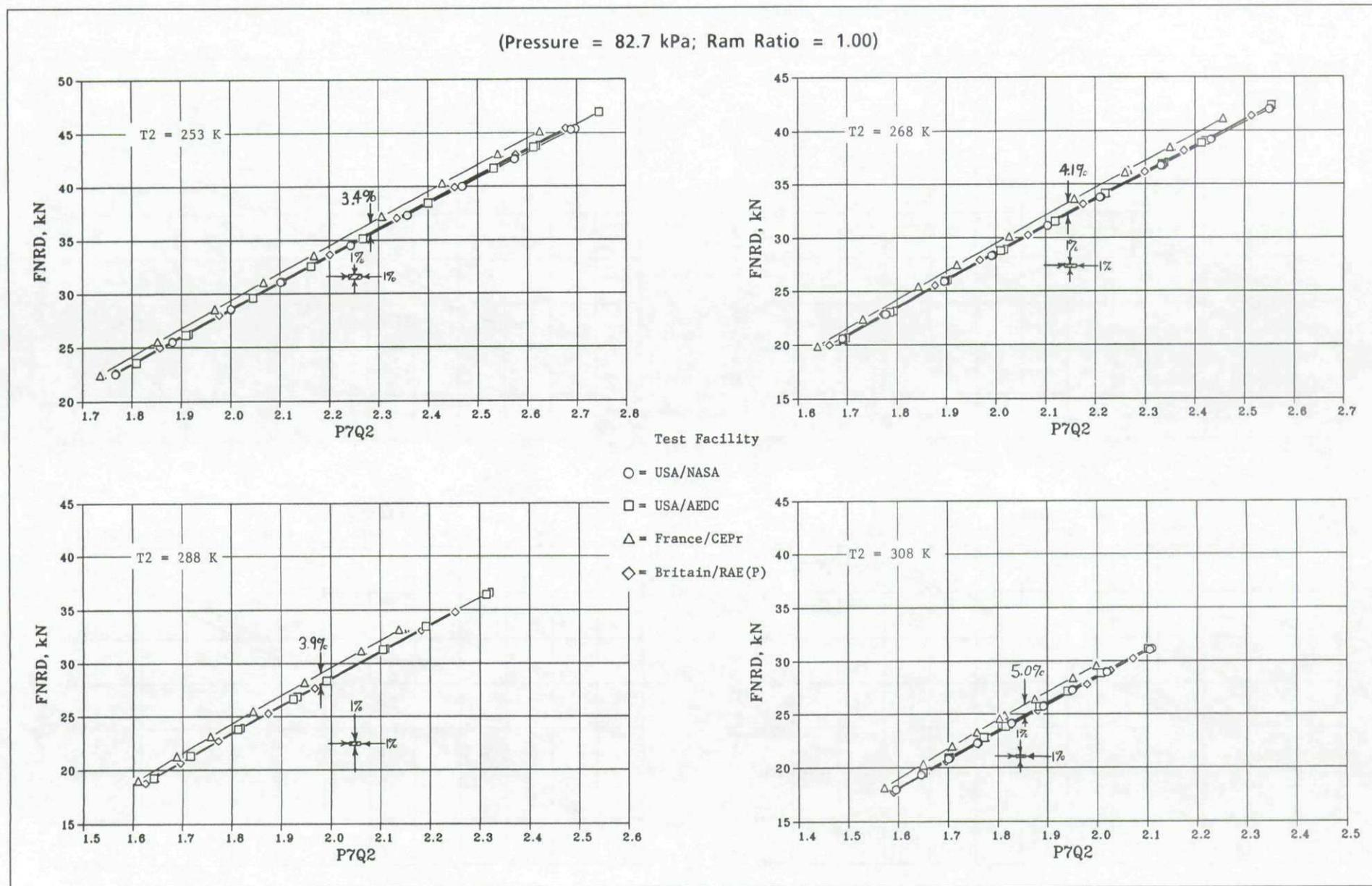
Fig.9-1e Altitude facility net thrust comparison with variable inlet temperature (engine 607954)
