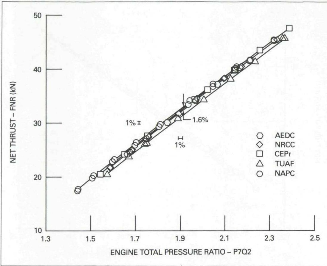
Fig.8 Net thrust vs. engine pressure ratio
