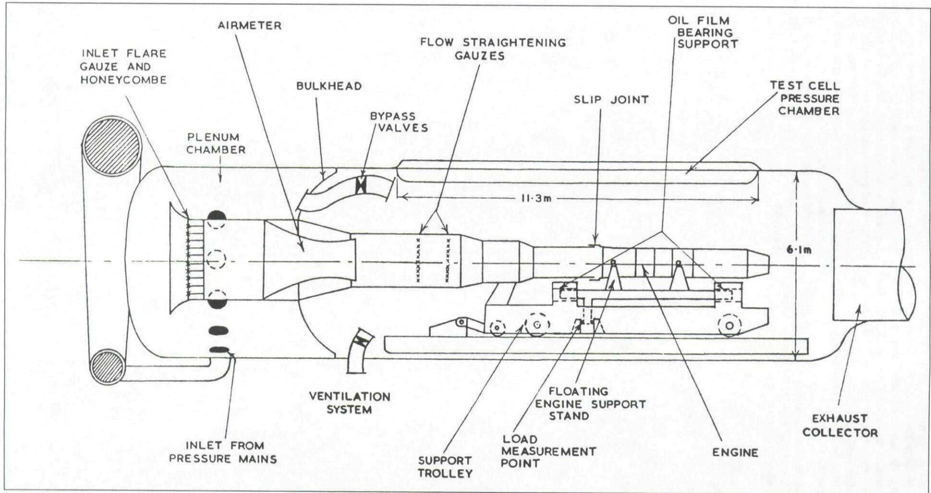
Fig.G Typical engine installation in RAE(P) altitude cell 3
