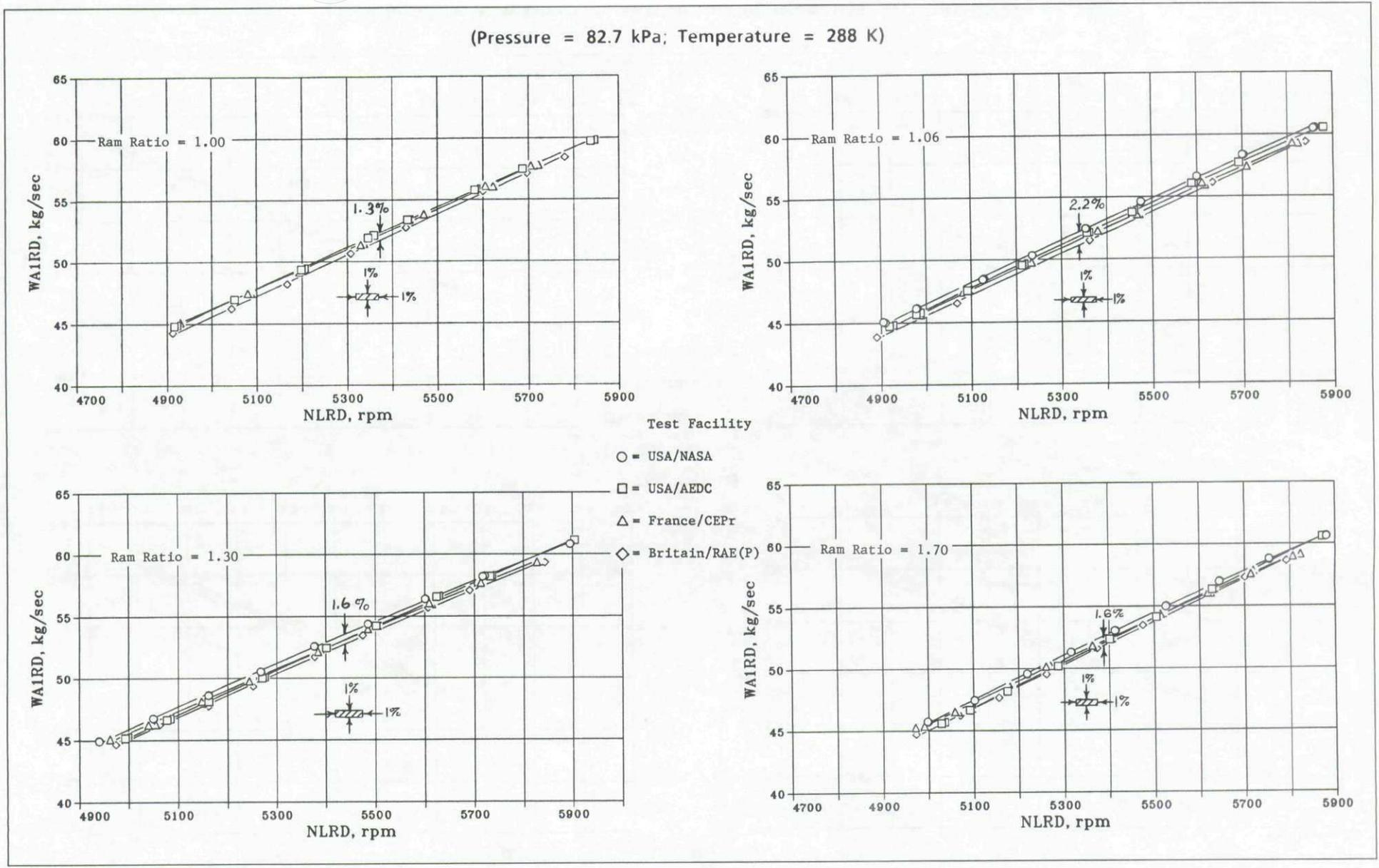
Fig.9-3c Altitude facility airflow comparison with variable RAM ratio (engine 607954)
