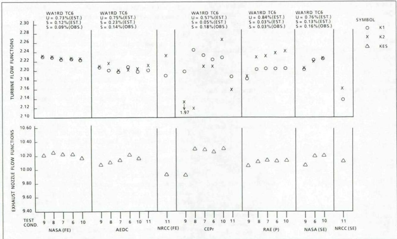
Fig.14-1 Variation of turbine and exhaust nozzle flow coefficients (engine 607594)
