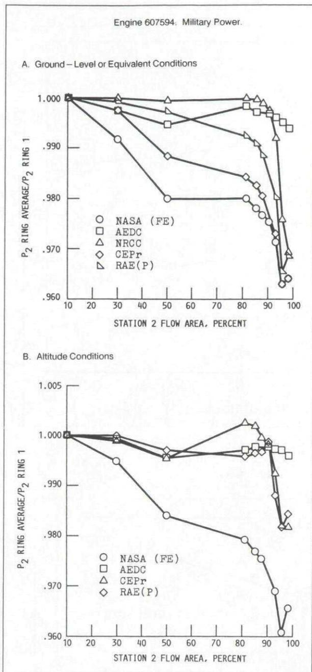
Fig.12-1 Comparison of inlet total pressure profiles
