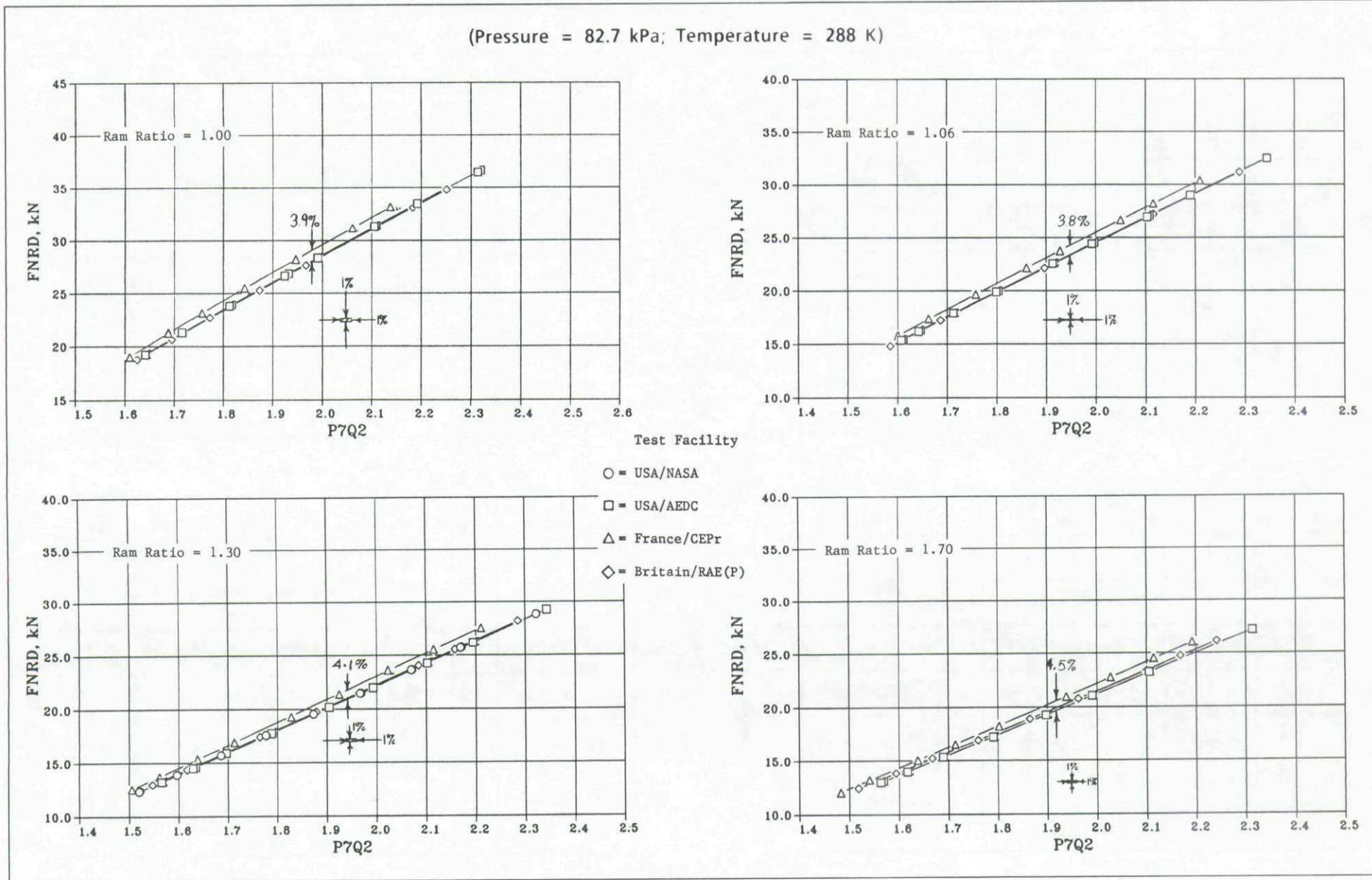
Fig.9-3e Altitude facility net thrust comparison with variable RAM ratio (engine 607954)
