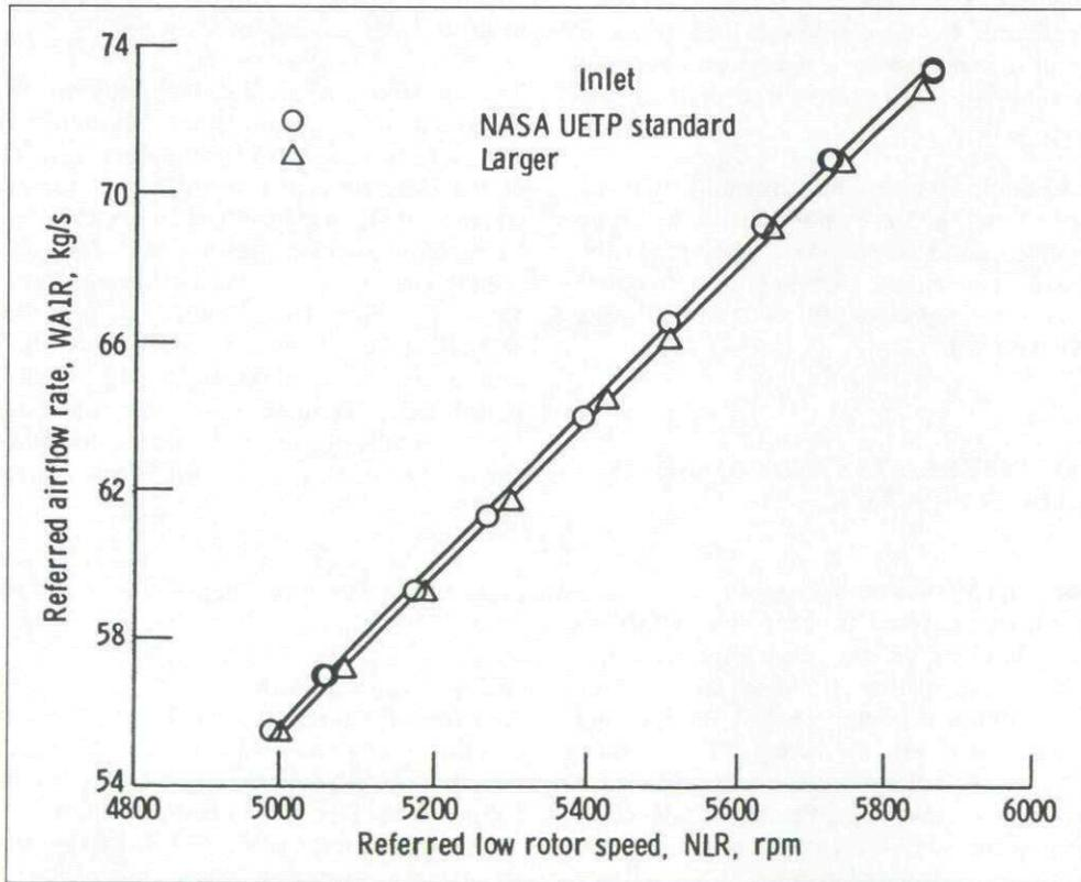
Fig.17-3B Effect of inlet duct on airflow (TC 6)
