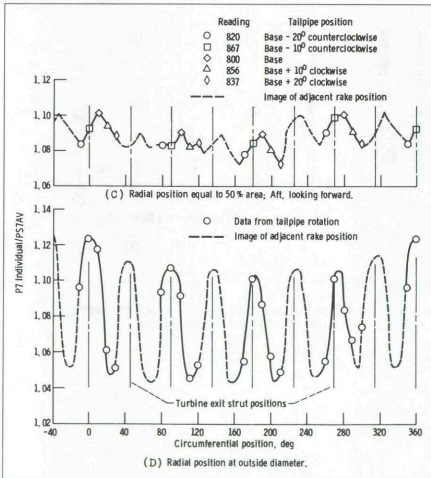
Fig.17-2C&D Total pressure variation with tailpipe rotation
