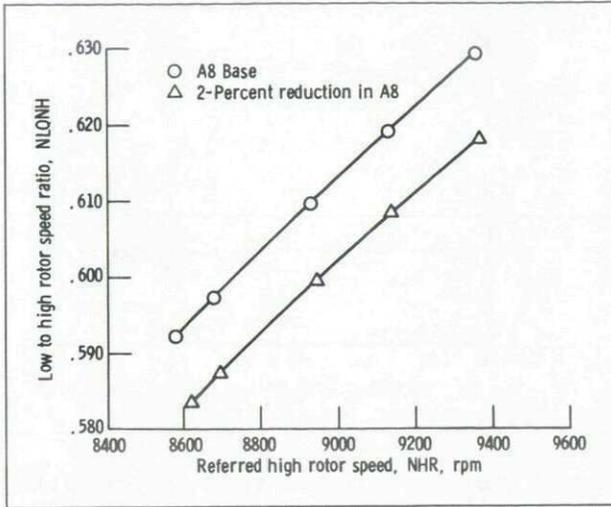
Fig.17-1A Effect of exhaust nozzle area on speed ratio (TC6-607594)
