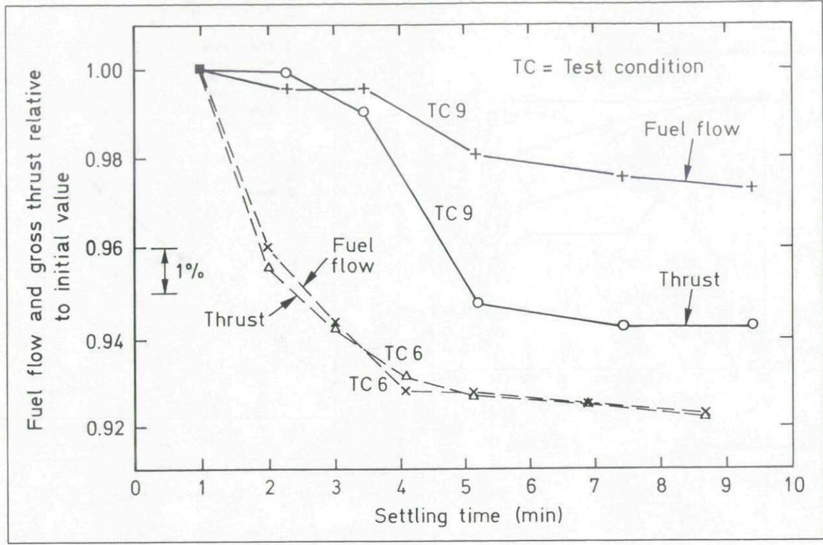
Fig.12-3 Fuel flow and thrust during stabilisation time
