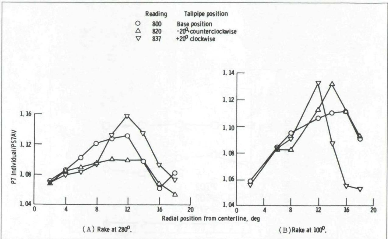
Fig.17-2A&B Station 7 radial total pressure profiles
