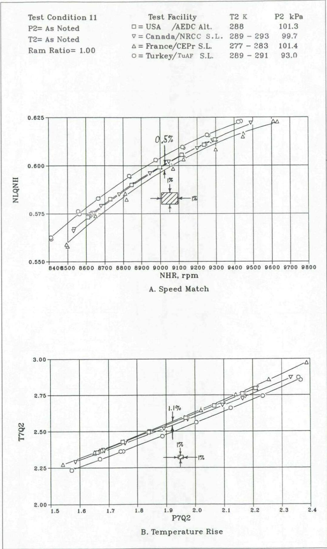
Fig.9-4 Ground level test facility comparison (engine 615037)
