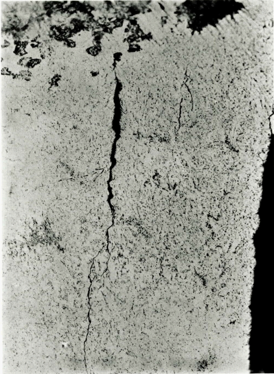
Fig.7 Optical photomicrograph of subsidiary fatigue crack under scar. (Taper section 1:10, magnification x 200)
