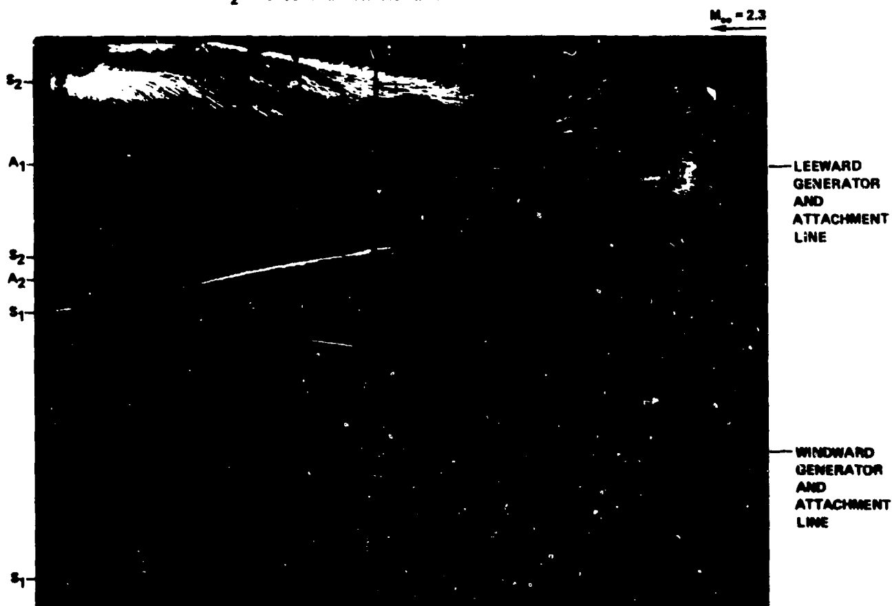
(b) UNWRAPPED SURFACE OF CYLINDRICAL AFTERBODY, R_{L_{\infty}} \sim 10 \times 10^6 , R_D = 1.3 \times 10^6
