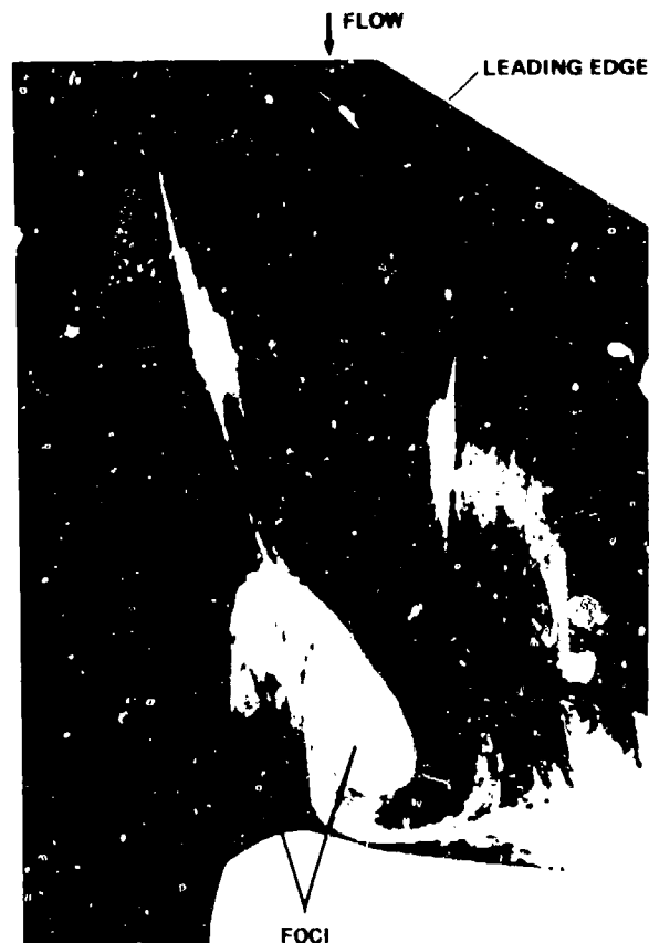
(d) TURBULENT FLOW ON INBOARD TRAILING-EDGE REGION OF LIFTING HIGH ASPECT RATIO SWEEP WING OF TRANSPORT AIRCRAFT AT HIGH SUBSONIC SPEED (COURTESY OF B. ELSENAAR, NLR)
