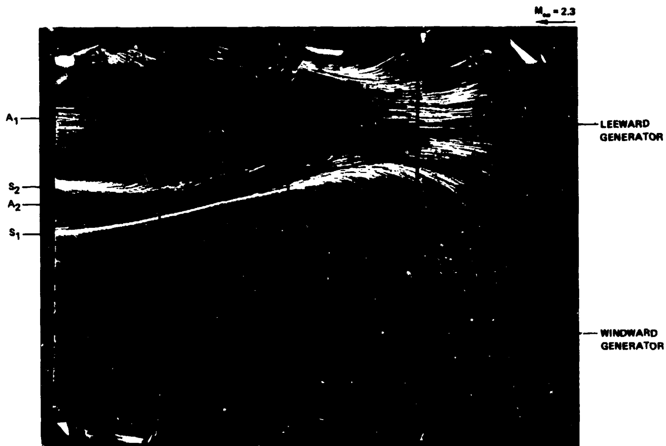
(c) UNWRAPPED SURFACE OF CYLINDRICAL AFTERBODY, R_{L_\infty} \sim 30 \times 10^6 , R_D = 4 \times 10^6
