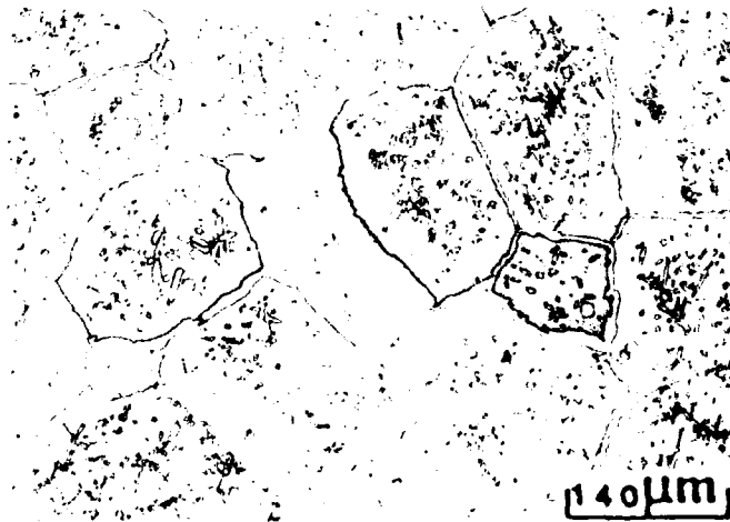
Figure 5. Microstructure of Ni-36 wt% Al (Number 13) After Heat Treatment at (a) 1200°C (2130°F) for 4 hours, cooling at 140°C (270°F) per hour, air cooling; (b) 1400°C (2550°F) for 64 hr, air cooling; (c) 1400°C (2550°F) for 64 hr, slow furnace cooling.
