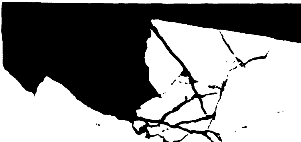
Figure 31. Photomicrograph of Ball Section Through Spall. Numerous Transgranular Cracks Emanated From Apparent Spall Origin.
