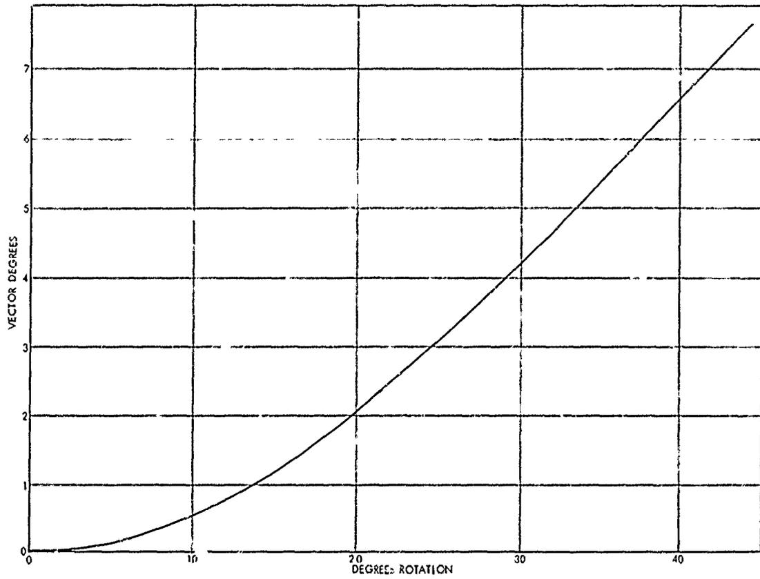
Figure 7-3. Thrust Vector vs. Shaft Rotation
