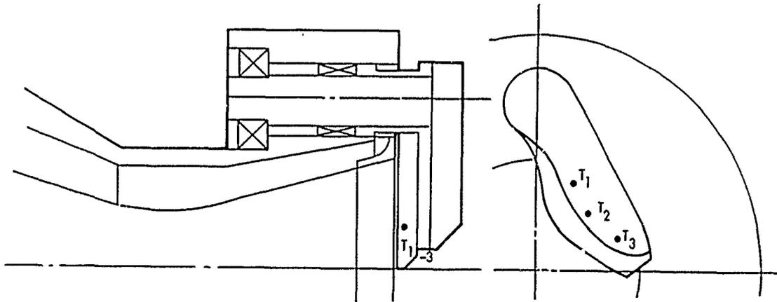
Figure 8-3. Thermocouple Location
