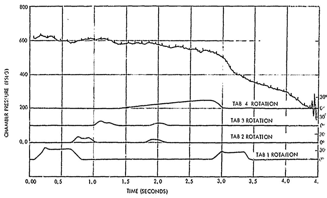
Figure 5-4. Motor Chamber Pressure and Tab Actuation, PI-1
