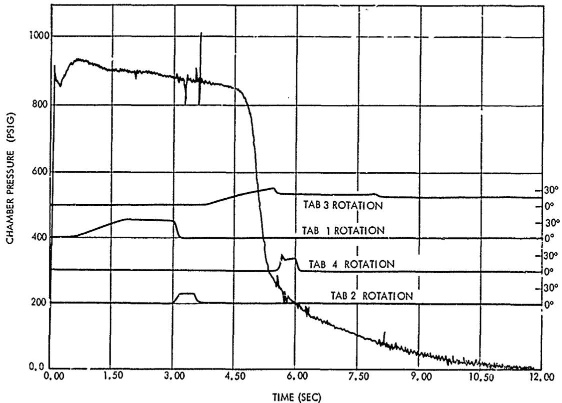
Figure 5-29 Tab Actuation and Motor Chamber Pressure PFRT-04
