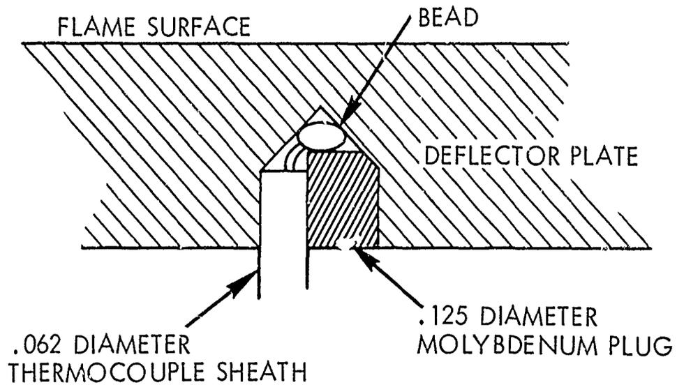
Figure 8-4. Buried Thermocouple
