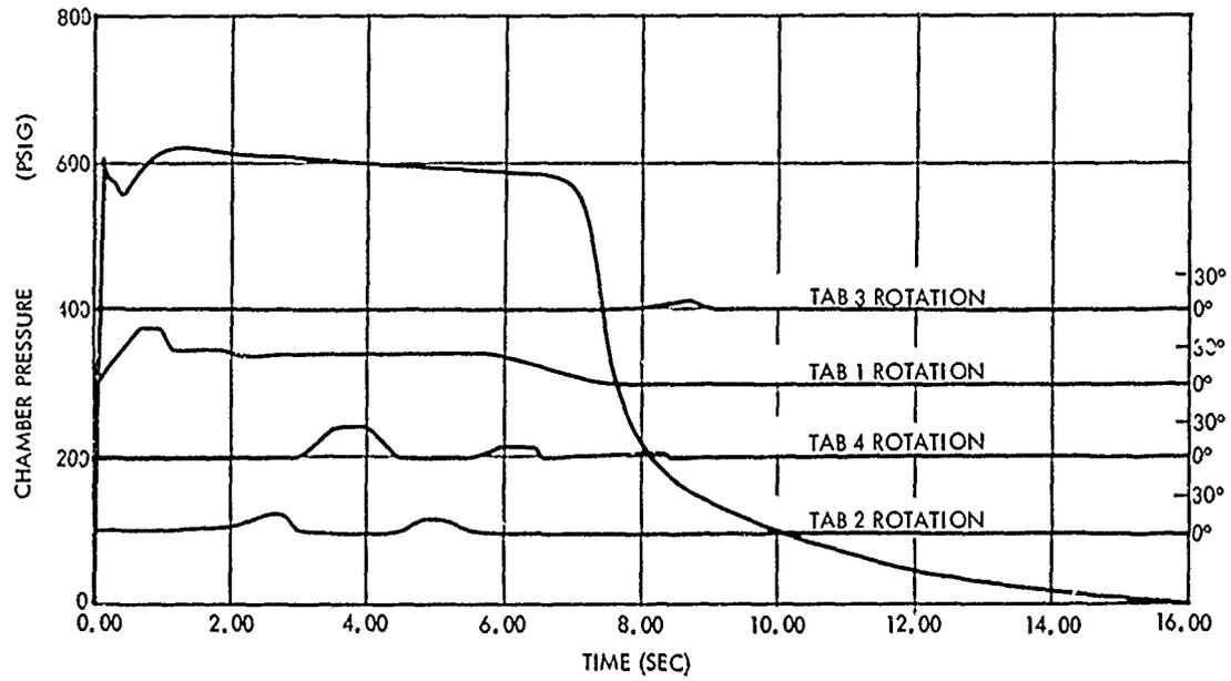
Figure 5-32. Tab Actuation and Motor Chamber Pressure, PFRT-05
