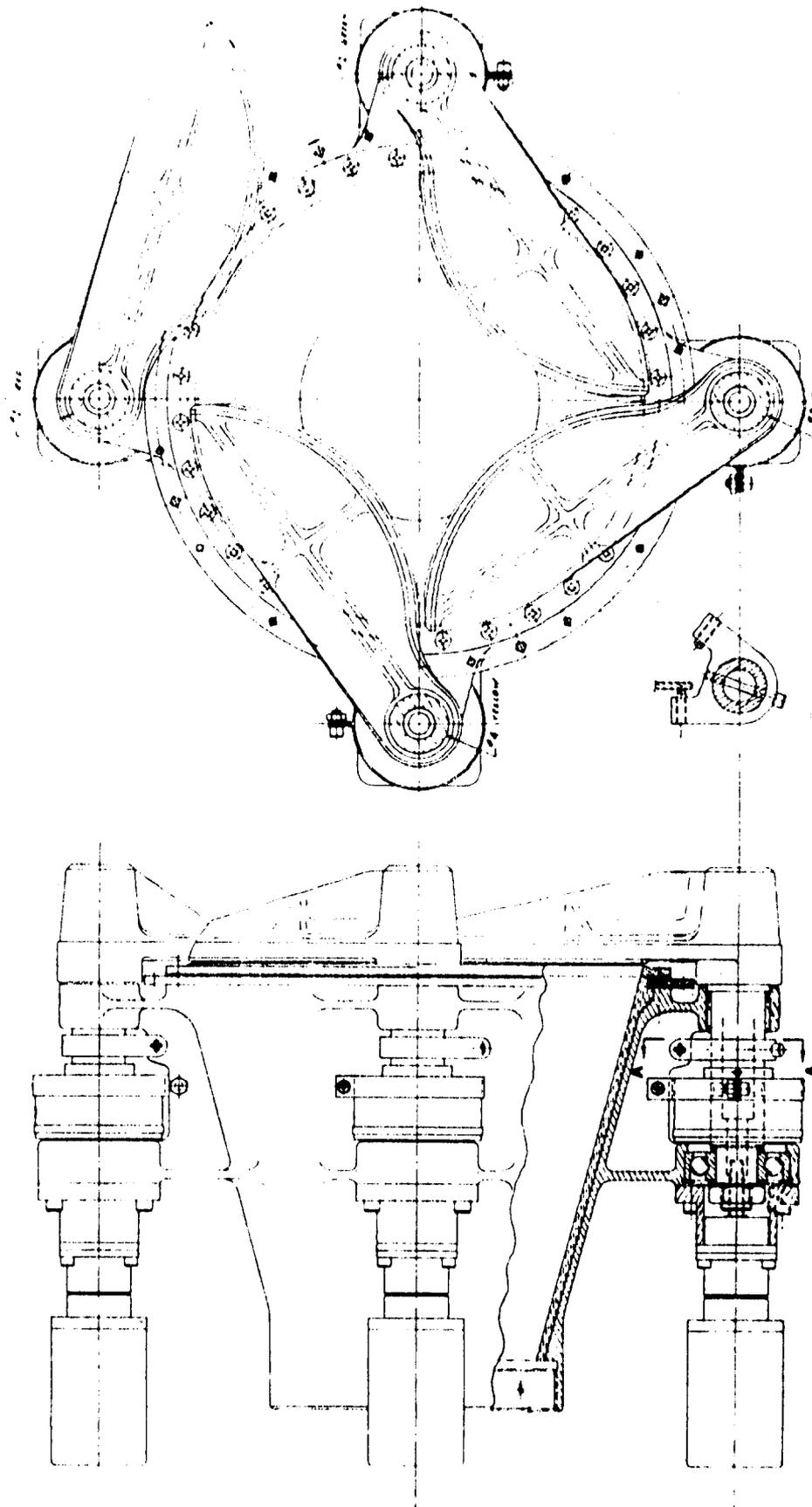
Figure 3-6. Jet Tab TVC System for JBQM-34H Ground Launch
