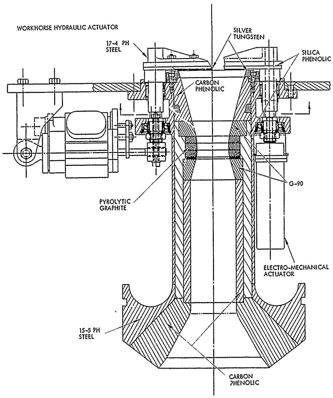
Figure 3-4. HIPPO Motor Jet Tab TVC System
