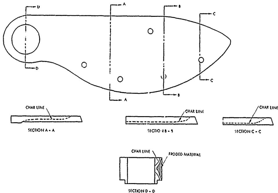
Figure 7-8. Tab Insulator Char Depth
