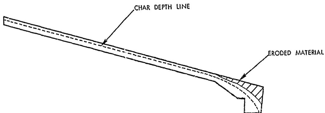
Figure 7-7. Nozzle Liner Char Depth
