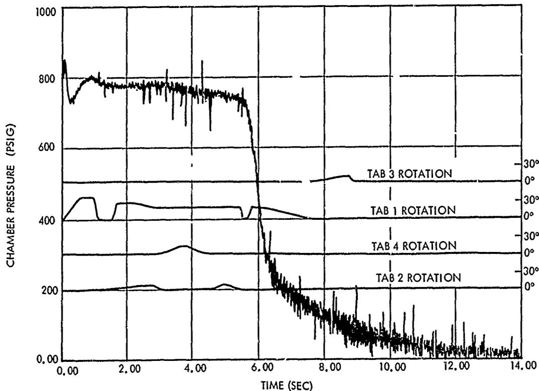
Figure 5-34. Tab Actuation and Motor Chamber Pressure, PFRT-06
