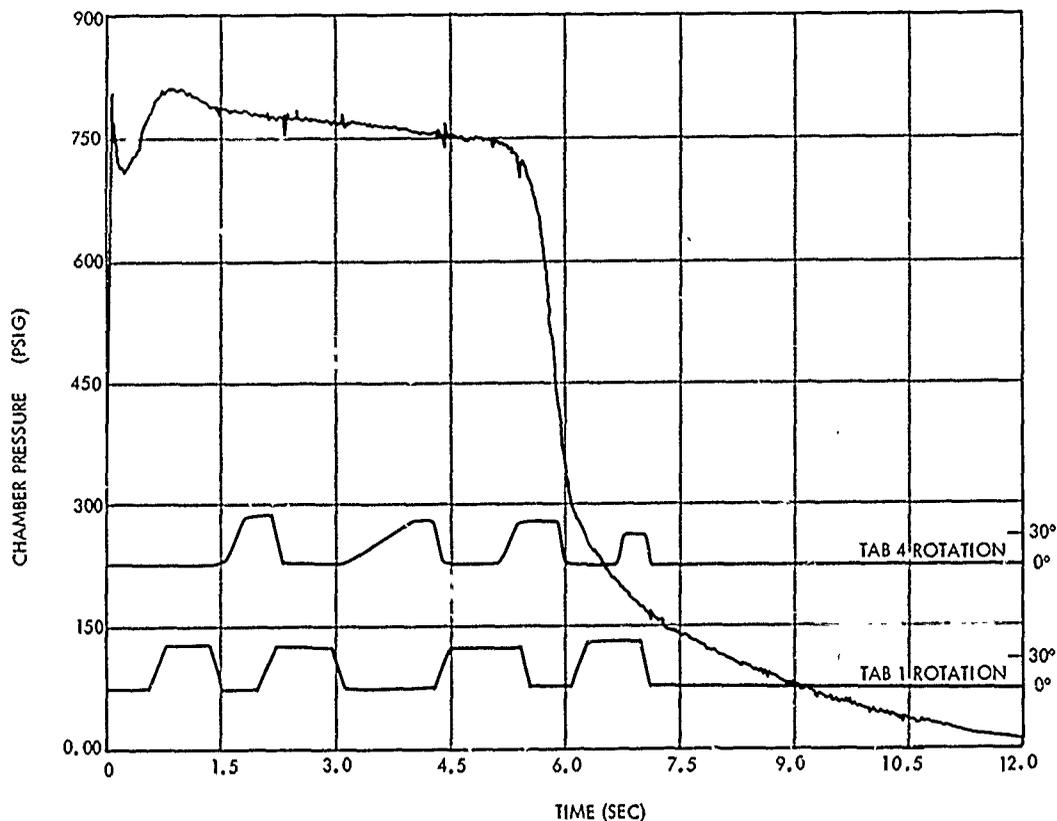
Figure 5-18. Tab Actuation and Motor Chamber Pressure, PFRT-01
