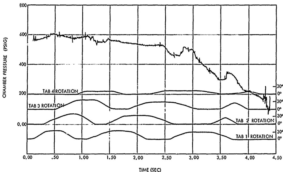
Figure 5-6. Motor Chamber Pressure and Tab Actuation, PI-2
