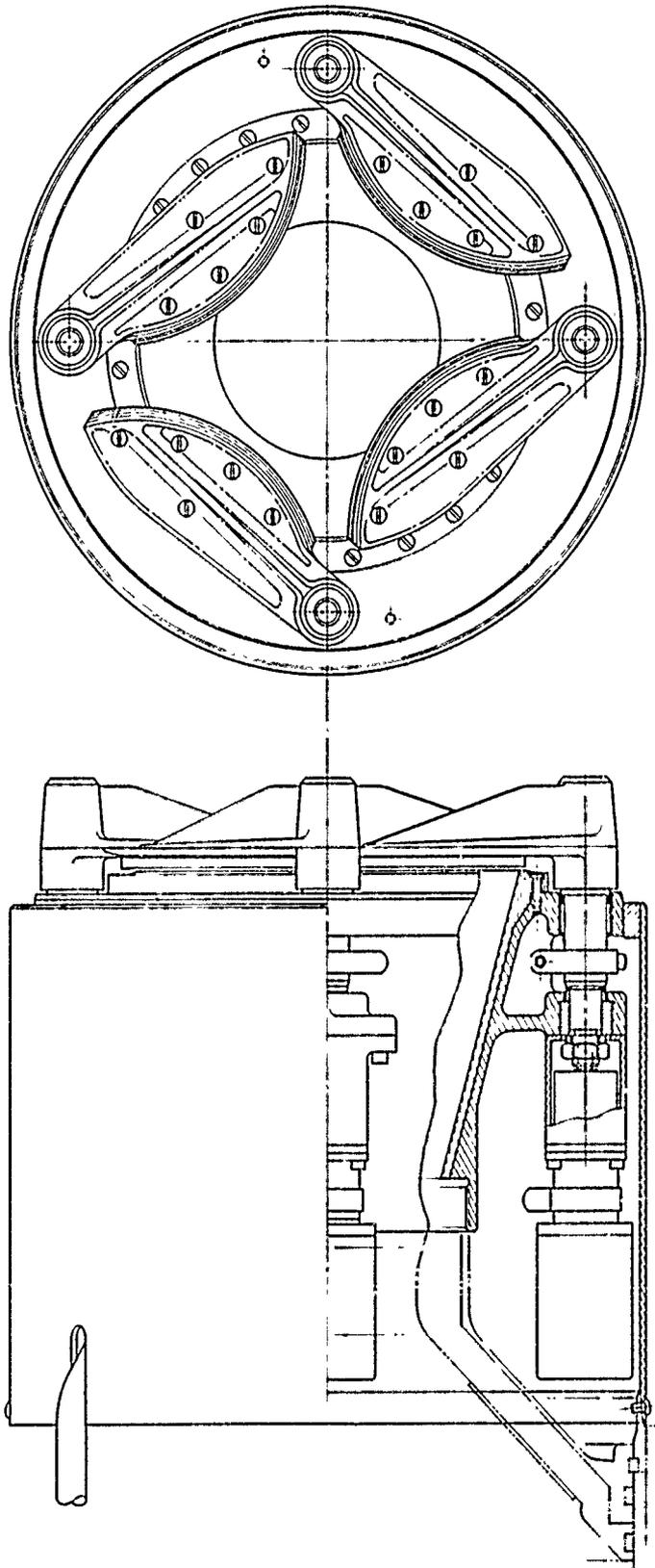
Figure 4-1. Jet Tab TVC System for BGM-34C
