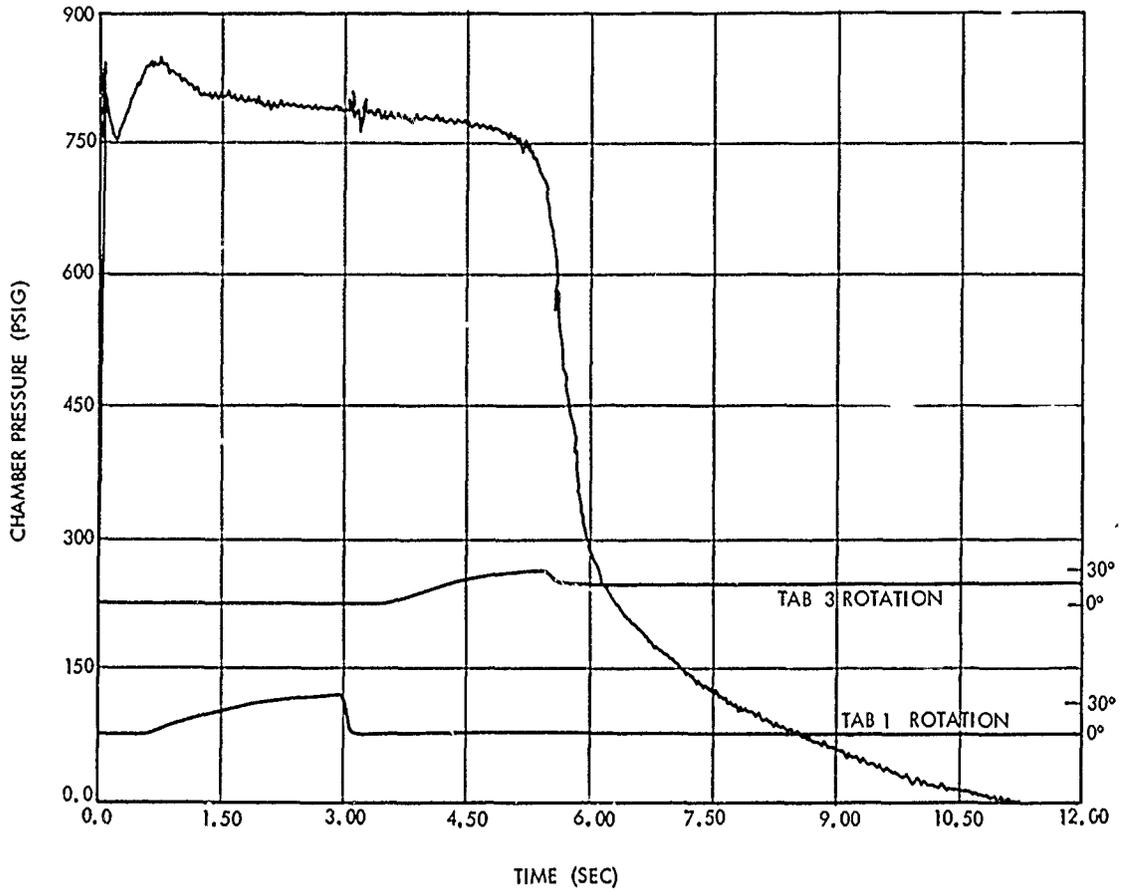
Figure 5-27. Tab Actuation and Motor Chamber Pressure, PFRT-03
