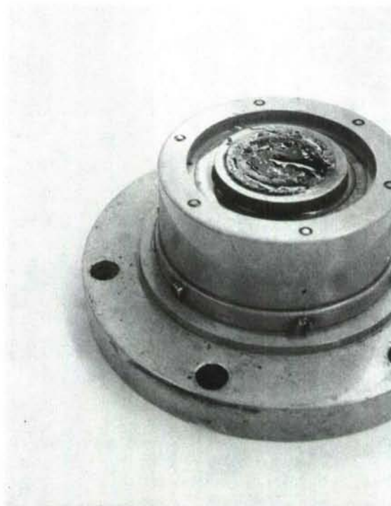
Figure 27 DC FCS 210/LS, 1:2 Copolymer Sealant With Beads After 1 Cycle (177 to -54^{\circ}\text{C} ), Lower Channel, Formulation #16
