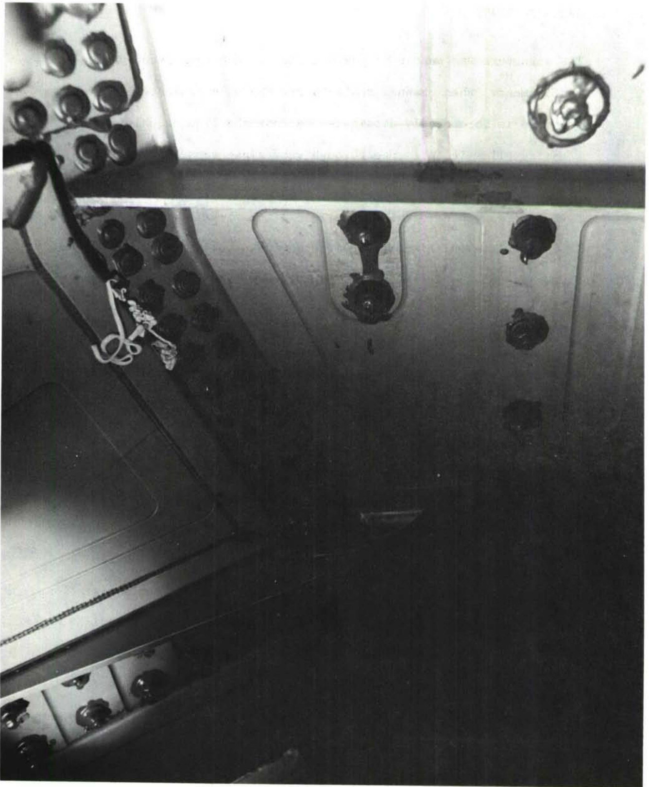
Figure 5 Gap Extrusion in an F-111 Saddle Tank
