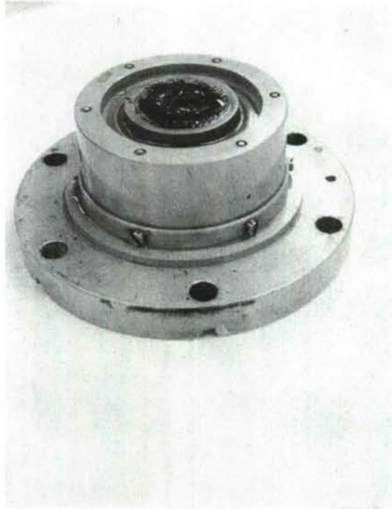
Figure 26 DC FCS 210/LS, 1:2 Copolymer Sealant After One Cycle (177 to -54^{\circ}\text{C} ), Formulation #15
