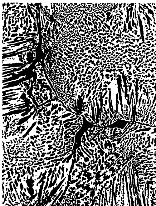
(q) HEAT 24280 (9619) Ti-19Cu-1Al 1560F-1 hr-FC
