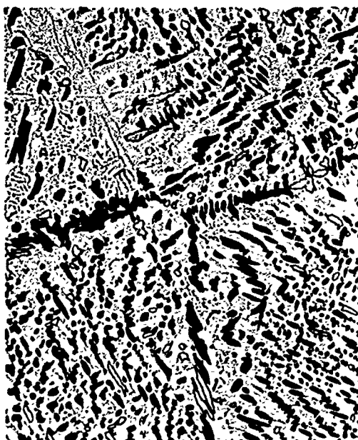
(i) Heat 24221 (9477) Ti-13Cu-1Co 1760F-1hr-FC
