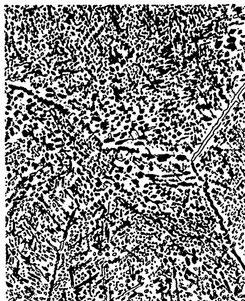
(j) Heat 24221 (9475) Ti-13Cu-1Co 1560F-1hr-FC
