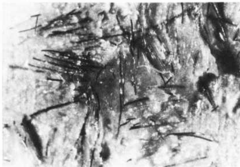
FIGURE 7. Photomicrographs (50 X) of the Failure Surface of ADX-653/PWA Carbon Fabric Single Overlap Shear Bonds.
