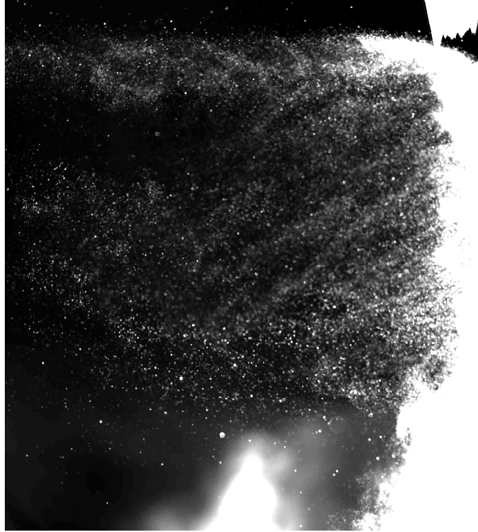
Figure 89. Average quality image of pylon wake on centerline (pylon on right edge of frame)
