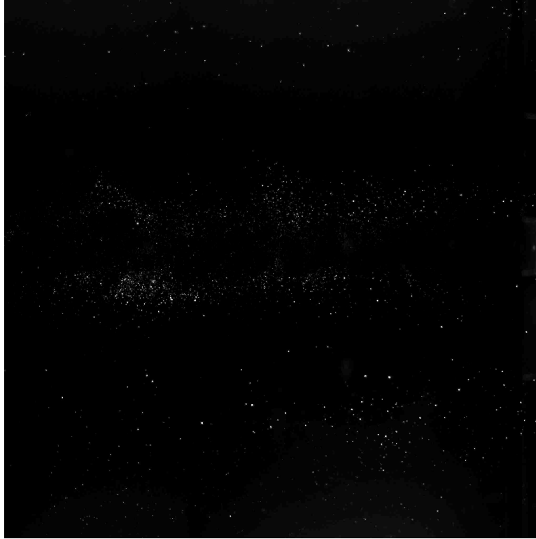
Figure 87. Good quality PIV wake image (pylon on center-right of frame, image plane at y = 3.7 cm)
