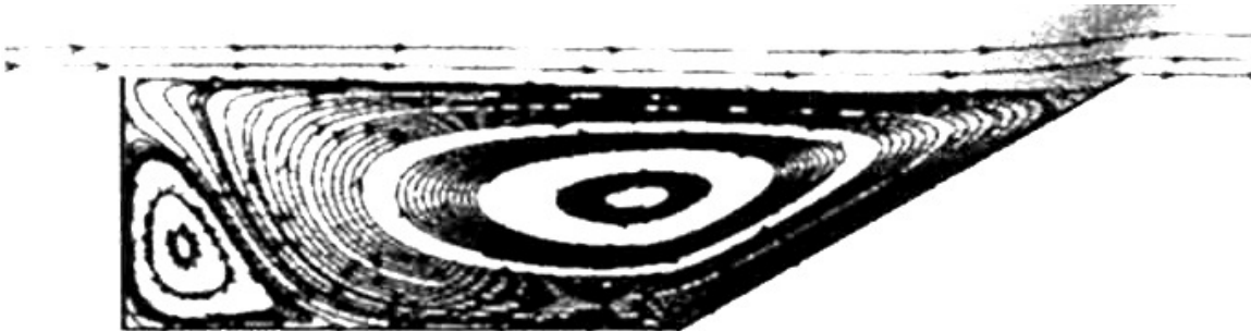
Figure 9. Computational streamlines for M = 3 , Re = 51 \times 10^6 \text{ m}^{-1} flow over an L/D = 3 , 30^\circ inclined cavity flameholder [38]
