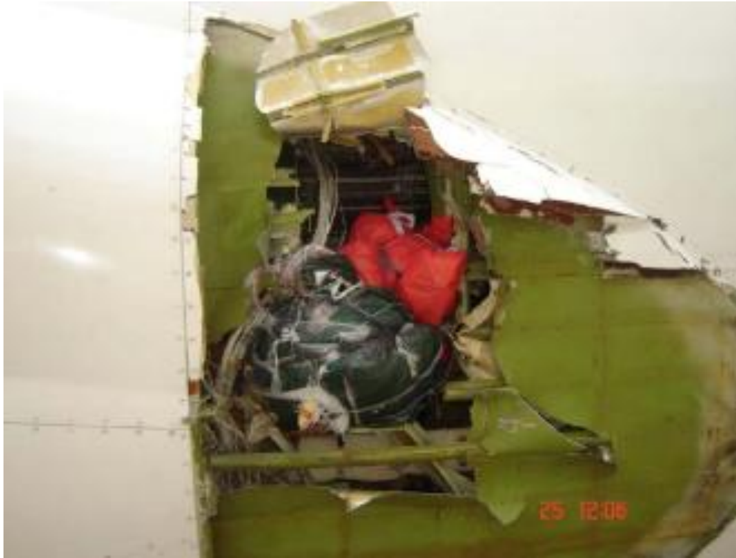
Figure I4: Alternate Close Up View of Boeing 747 Fuselage After On-Board Explosion Illustrating Loss of Structure
