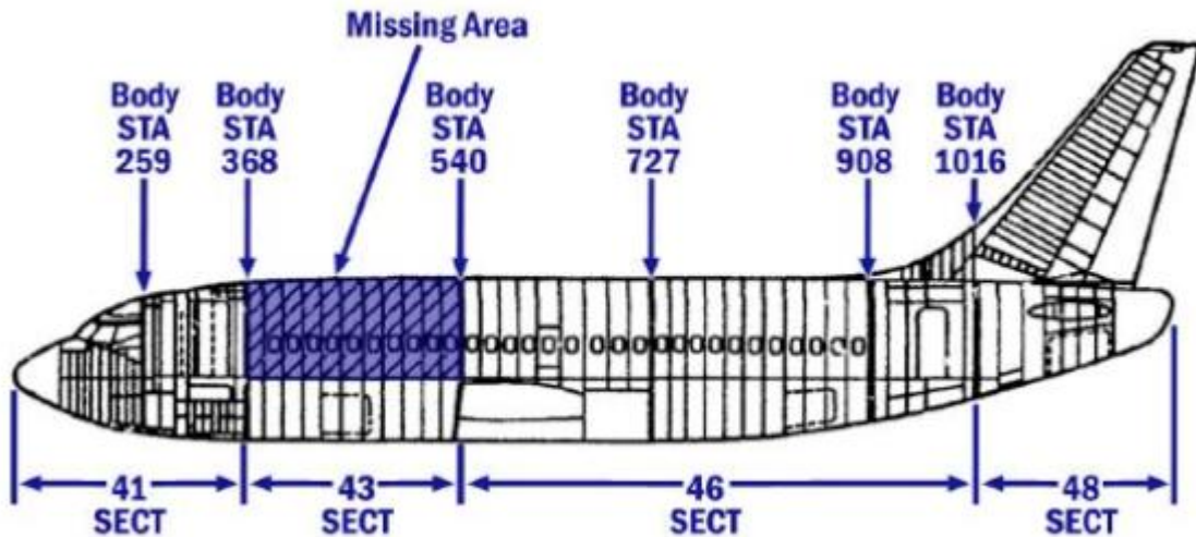
Figure J3: Sketch Illustrating Side View of Fuselage with Missing Area of Boeing 737 Aircraft
