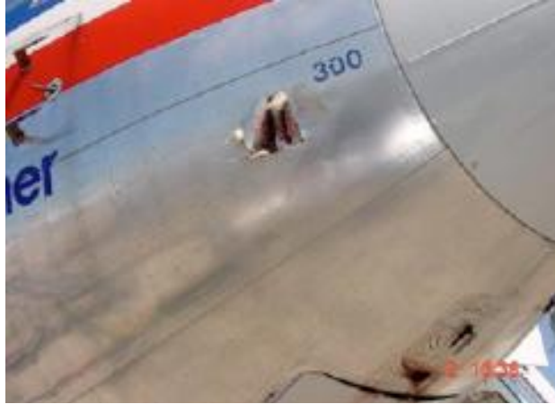
Figure G5. Photo of Bird-Strike Damage to Underside of B767 Fuselage Just Aft of the Radome
