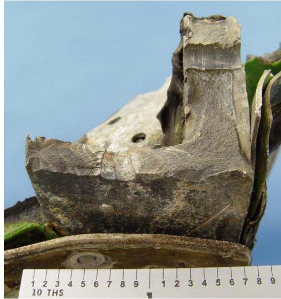
Figure C18: Photo of the Fracture Face of the Right Wing Rear Spar Cap [C13]
