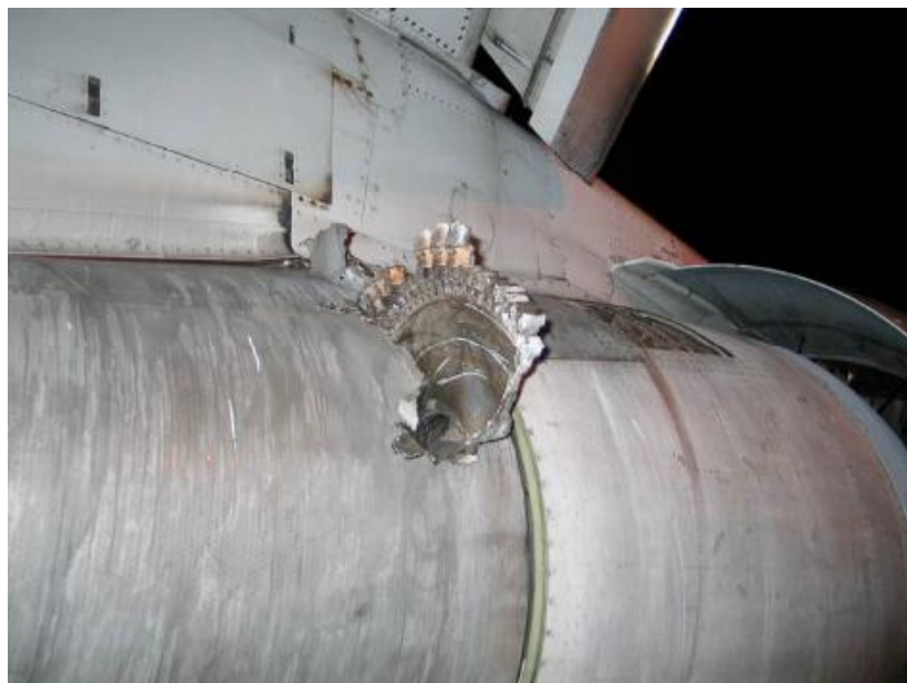
Figure F17: Photo of B747 with Disk Embedded in No. 2 Engine Resulting from Uncontained Rotor Failure in No. 1 Engine
