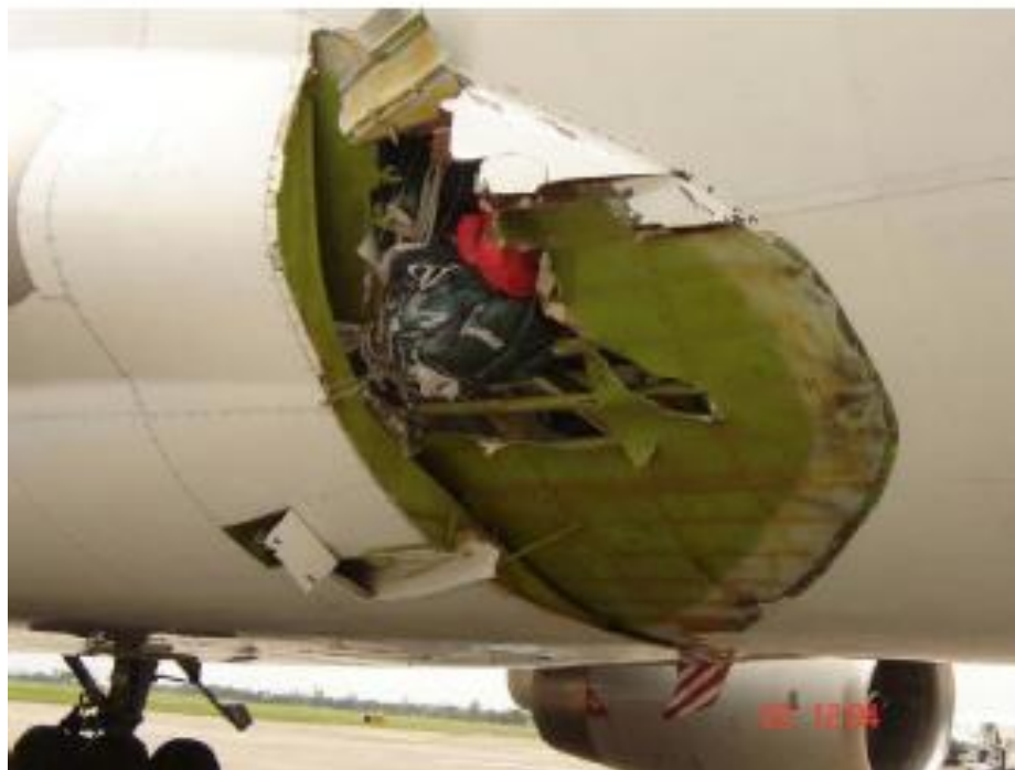
Figure I3: Close Up View of Boeing 747 Fuselage after On-Board Explosion
