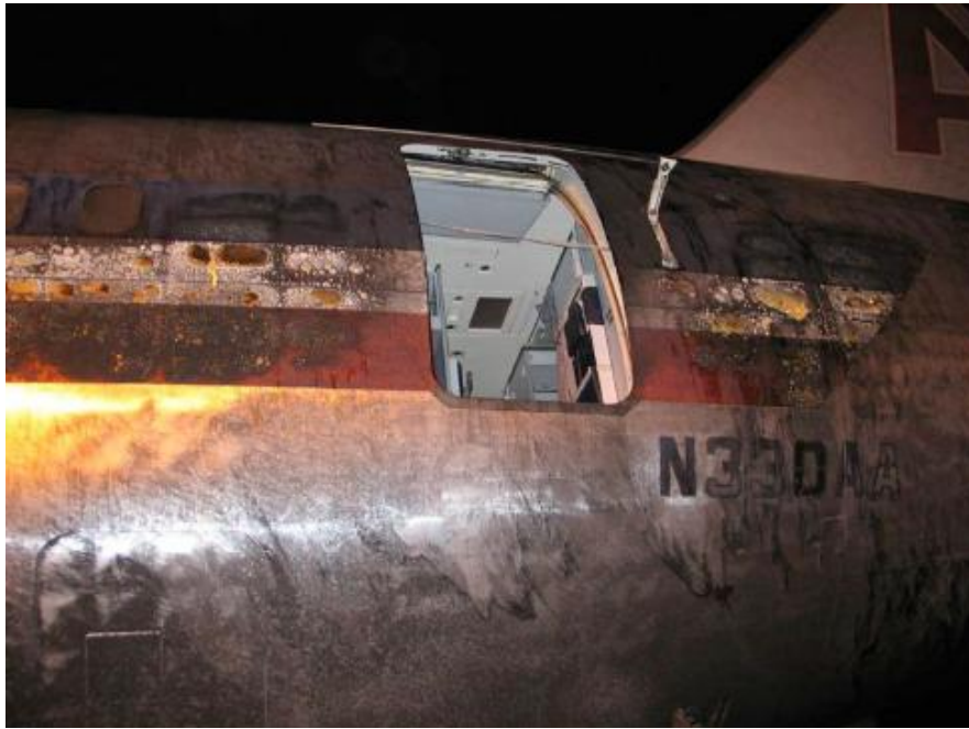
Figure F18: Photo of Engine Damage to the B747 Fuselage Resulting From Engine Failure
