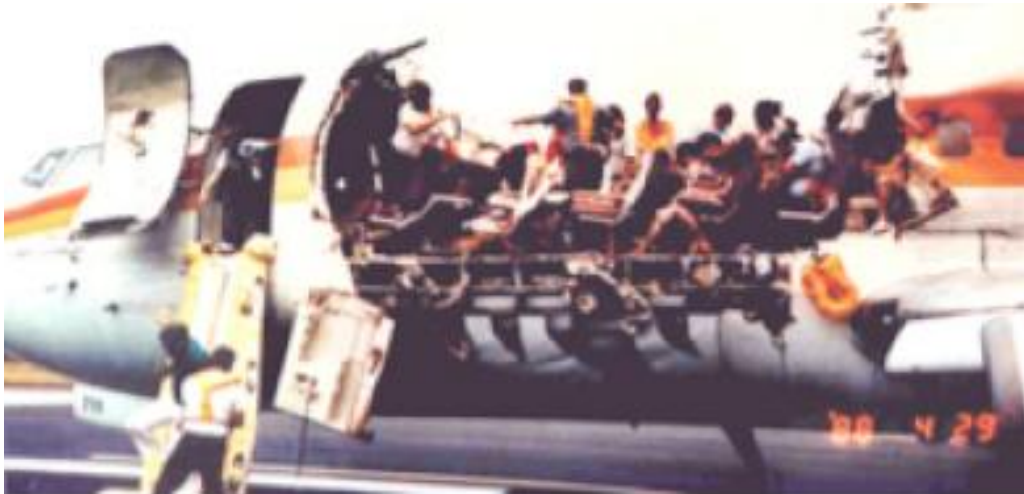
Figure J2. Photo Illustrating Extent of Aircraft Damage to Boeing 737 Aircraft Following Failure Due to Widespread Fatigue Damage
