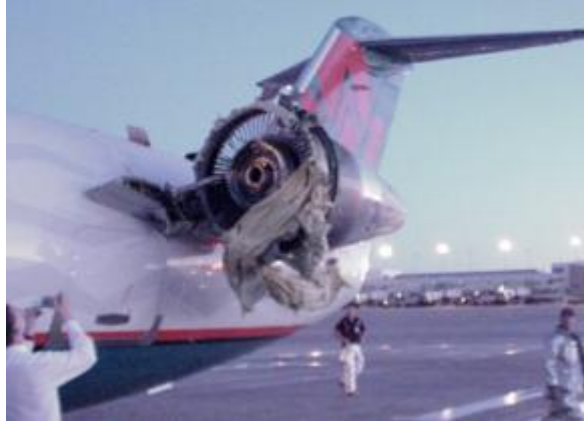
Figure F14: Photo of Damage Associated With Engine Failure
