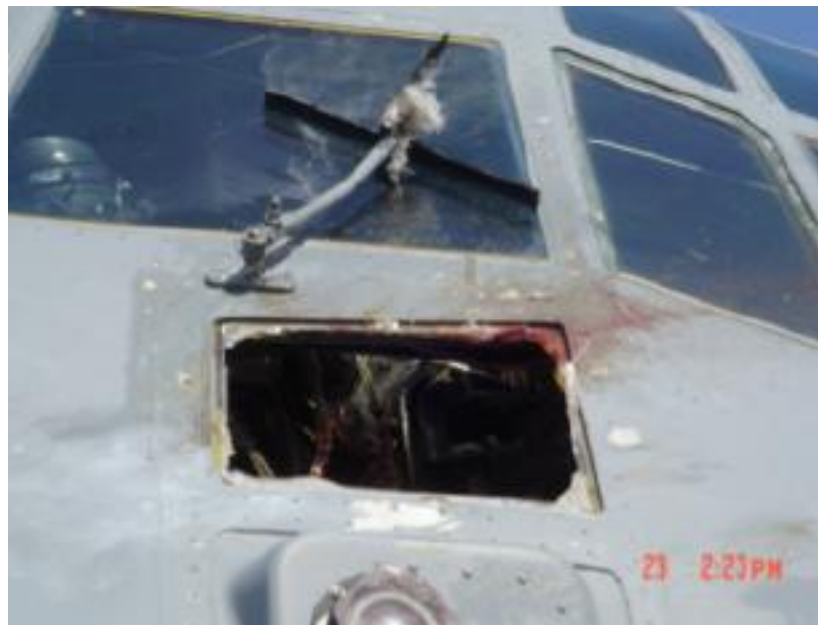
Figure G7.: Photo of Bird Strike Damage to Outside of the C-130 Aircraft
