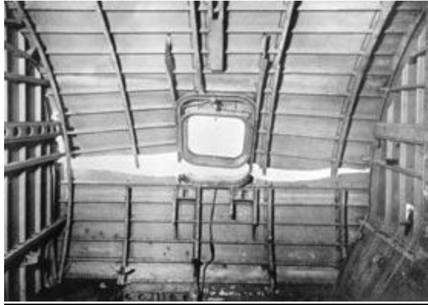
Figure A.5: Uncontained Running Cracks Caused the Breakup of this Hydro Test of the Retired Comet 1 (G-ALYU). Cracks Propagating from Forward Escape Hatch on the Port Side. Note that No Straps or Shear Tied Frames were Used. No Crack Arrestment Capability was Provided by this Construction. [A2]
