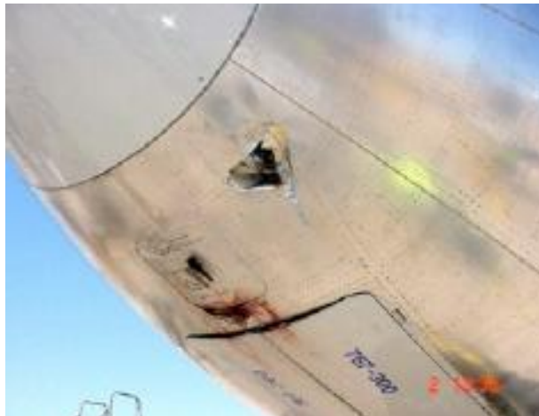
Figure G4: Photo of Bird Strike Damage to Underside of Fuselage of B767 Aircraft
