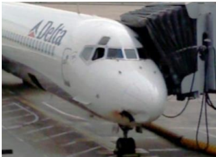
Figure G2: Photo of Bird Strike Damage to Radome
