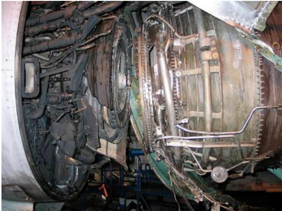
Figure F15: Photo of Damage Associated with Uncontained Rotor Failure in a GE CF6 Engine
