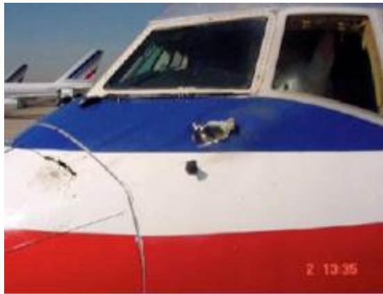
Figure G3: Photo of Bird Strike Damage to B767 Aircraft Just Below the Cockpit Windows
