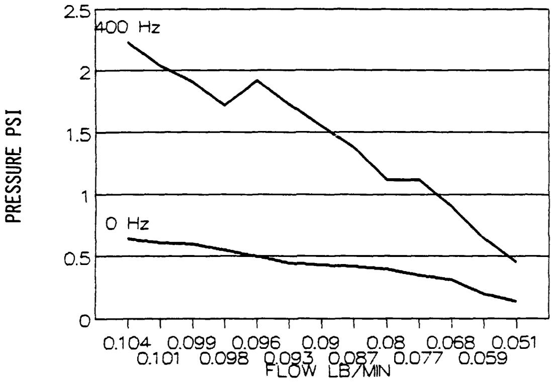
Figure 5-7, Pressure Into Chopper VS Flow
