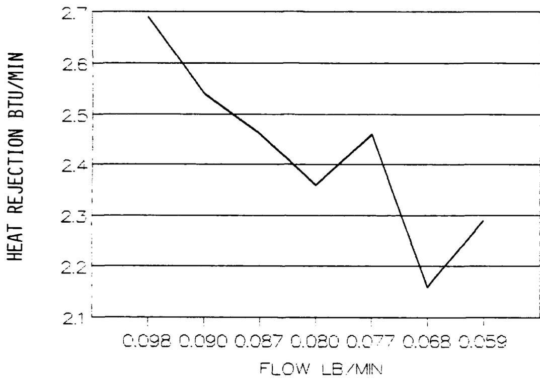
Figure 5-10, Heat Rejection VS Flow
