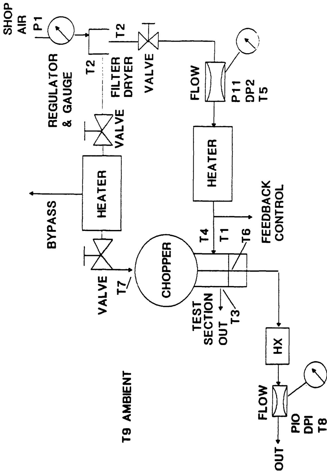
Figure 4-1, Experimental Apparatus
