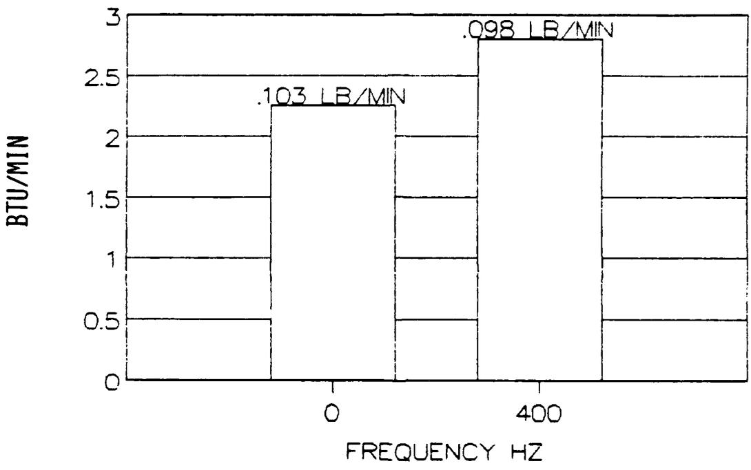
Figure 5-8, Change in Heat Rejection
