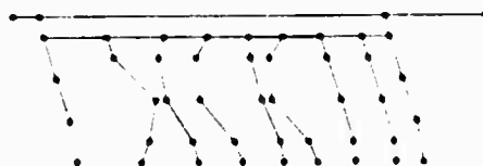
FIGURE 4b MODE SHAPE NO. 2 FREQUENCY 8.640 Hz
