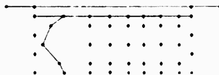
FIGURE 4a MODE SHAPE NO. 1 FREQUENCY 3.610 Hz
