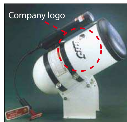
Typical BRS Canister system commonly used in ultralight and sport aircraft illustrating the manufacturers logo
