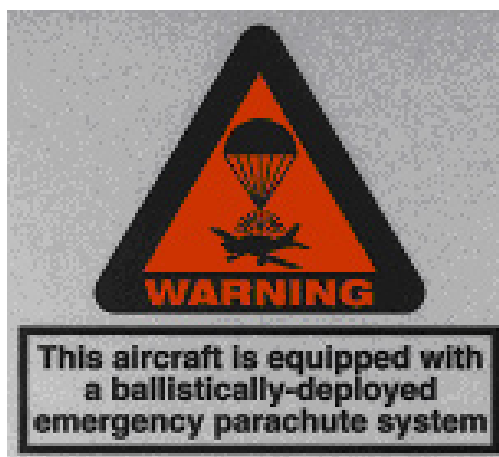
Ballistic recovery system warning sign
