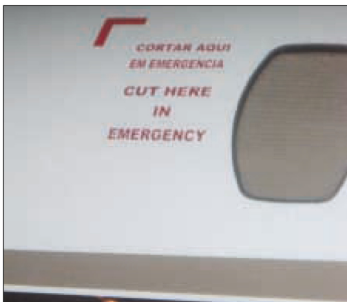
Emergency cutting area on aircraft fuselage
