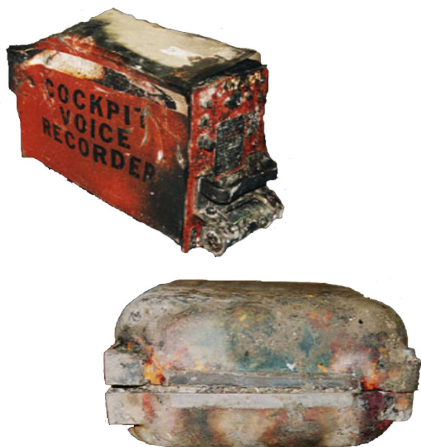
An example of a partially damaged CVR and the discoloured crash-protected tape module from a damaged FDR
