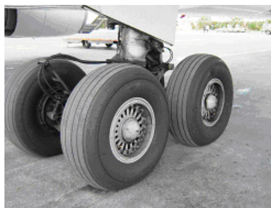
Commercial aircraft tyres can be pressurised to 250 psi, and can deflate explosively if damaged by fire and/or impact
