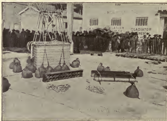
FIG. 132.—Basket of Count de la Vaulx' balloon, showing the deviators.
