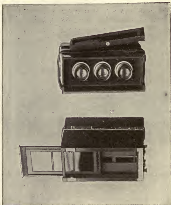
FIG. 213.—Miethe's camera for three-colour photography in a balloon.
