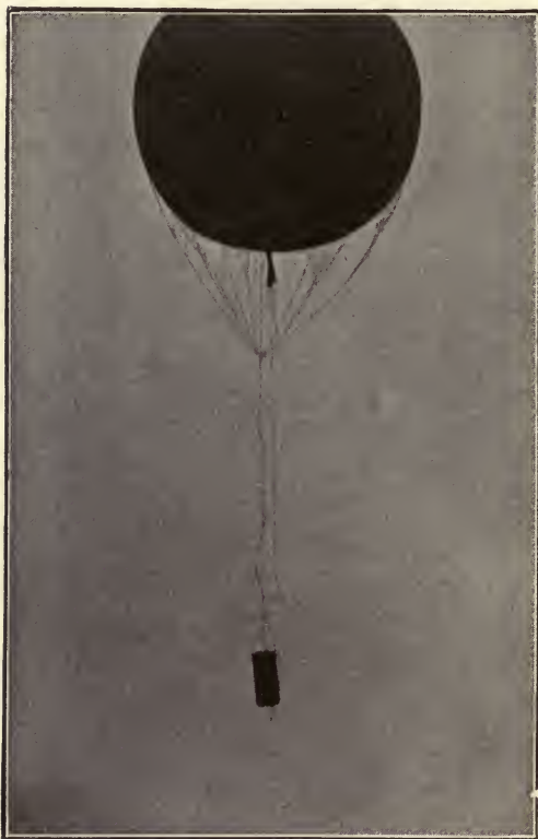
FIG. 157.—A recording balloon with instruments.
