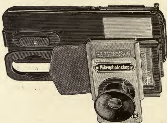
FIG. 121.—Vollbehr's microphotoscope for reading maps on a reduced scale, together with illuminating device for night work.
