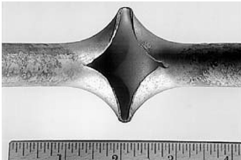
FIGURE 7. Tubing split caused by pitting. 26
