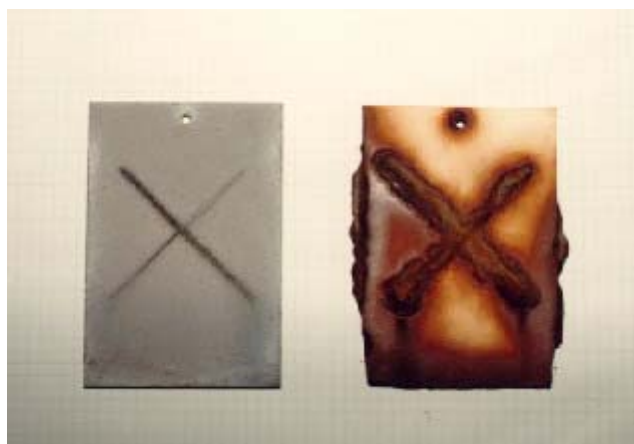
FIGURE 5. Untopcoated inorganic ZRP (left steel panel) and epoxy and urethane topcoated inorganic ZRP (right steel panel) after 8 years of atmospheric exposure at the BCTS. 5
