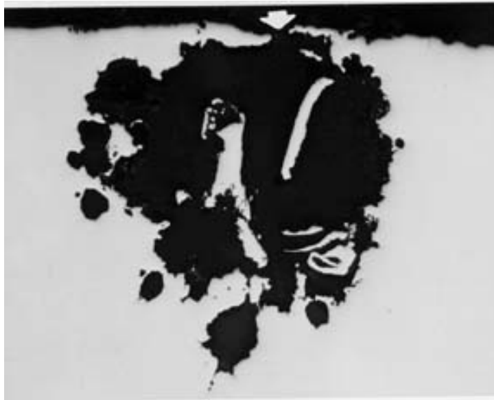
FIGURE 6. Micrograph (100x magnification) of pit from KSC's launch pad tubing. 26
