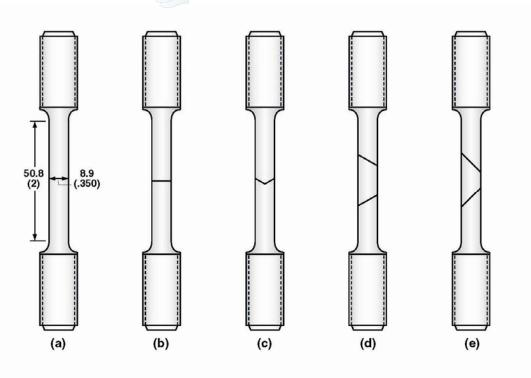
(a) - base metal blanks; (b) – butt joints; (c) – V60; (d) – D60 and (e)  $-45^{\circ}$  (e)
