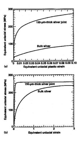
Fig.2.8 Equivalent uniaxial stress vs. equivalent uniaxial strain plot for silver-brazed maraging steel butt brazed specimens tested in torsion. An expanded view of the initial region of the test, up to 0.1 strain is shown in (a). The entire test is captured in (b). Note a significant difference in strain hardening rate between the bulk silver and a silver layer in the brazed joint. Reprinted with permission from Rosen R. S., et al (1980). Copyright 1980, American Vacuum Society.
