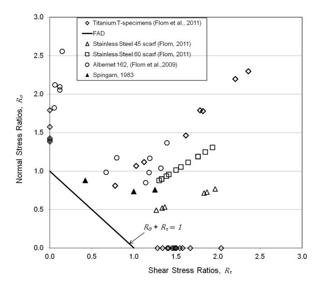
Fig.2. 10 Test results from previous studies plotted as stress ratios. As one can see the FAD line defined by  $R_{\sigma}+R_{\tau}=1$  can be used quite conservatively for the lower bound estimate of stress combinations that may cause brazed joint failure. Titanium lap shear and butt brazed specimens (Flom et al., 2011) are also plotted along shear and normal stress axes, respectively.
