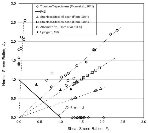
Fig.2. 11 The same results as in Fig.10 shown here with the addition of the trend or brazed joint lines (dashed). Each trend line is associated with a specific braze joint geometry. We can also call them braze joint lines. A position of the data point on such line indicates a particular stresses combination.
