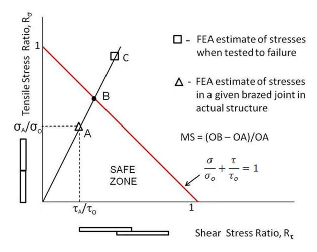
Fig.2. 13 This graph illustrates the process of constructing the braze joint line and determining margins of safety of the brazed joint. Safe zone represents safe combinations of stresses.
